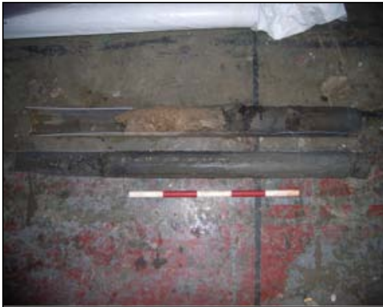
Plate 2 Borehole cores 0-2m from BH4. Note thin layer of 'organic material' between 1.77m-1.85m
