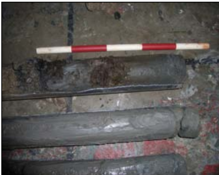
Plate 3 Close-up of layer of 'organic material' from BH4
