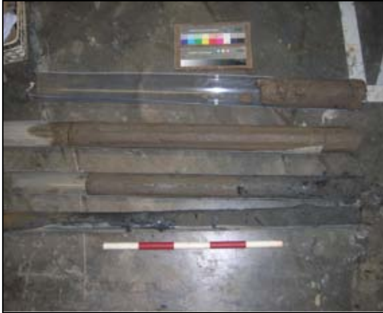
Plate 4 Borehole cores 0-4m, from BH3. Note very thin deposit of 'organic material' between 2.68m-2.7m
