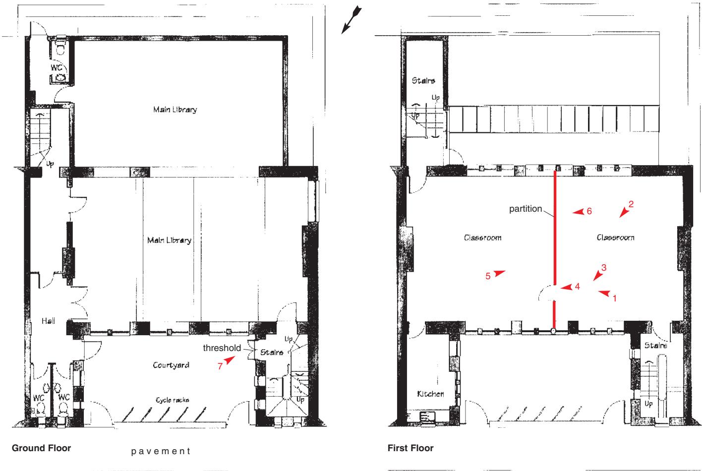
Fig.2 General plan of the library indicating the location of the proposed alterations and plate directions in red
