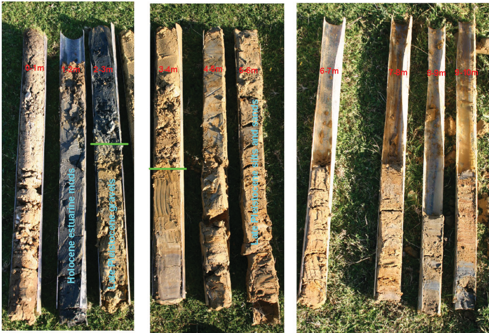
Figure 9. Holocene and Pleistocene sediments from borehole 5 at Allhalllows.
