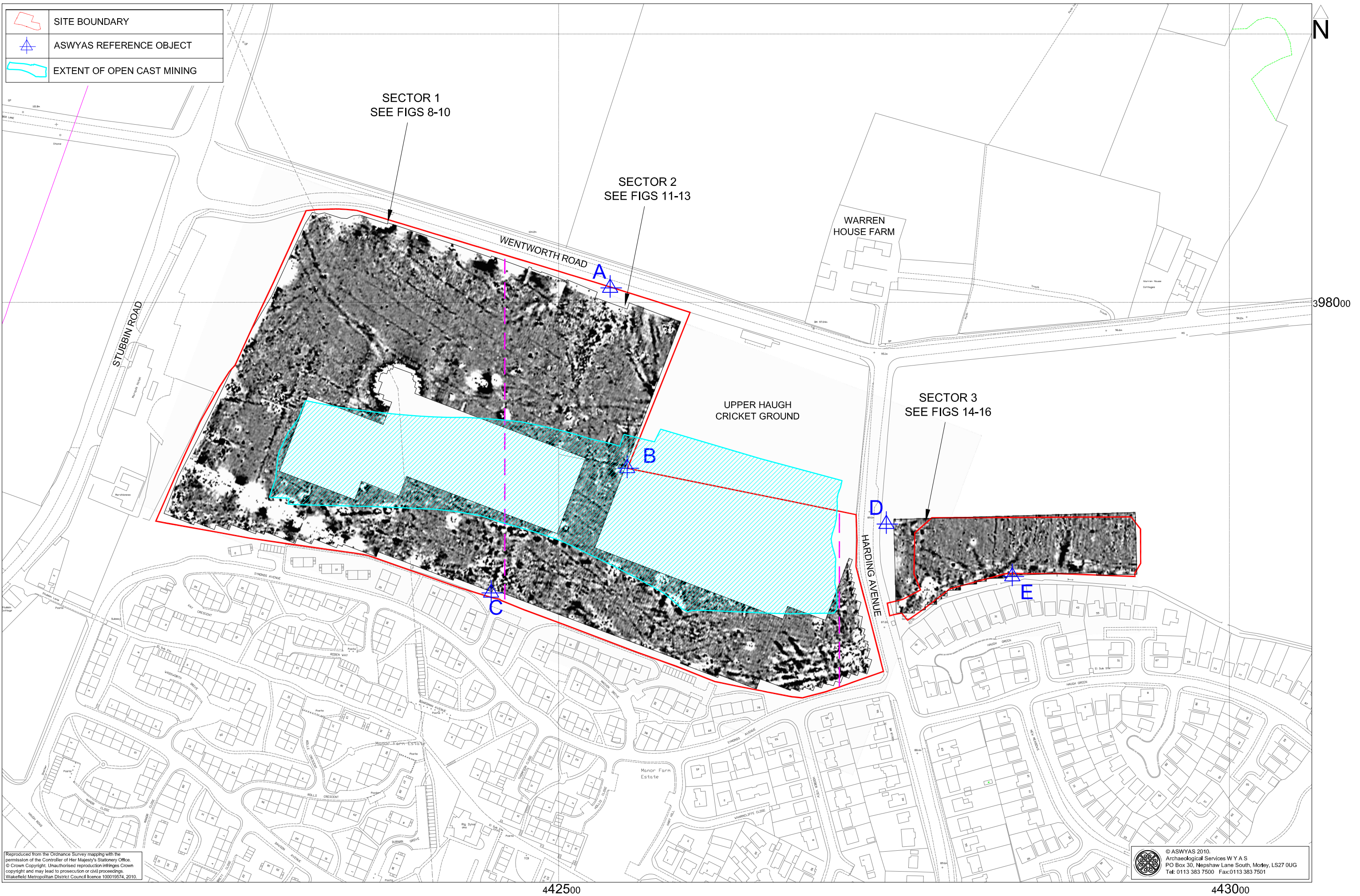
Fig. 2. Site location showing magnetometer data and extent of open cast mining (1:2500 @ A3)
