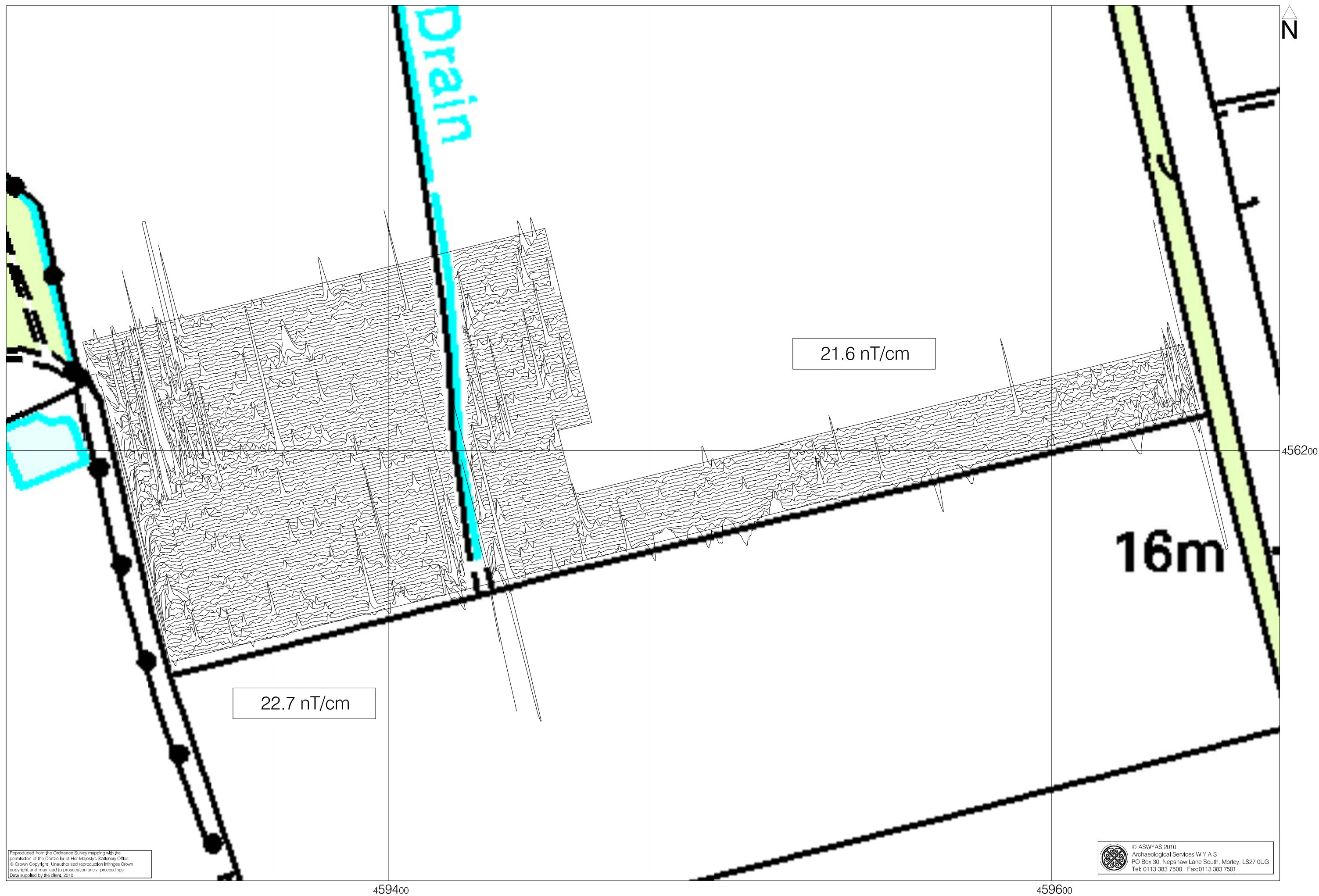
Fig. 4. XY trace plot of unprocessed magnetometer data (1:1000 @ A3)
