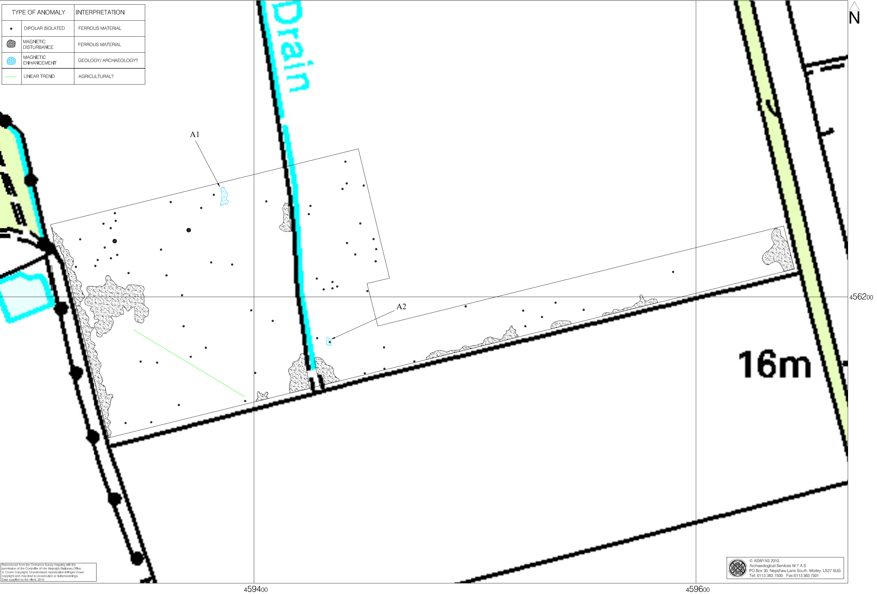
Fig. 5. Interpretation of magnetometer data (1:1000 @ A3)
