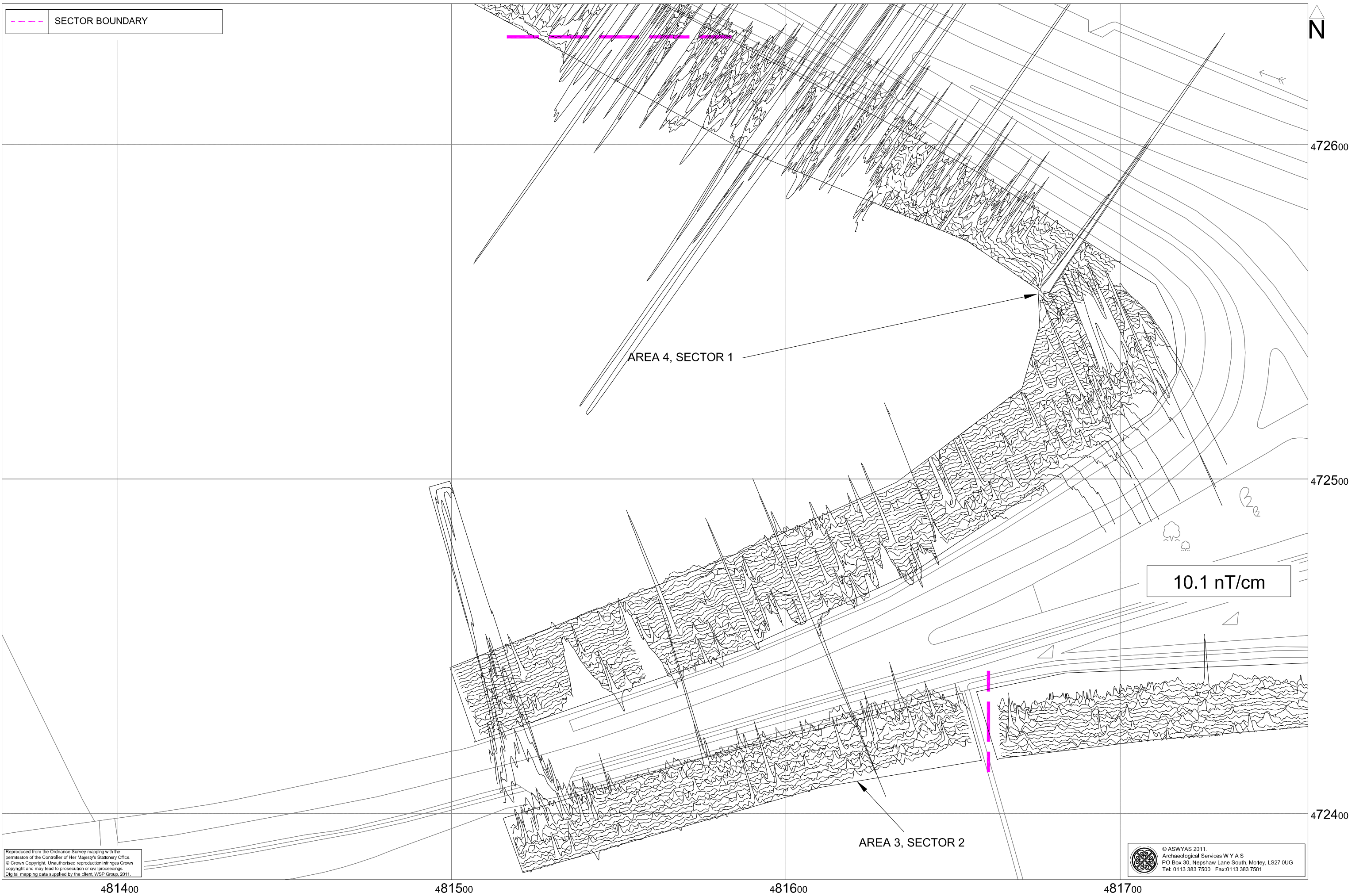
Fig. 11. XY trace plot of unprocessed magnetometer data; Area 3, Sector 2 and Area 4, Sector 1 (1:1000 @ A3)
