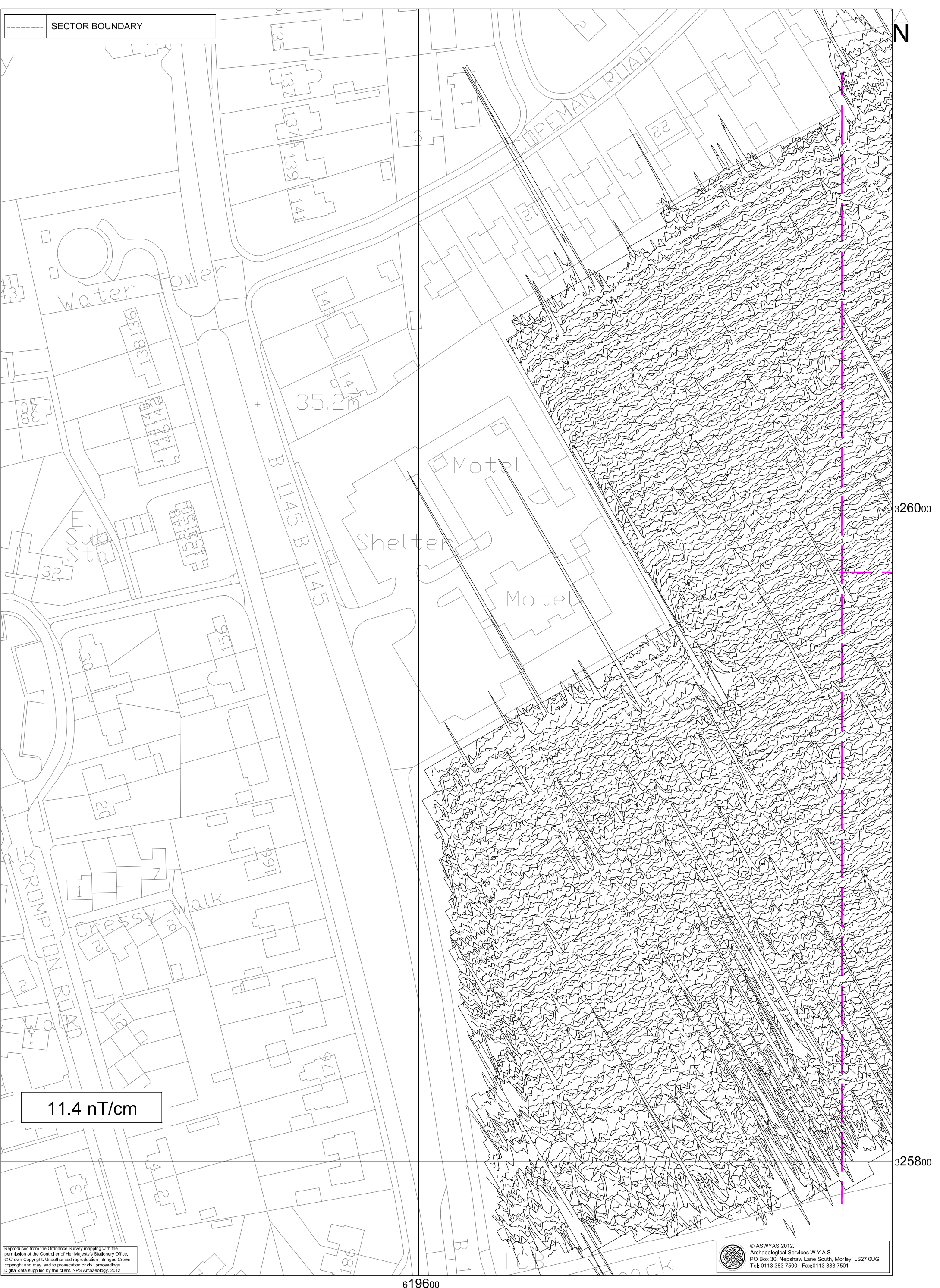
XY trace plot of raw magnetometer data; Sector 1 (1:1000 @ A3)
