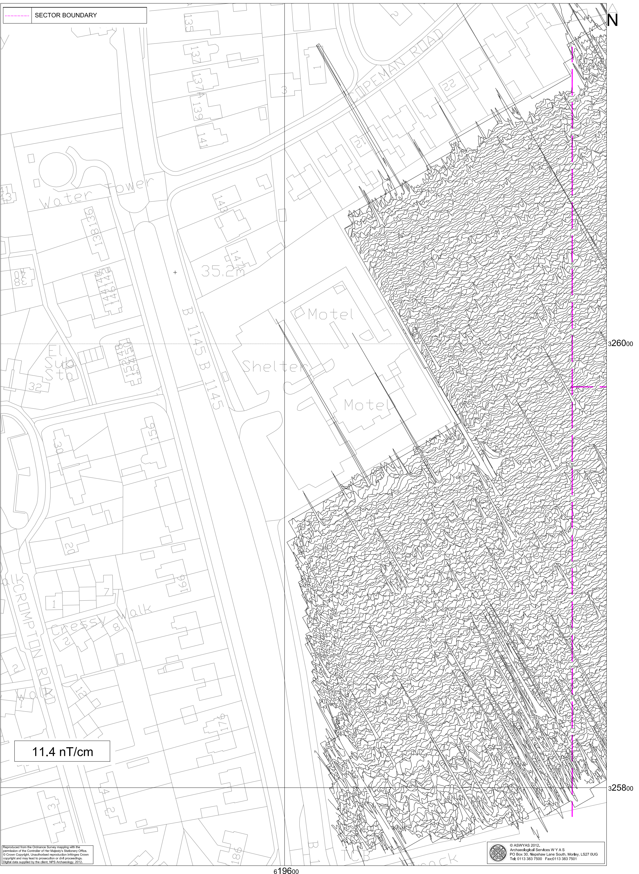
Fig. 5. XY trace plot of minimally processed magnetometer data; Sector 1 (1:1000 @ A3)
