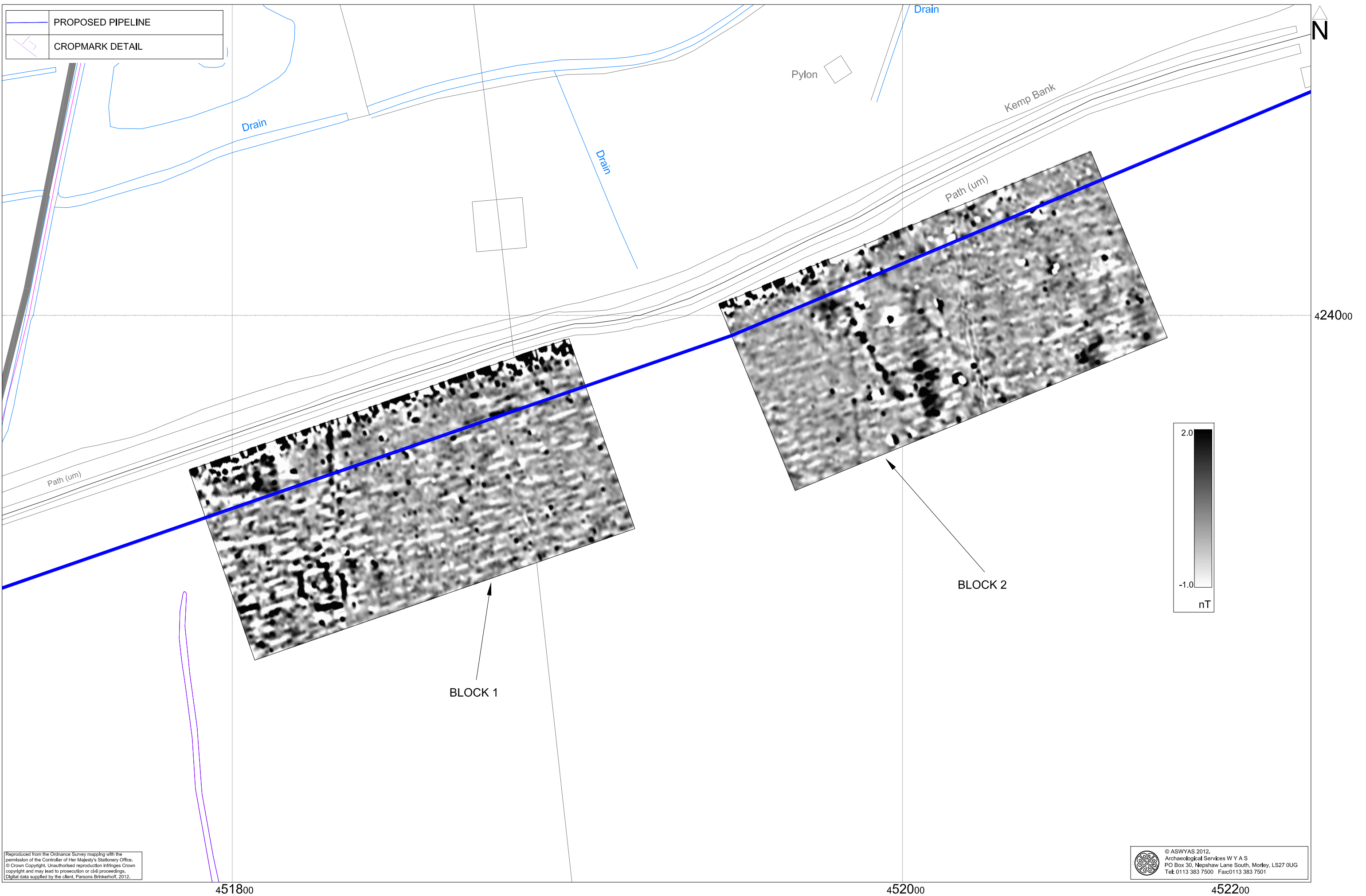
Fig. 3. Processed greyscale magnetometer data; Block 1 and Block 2 (1:1000 @ A3)
