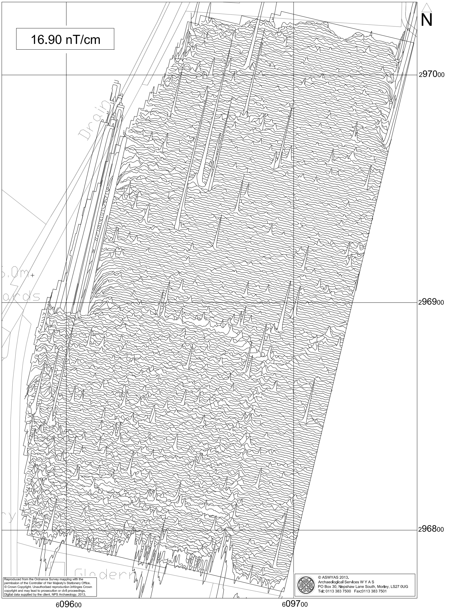
Fig. 7. XY trace plot of minimally processed magnetometer data; Area 2 (1:1000 @ A4)
