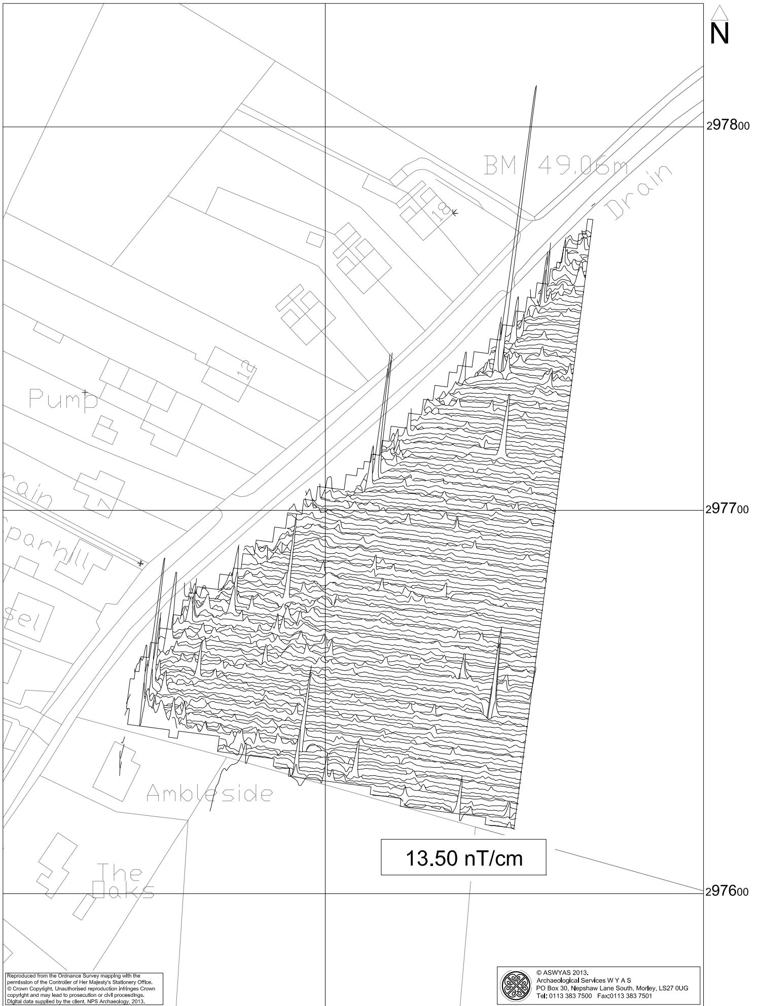
XY trace plot of raw magnetometer data; Area 1 (1:1000 @ A4)
