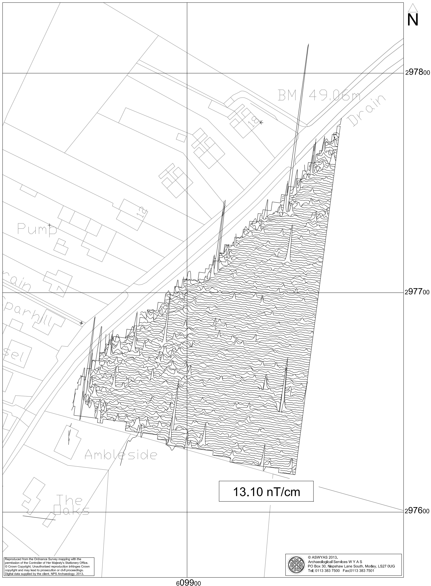
Fig. 4. XY trace plot of minimally processed magnetometer data; Area 1 (1:1000 @ A4)
