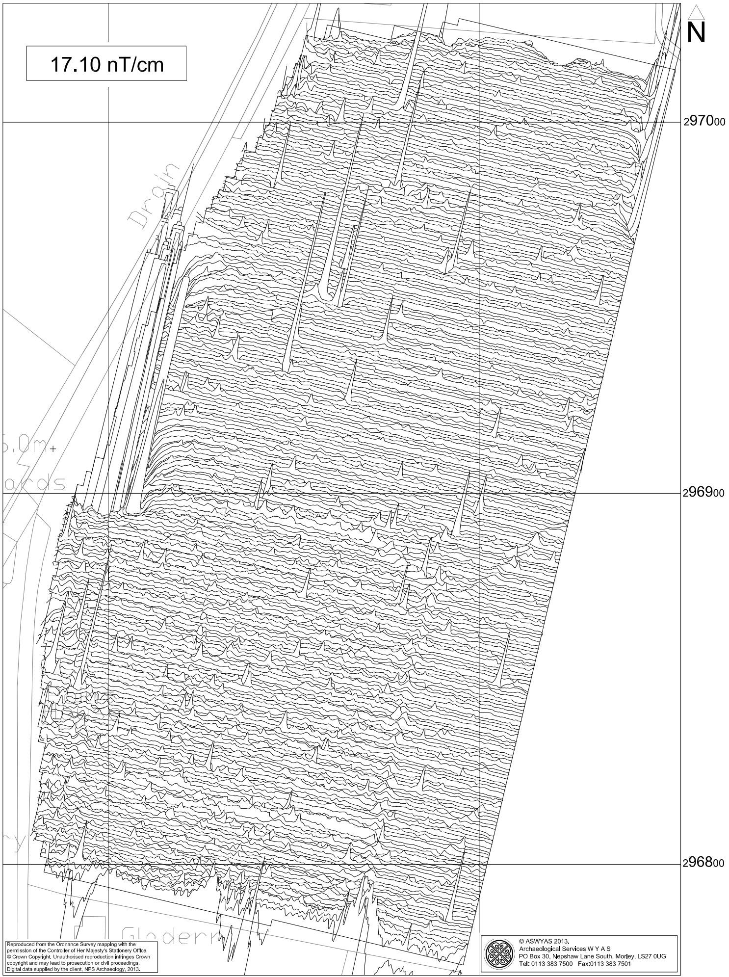
XY trace plot of raw magnetometer data; Area 2 (1:1000 @ A4)
