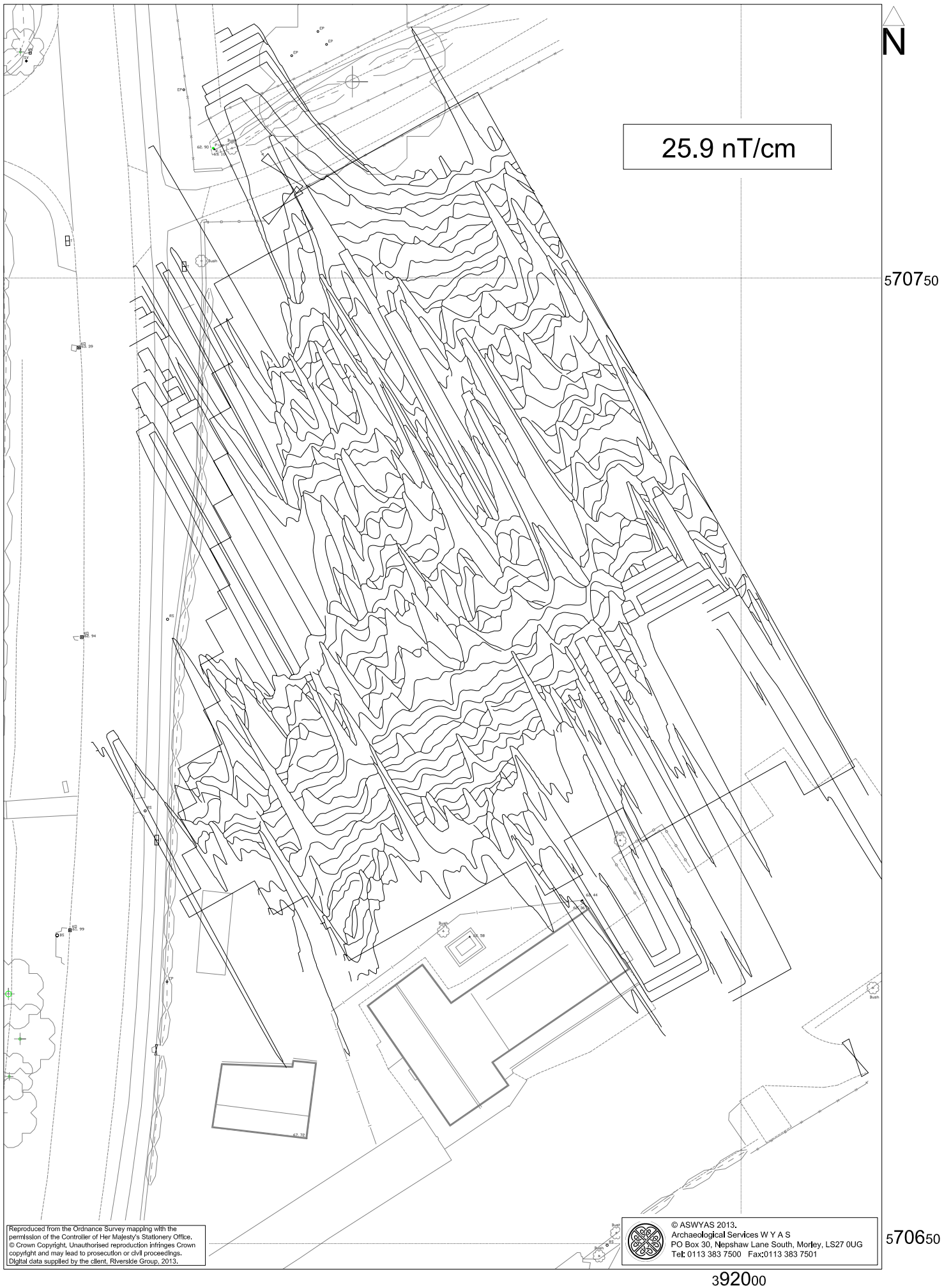
Fig. 4. XY trace plot of minimally processed magnetometer data (1:500 @ A4)
