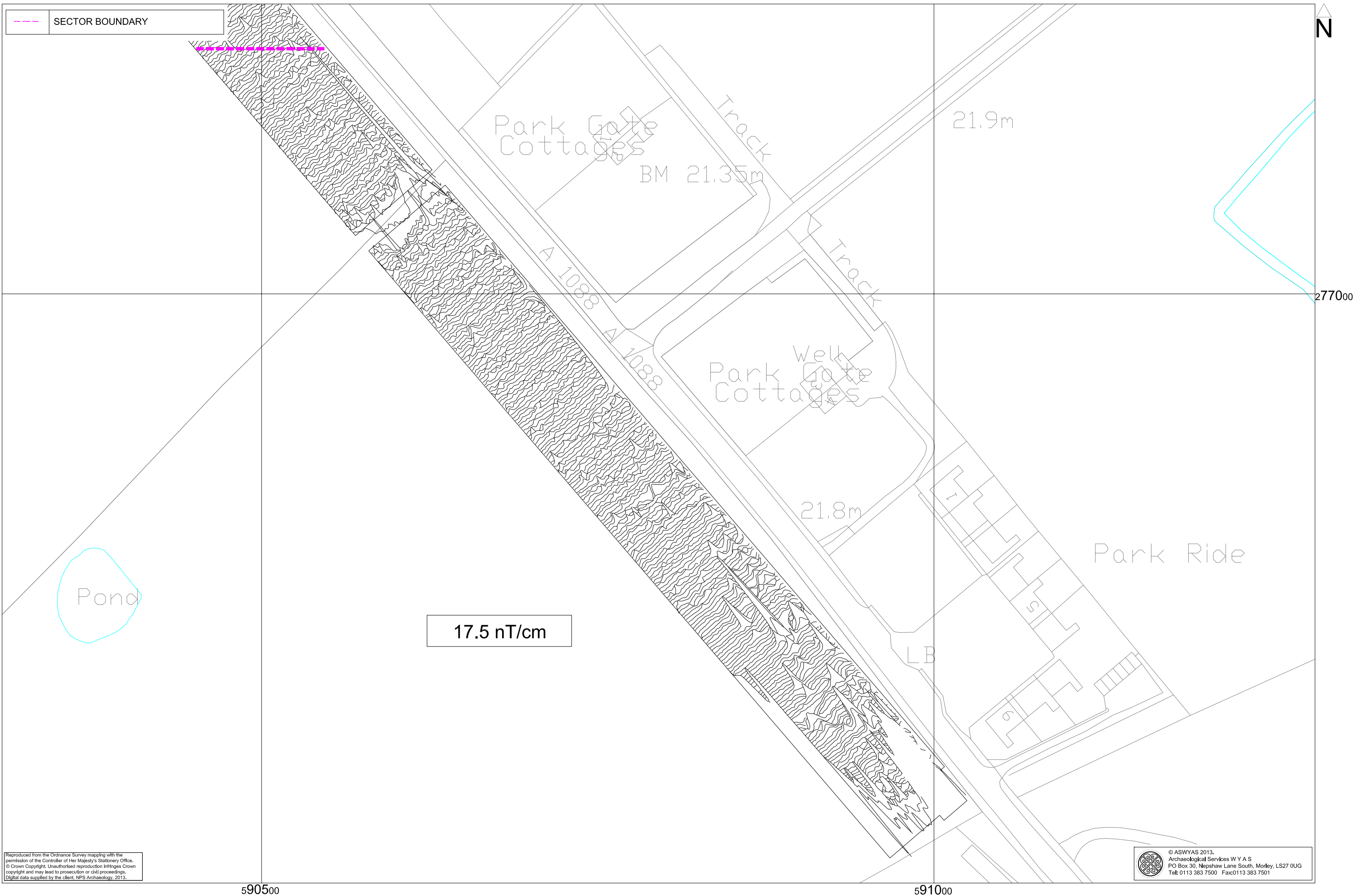
Fig. 19. XY trace plot of minimally processed magnetometer data; Area 1, Sector 4 (1:1000 @ A3)
