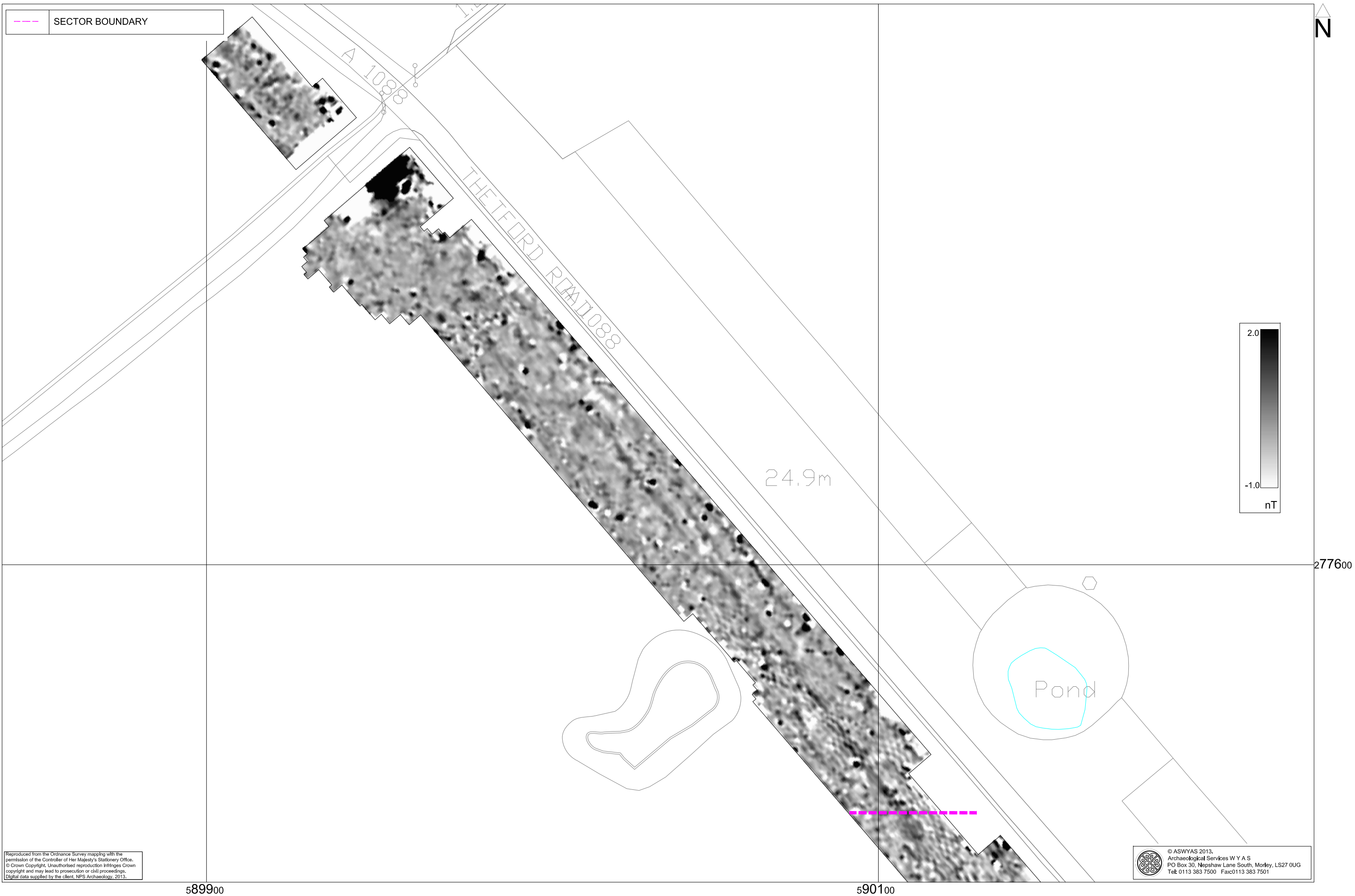
Fig. 9. Processed greyscale magnetometer data; Area 1, Sector 1 (1:1000 @ A3)
