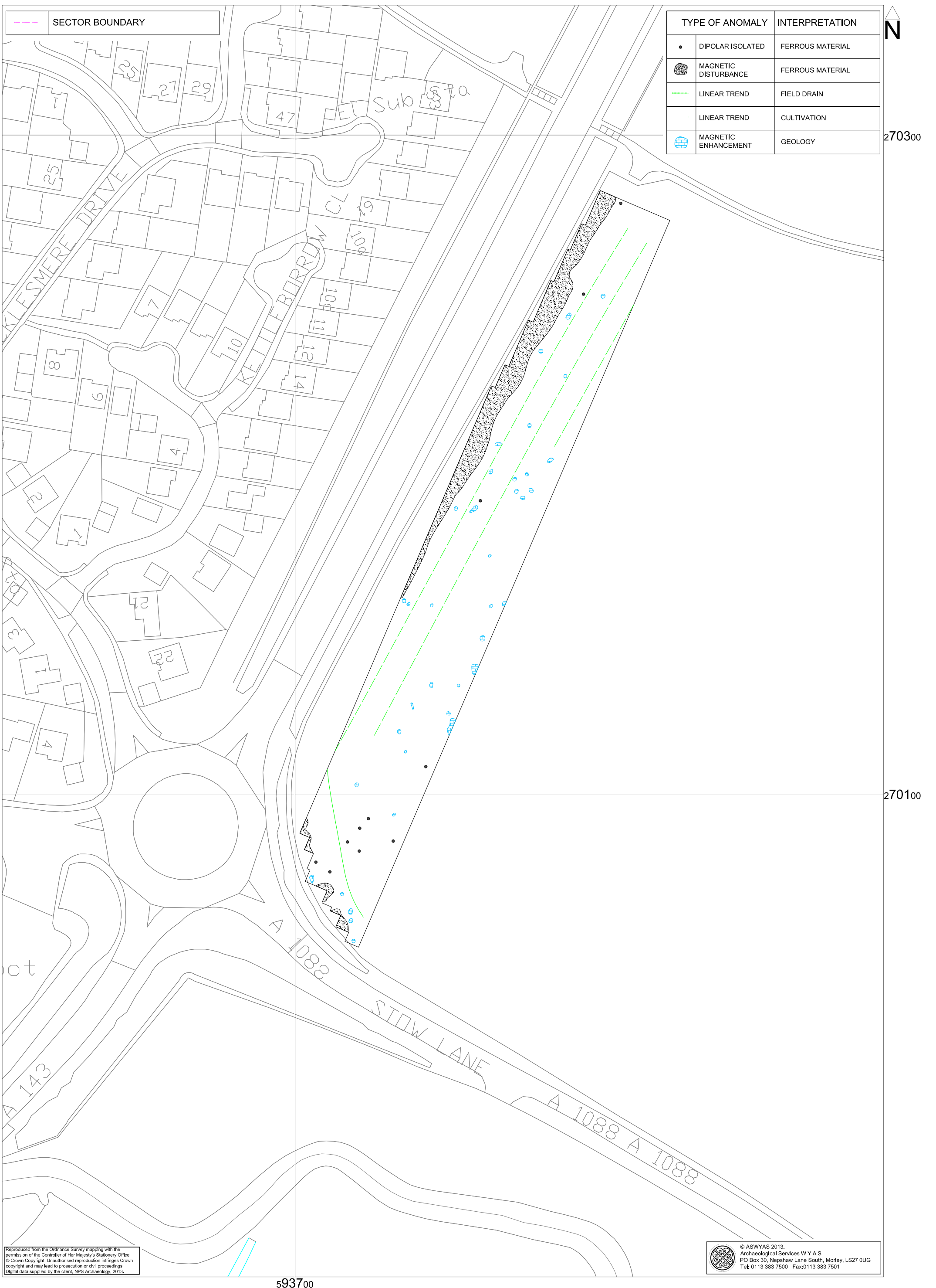
Fig. 23. Interpretation of magnetometer data; Area 2, Sector 1 (1:1000 @ A3)
