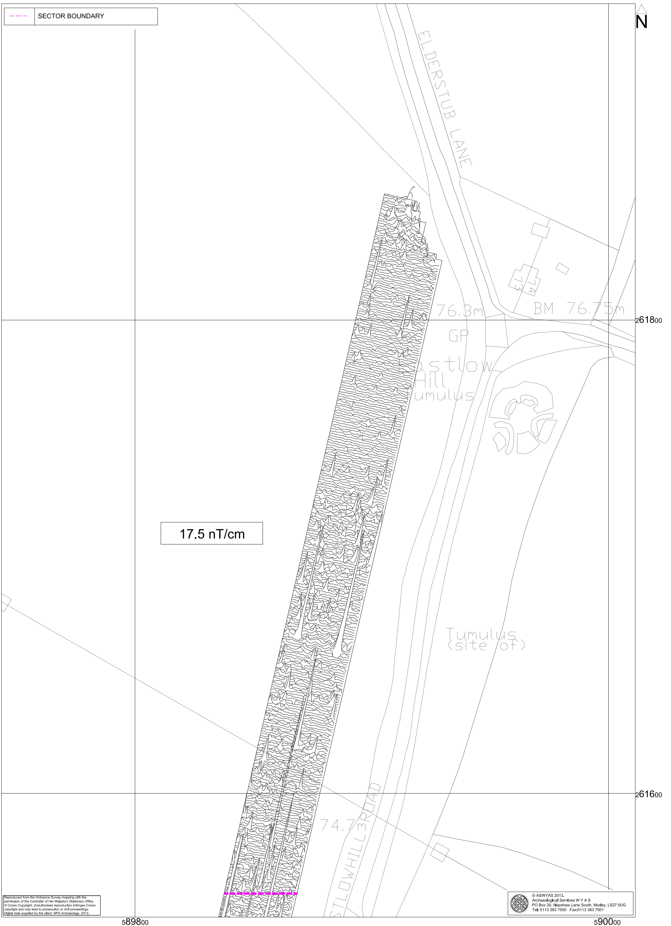
Fig. 31. XY trace plot of minimally processed magnetometer data; Area 4, Sector 1 (1:1000 @ A3)
