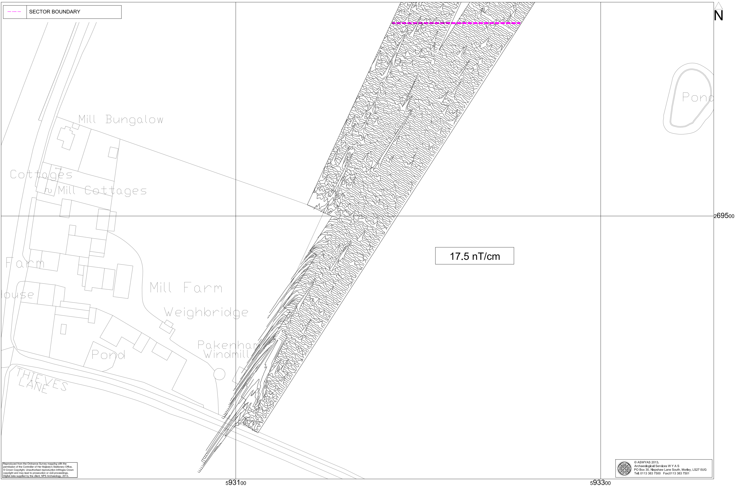
Fig. 28. XY trace plot of minimally processed magnetometer data; Area 3, Sector 2 (1:1000 @ A3)
