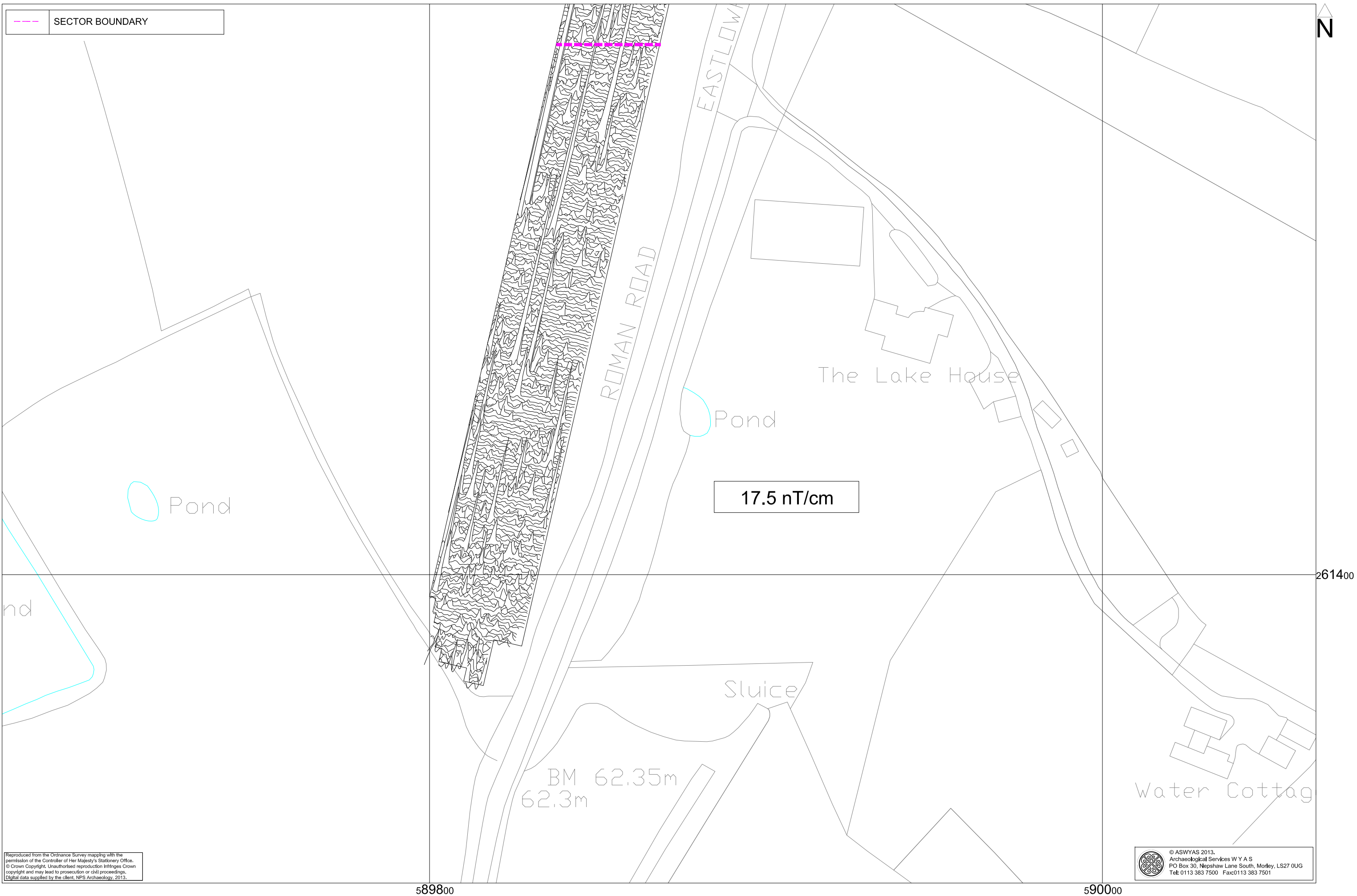
Fig. 34. XY trace plot of minimally processed magnetometer data; Area 4, Sector 2 (1:1000 @ A3)
