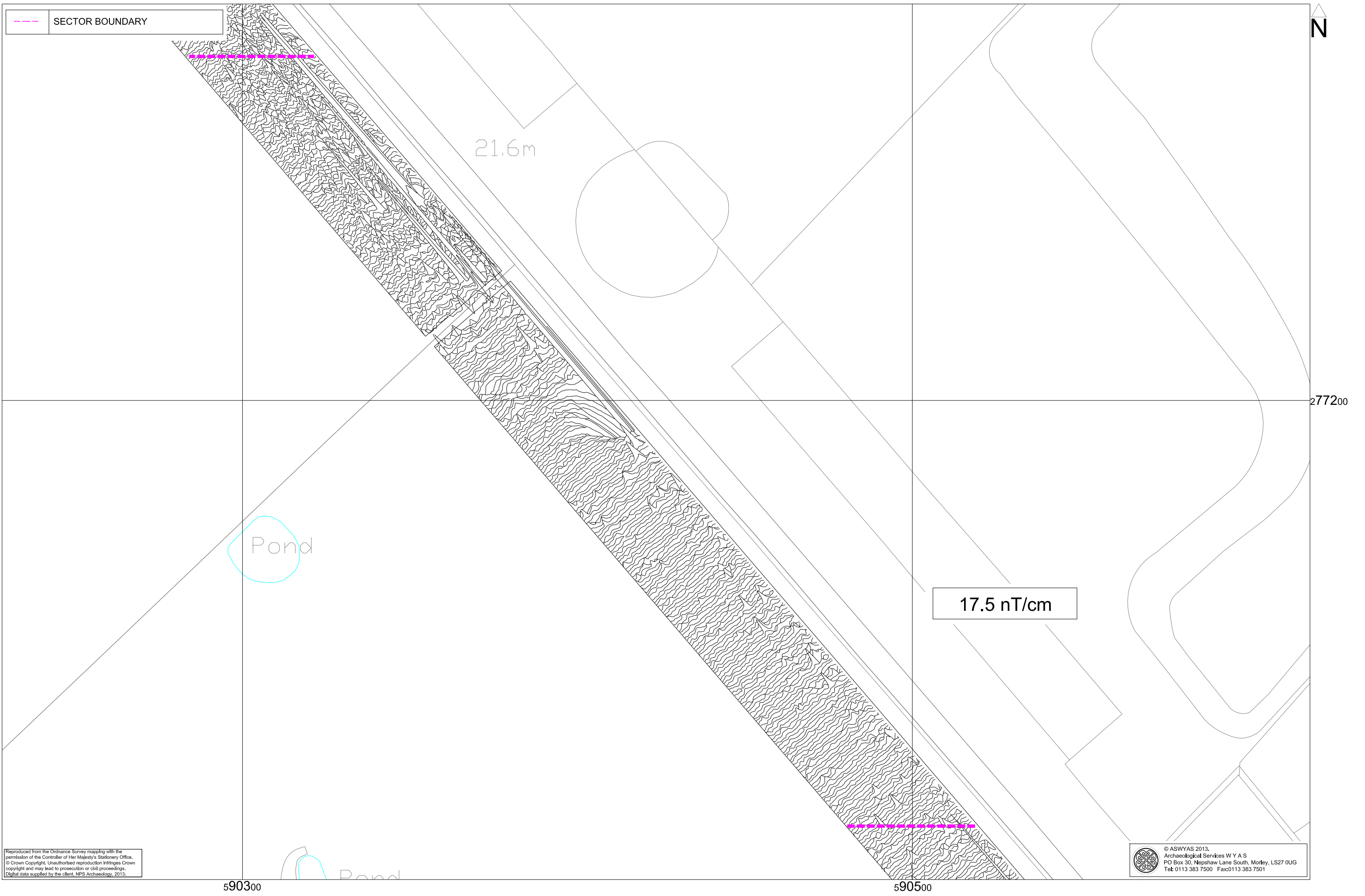
Fig. 16. XY trace plot of minimally processed magnetometer data; Area 1, Sector 3 (1:1000 @ A3)
