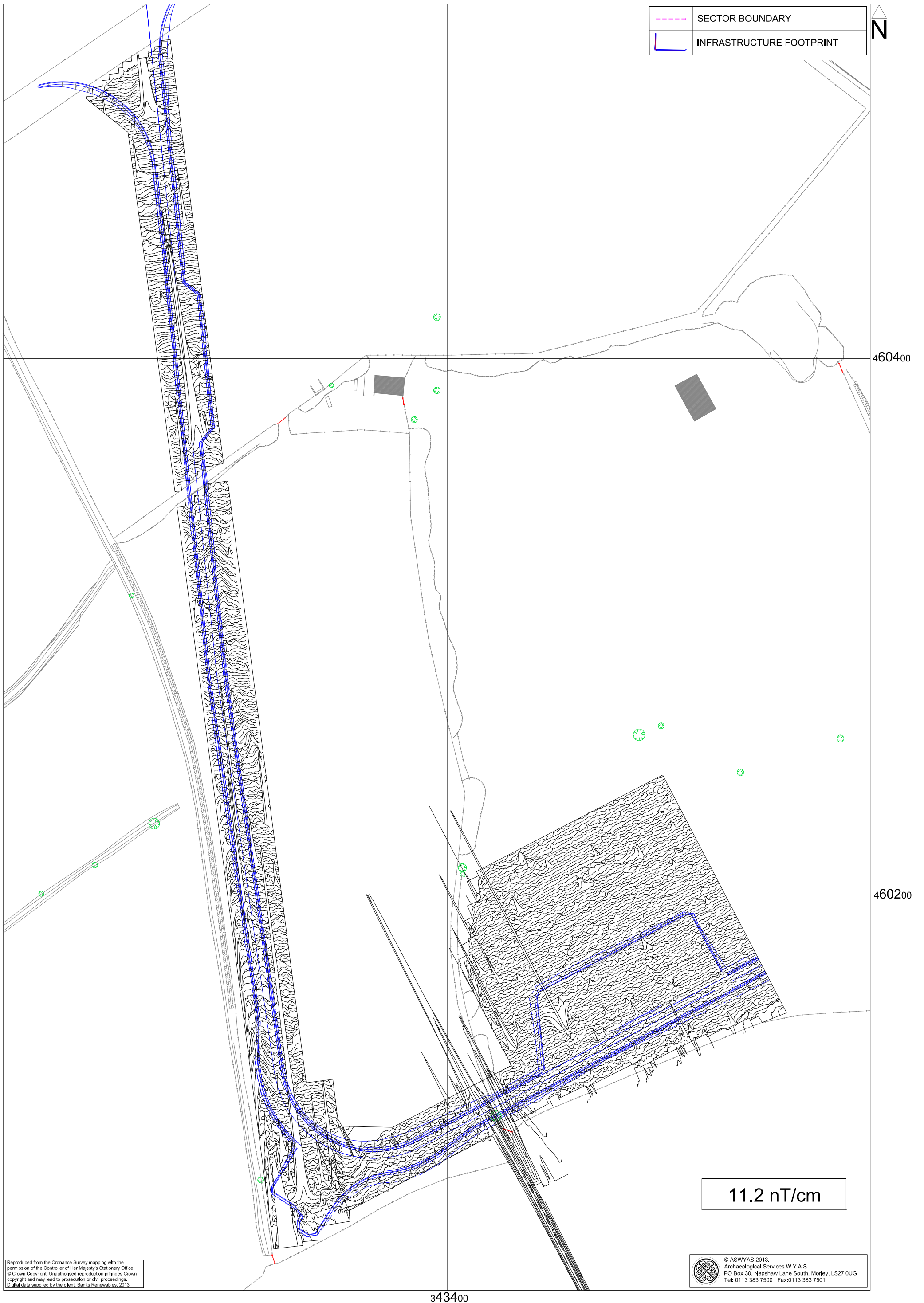
Fig. 11. XY trace plot of minimally processed magnetometer data; Turbine 3 and Access Track 3 (1:1000 @ A3)
