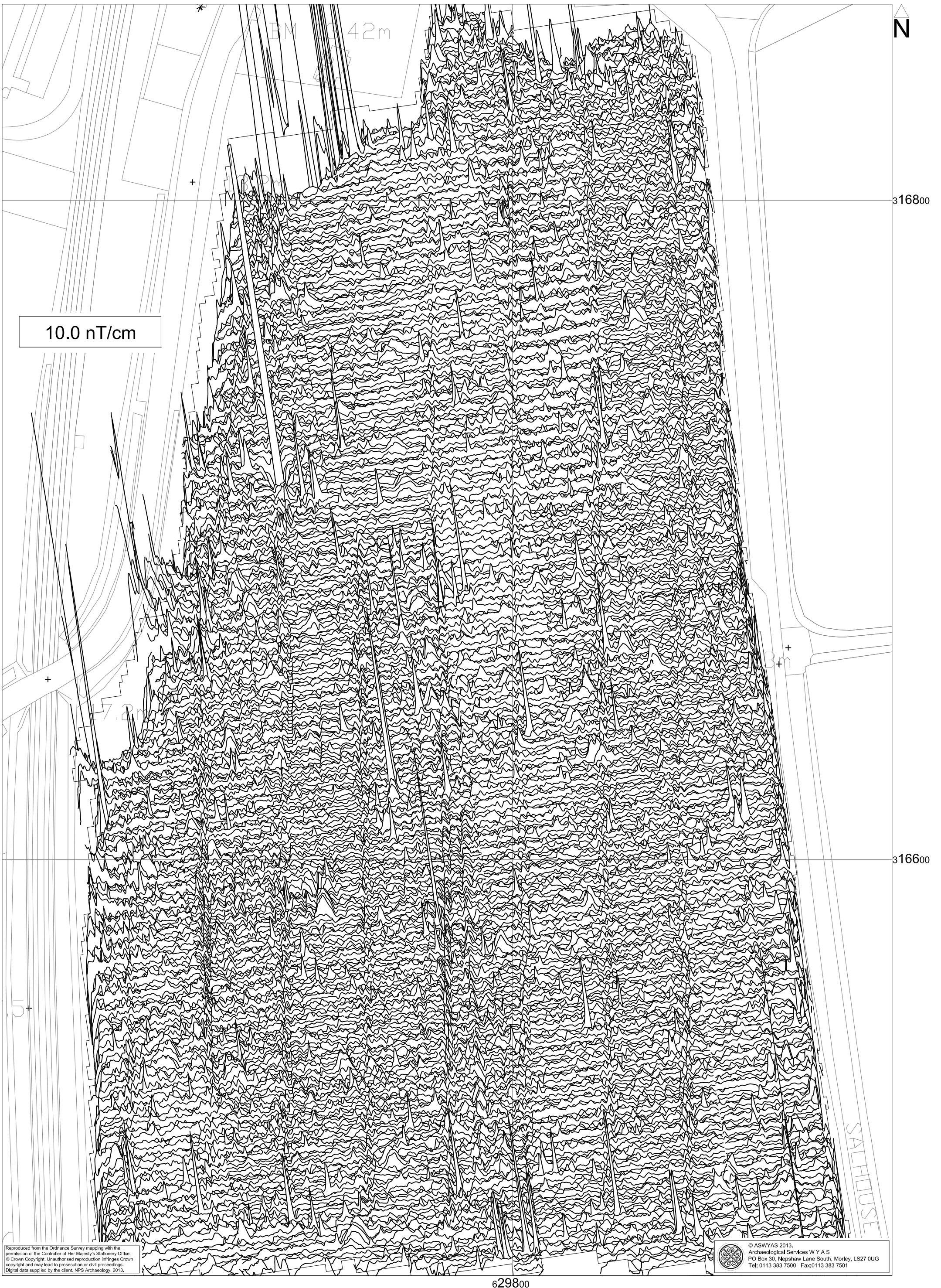
XY trace plot of raw magnetometer data (1:1000 @ A3)
