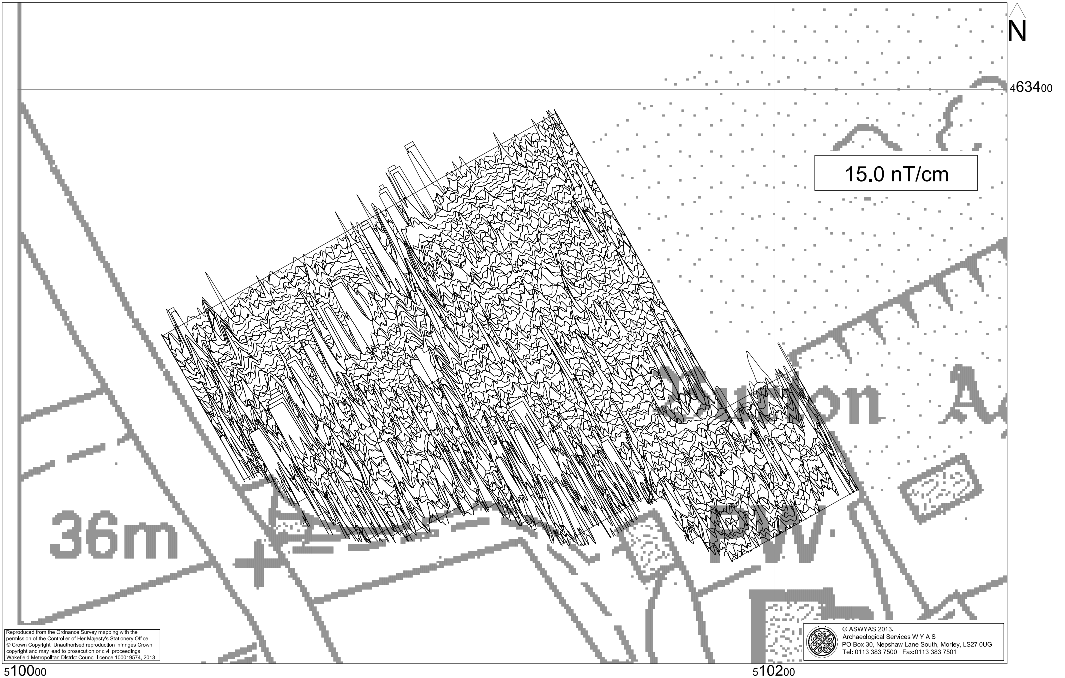
Fig. 5. XY trace plot of minimally processed magnetometer data (1:1000 @ A4)
