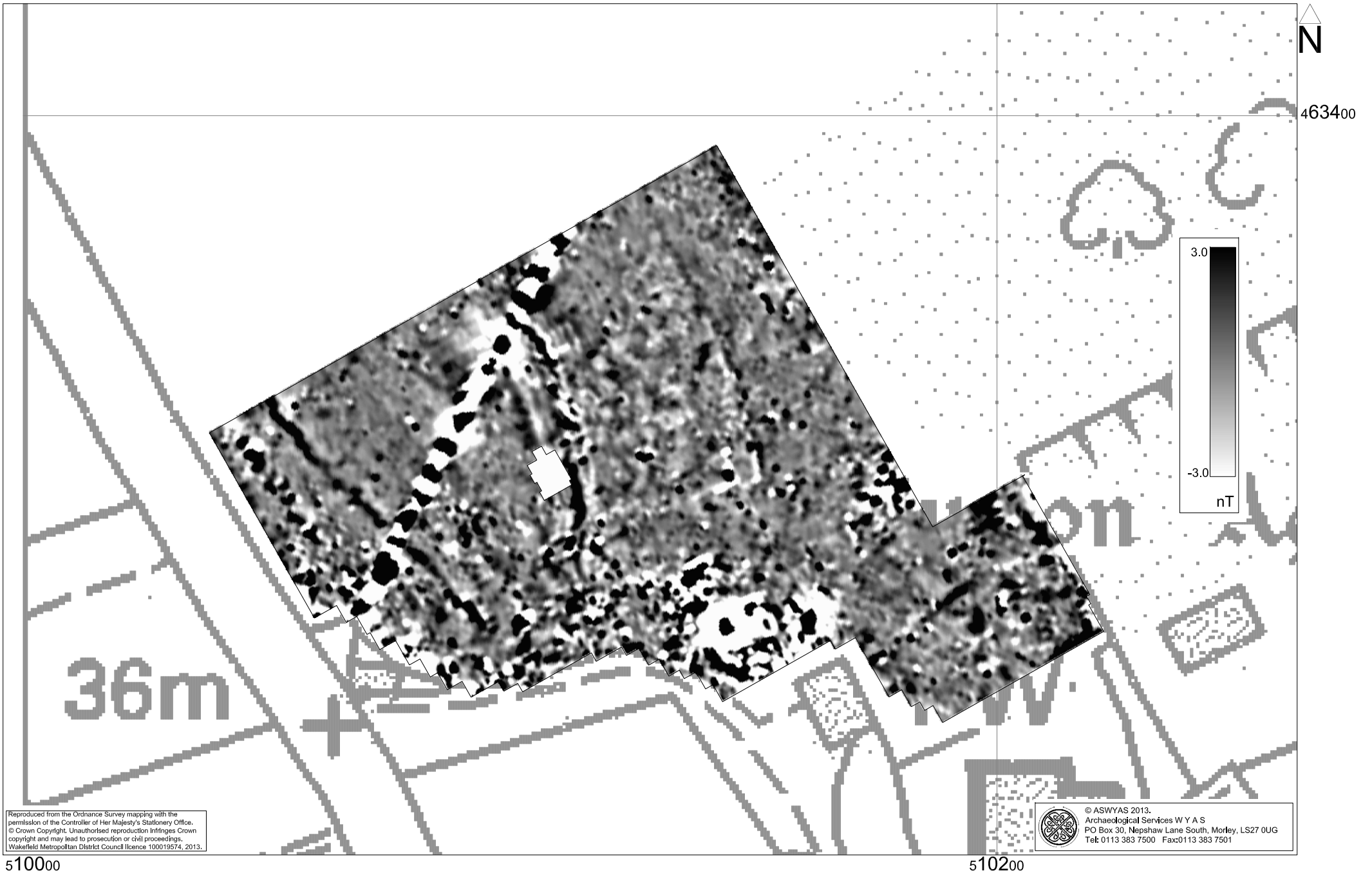
Fig. 4. Processed greyscale magnetometer data (1:1000 @ A4)
