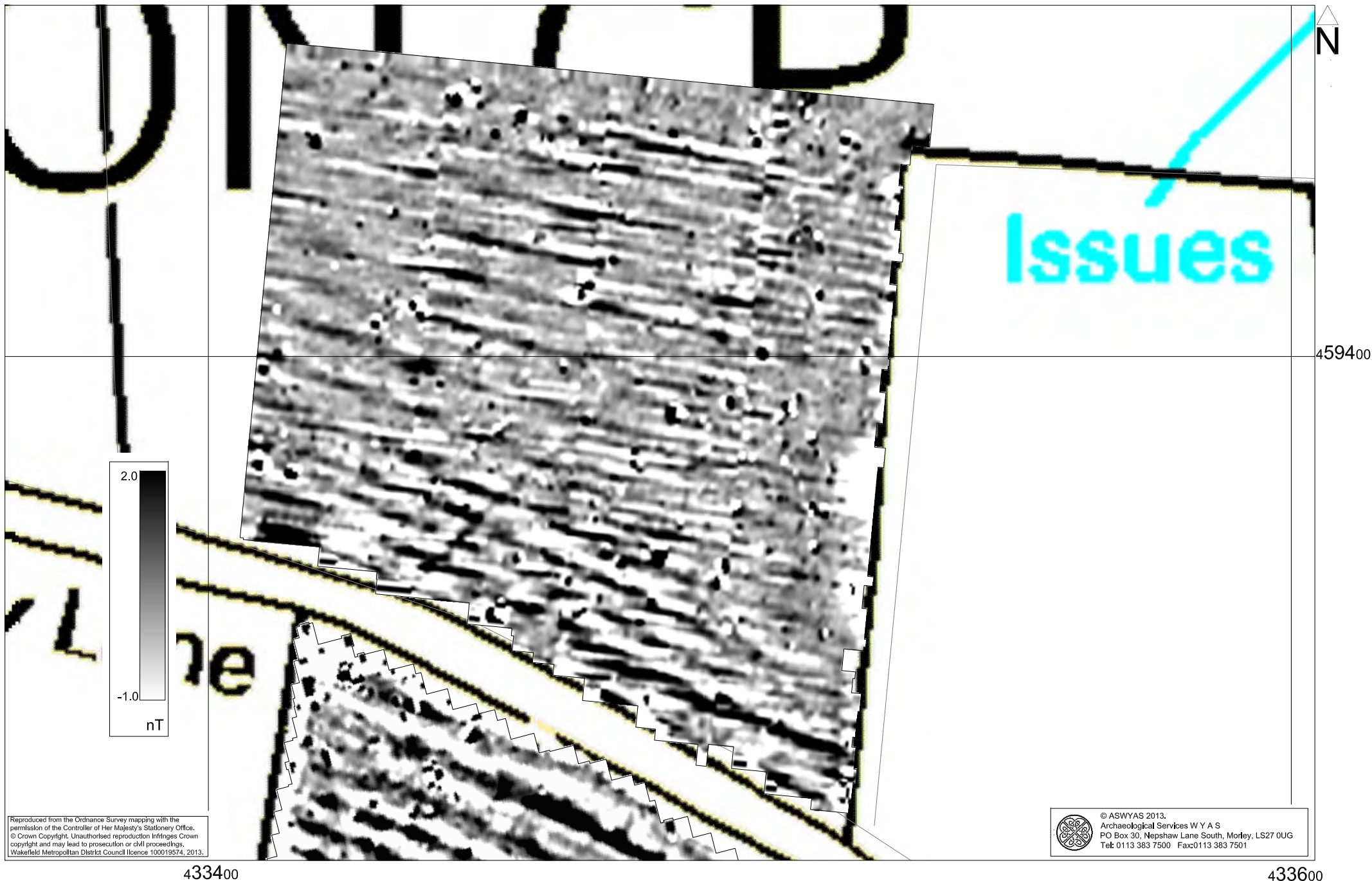
Fig. 21. Processed greyscale magnetometer data; Knaresborough, Area 8 (1:1000 @ A4)
