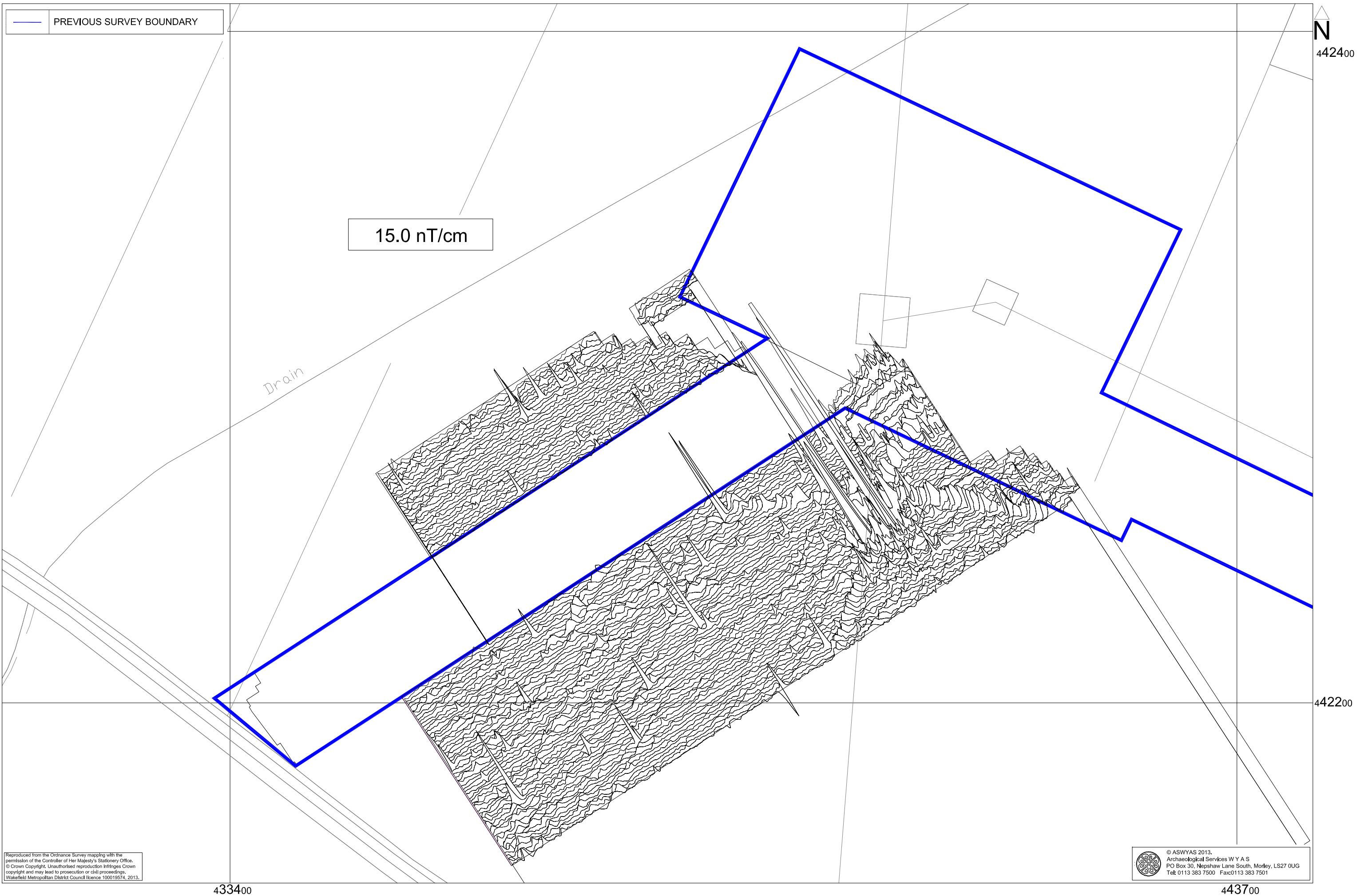
Fig. 7. XY trace plot of minimally processed magnetometer data; Bramham, Area 1 (1:1000 @ A3)
