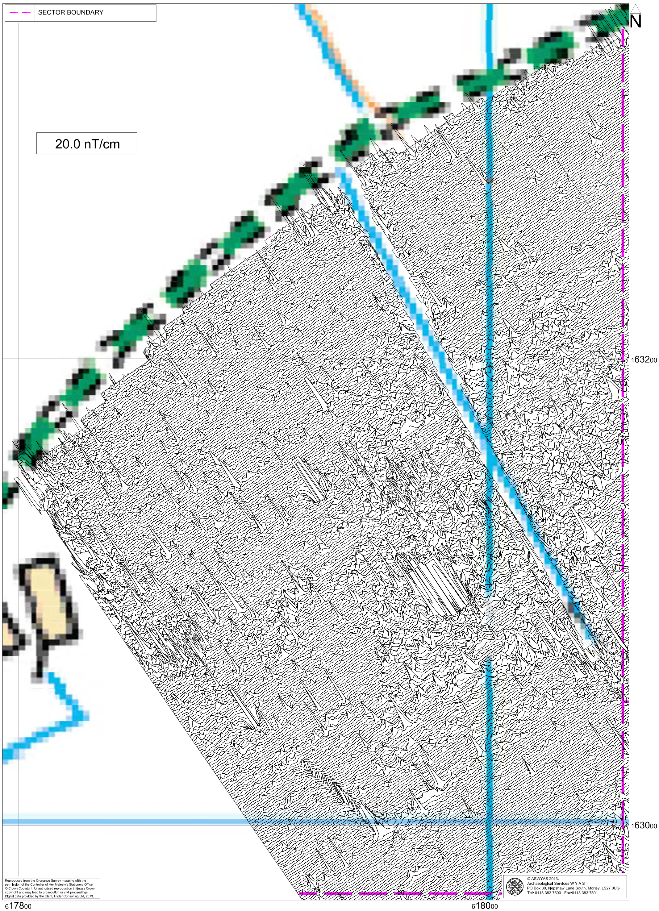
Fig. 8. XY trace plot of minimally processed magnetometer data; Field 1, Sector 2 (1:1000 @ A3)
