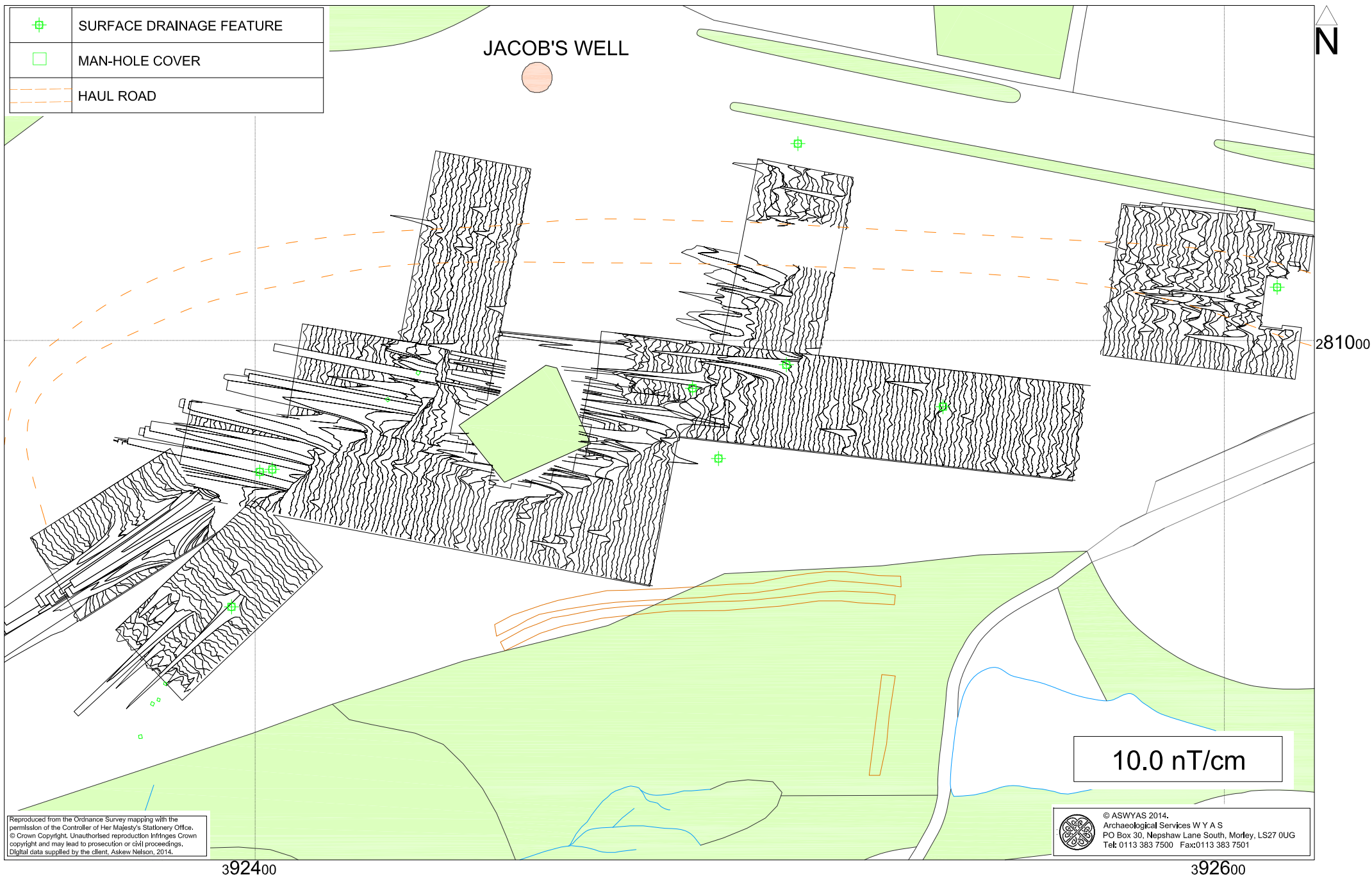
Fig. 4. XY trace plot of minimally processed magnetometer data (1:1000 @ A4)
