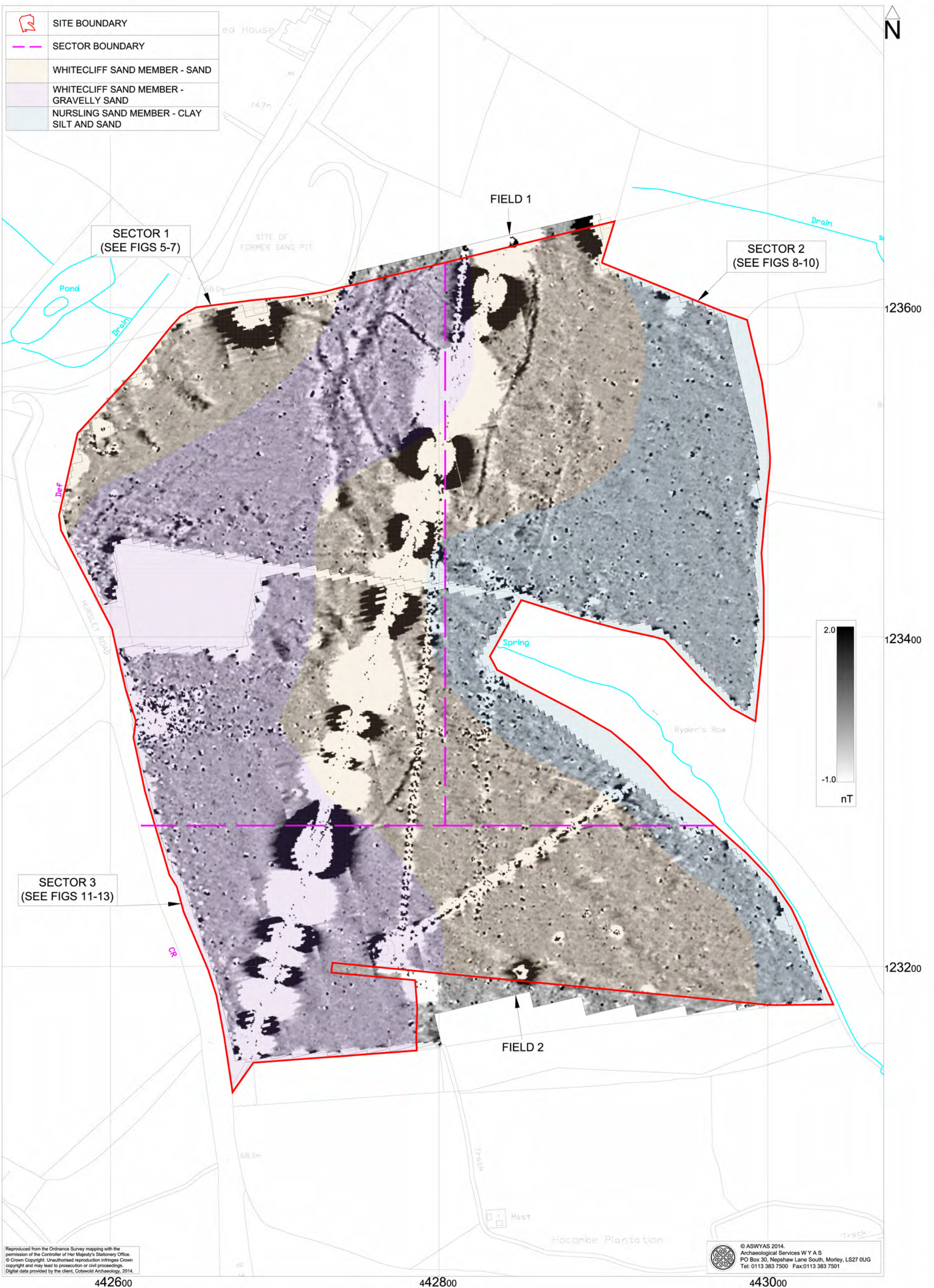
Fig. 3. Processed greyscale magnetometer data showing geology detail (1:2000 @ A3)
