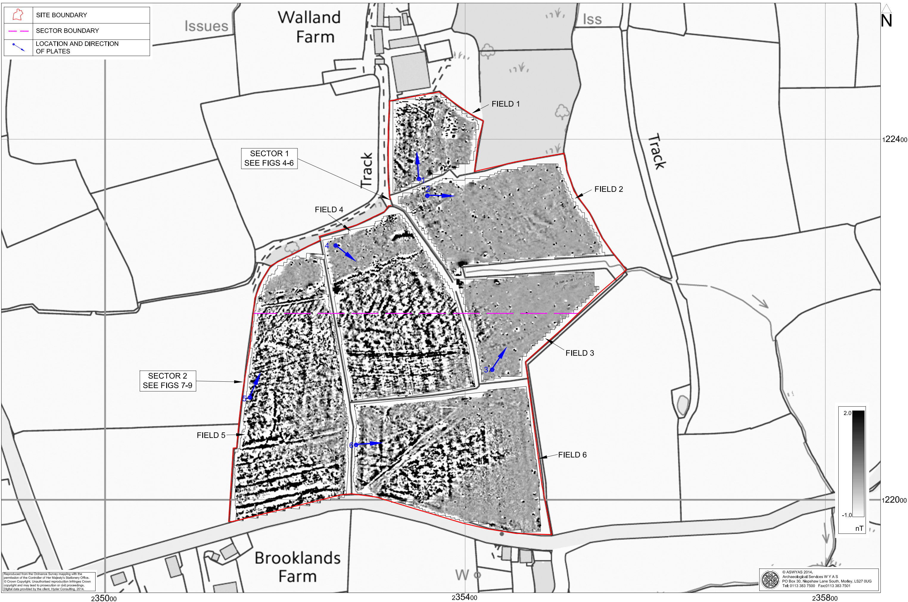
Fig. 2. Site location showing greyscale magnetometer data (1:2500 @ A3)
