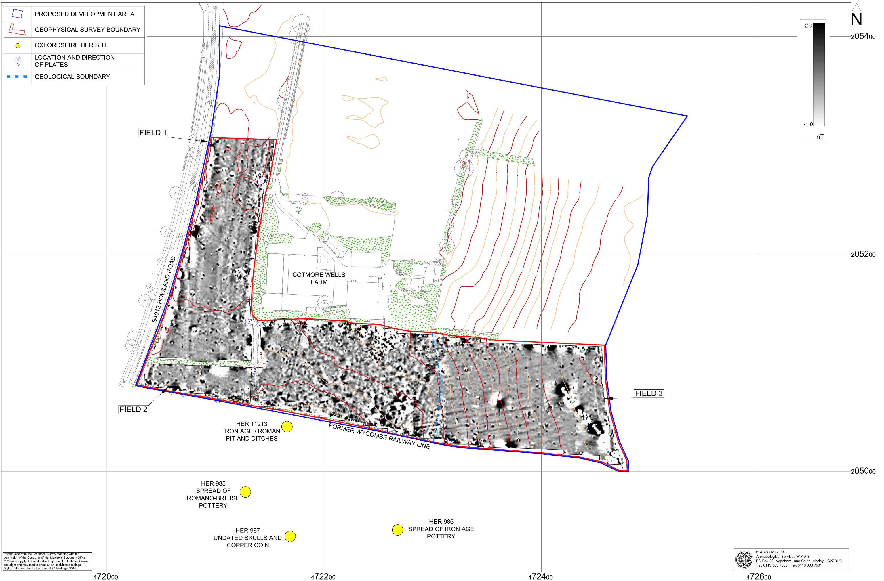
Fig. 2. Site location showing greyscale magnetometer data, contour detail and Oxfordshire HER data (1:2000 @ A3)
