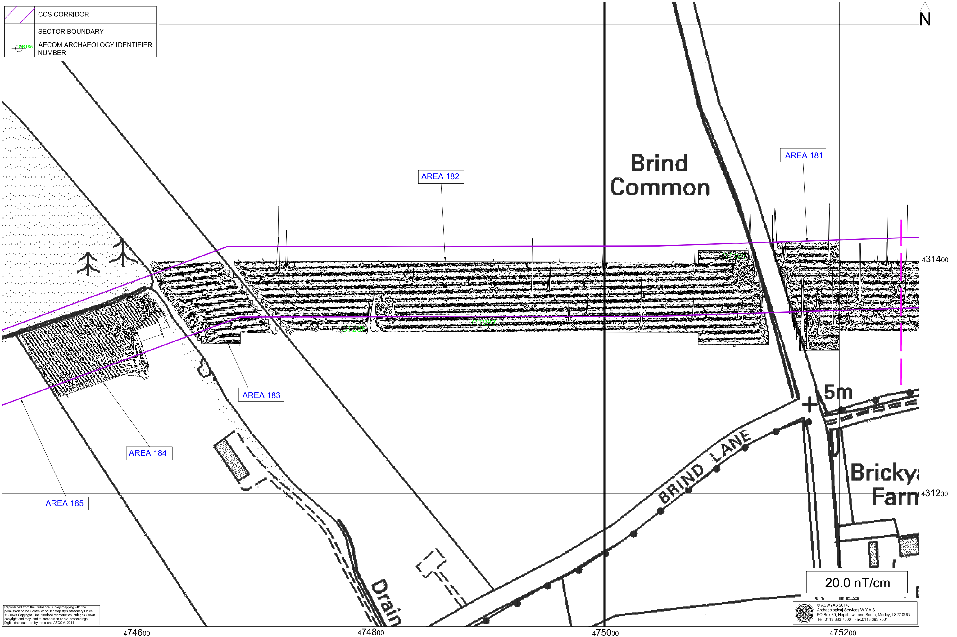
Fig. 52. XY trace plot of minimally processed magnetometer data; Sector 8 (1:2000 @ A3)
