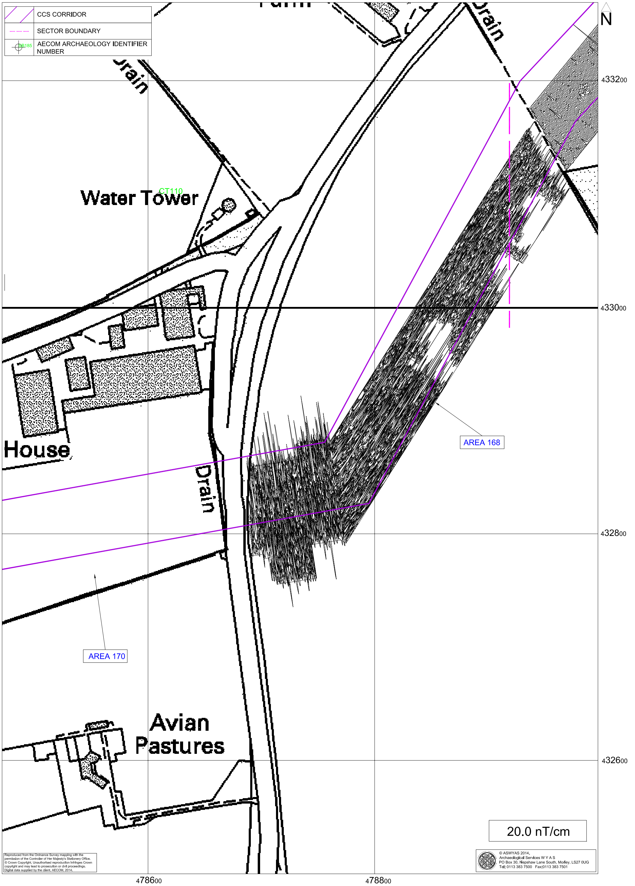
Fig. 58. XY trace plot of minimally processed magnetometer data; Sector 11 (1:2000 @ A3)
