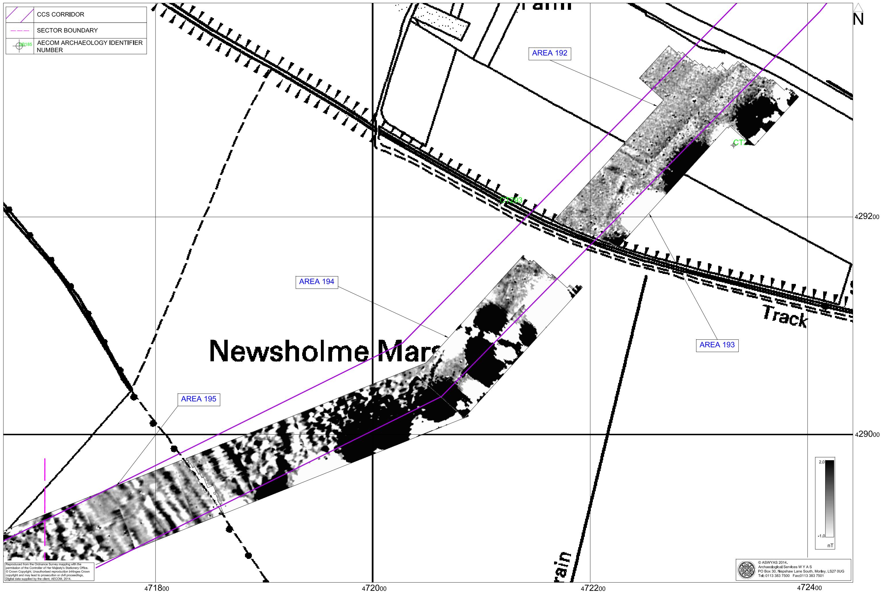
Fig. 42. Processed greyscale magnetometer data; Sector 5 (1:2000 @ A3)
