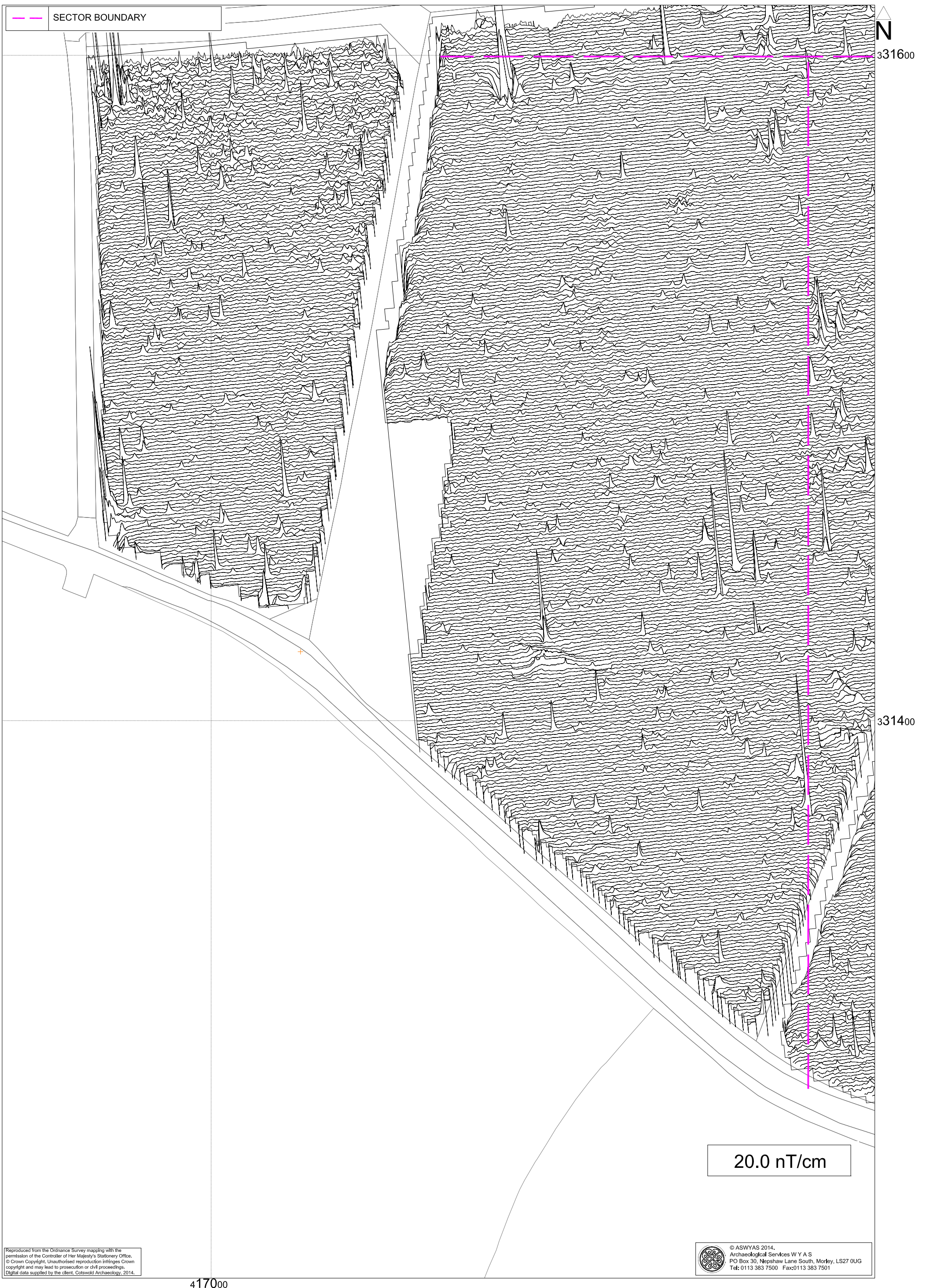
Fig. 15. XY trace plot of minimally processed magnetometer data; Sector 4 (1:1000 @ A3)
