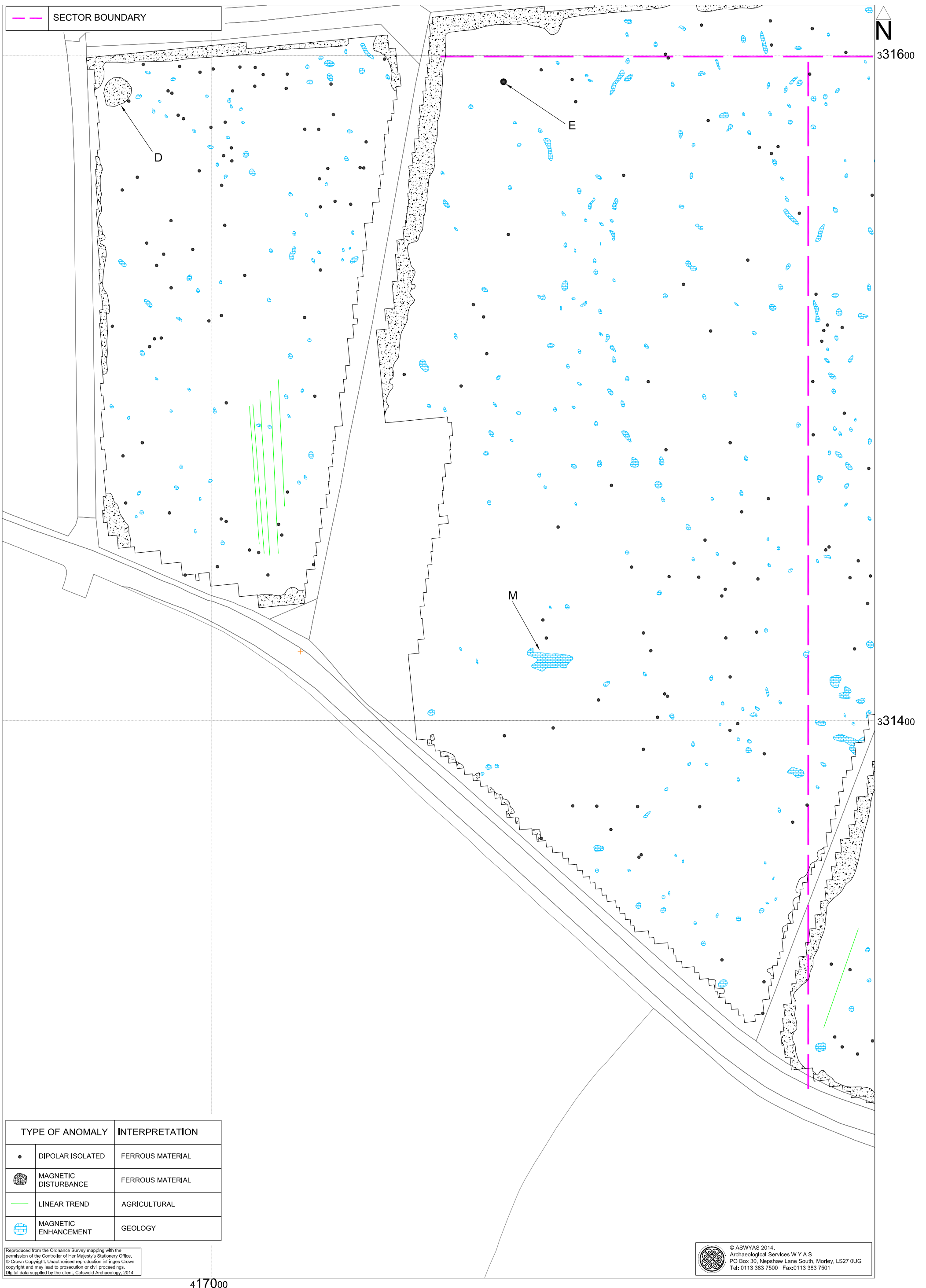
Fig. 16. Interpretation of magnetometer data; Sector 4 (1:1000 @ A3)
