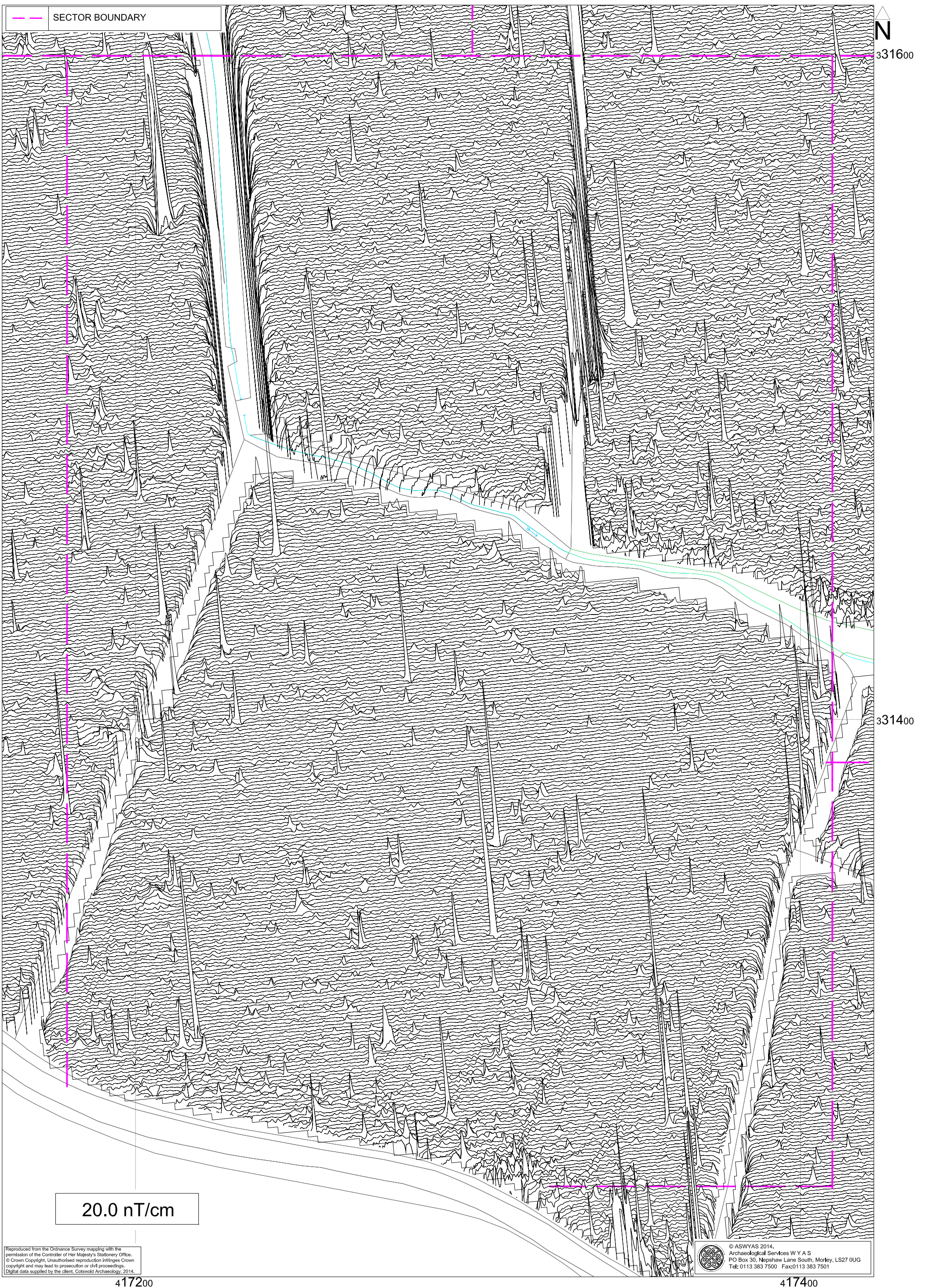
Fig. 18. XY trace plot of minimally processed magnetometer data; Sector 5 (1:1000 @ A3)
