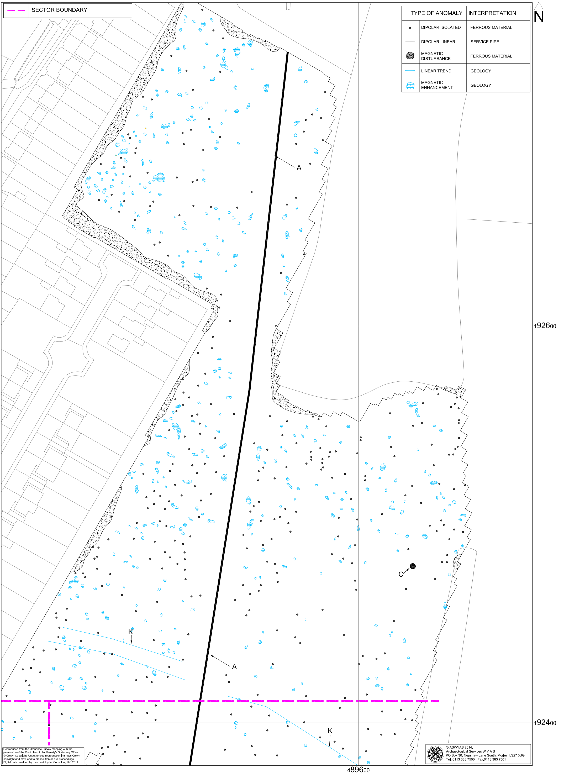
Fig. 9. Interpretation of magnetometer data; Sector 2 (1:1000 @ A3)
