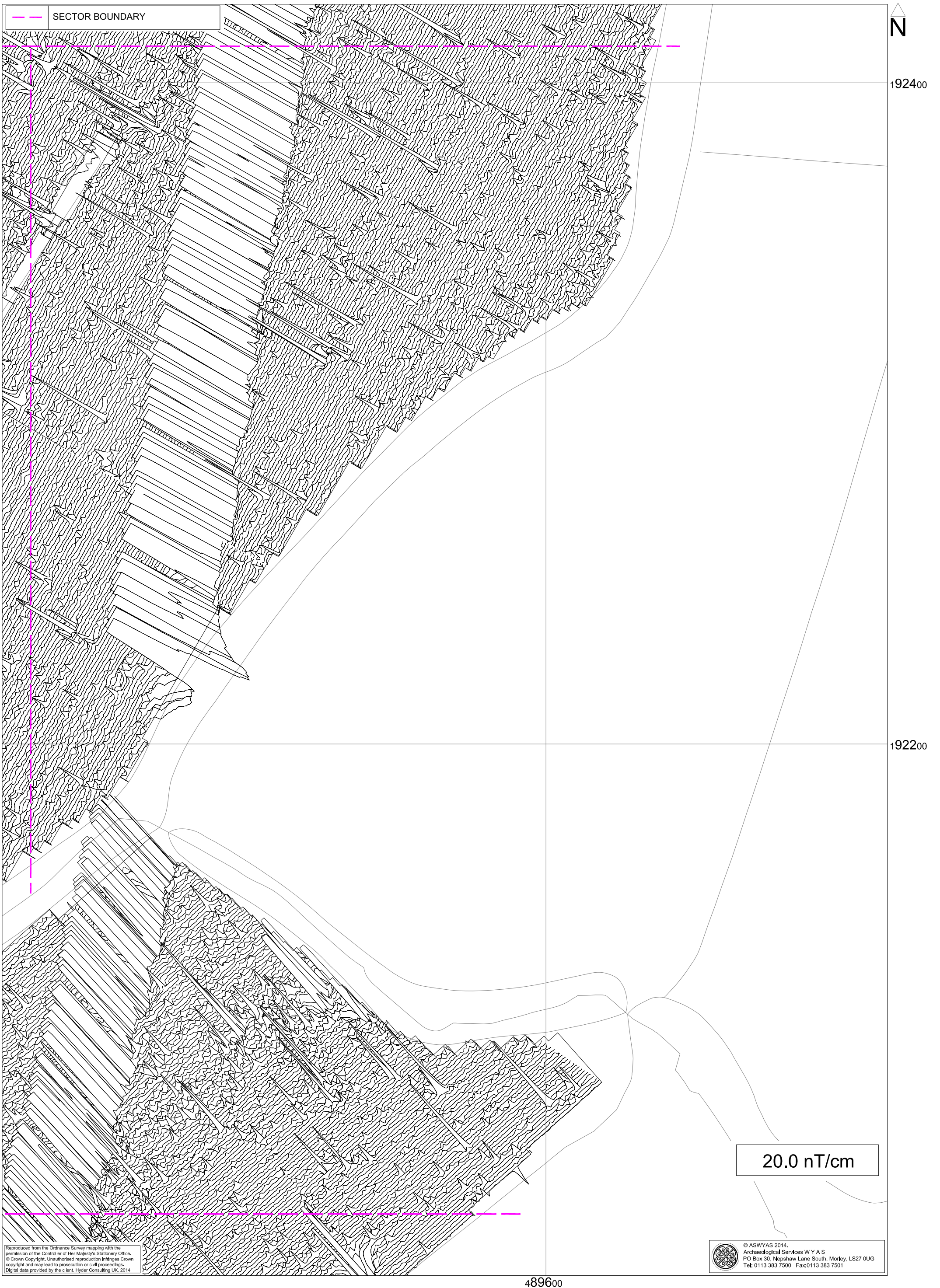
Fig. 14. XY trace plot of minimally processed magnetometer data; Sector 4 (1:1000 @ A3)
