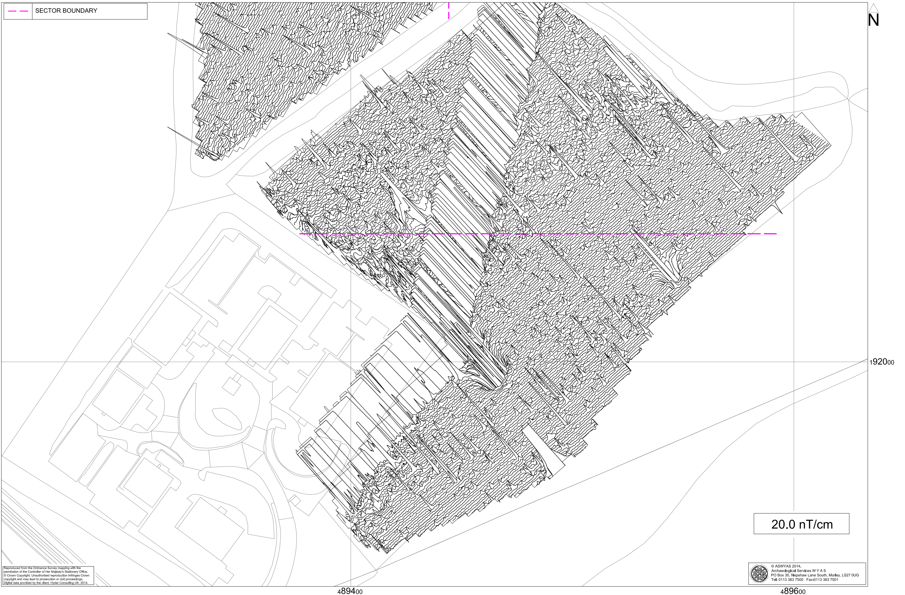
Fig. 17. XY trace plot of minimally processed magnetometer data; Sector 5 (1:1000 @ A3)
