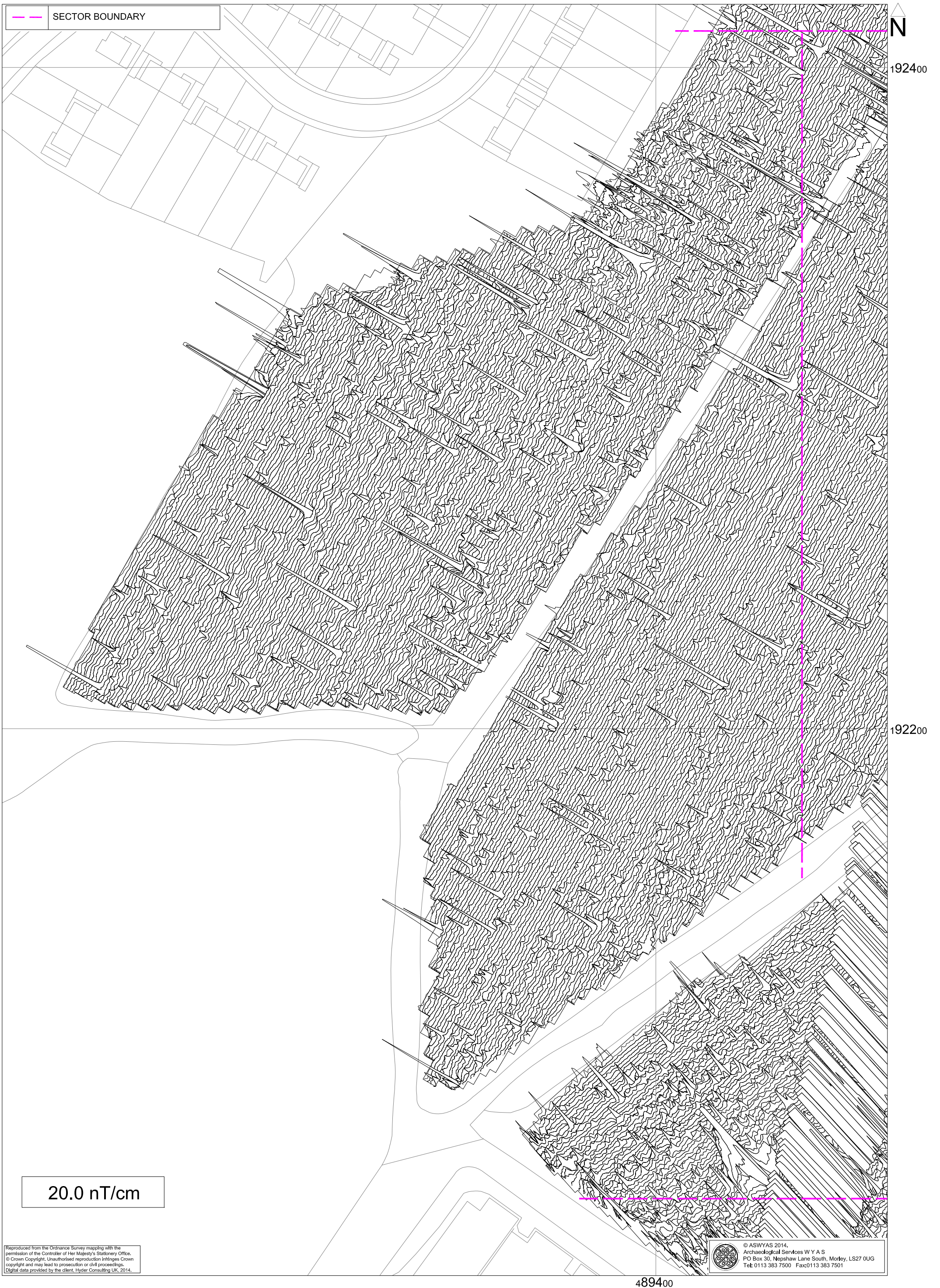
Fig. 11. XY trace plot of minimally processed magnetometer data; Sector 3 (1:1000 @ A3)
