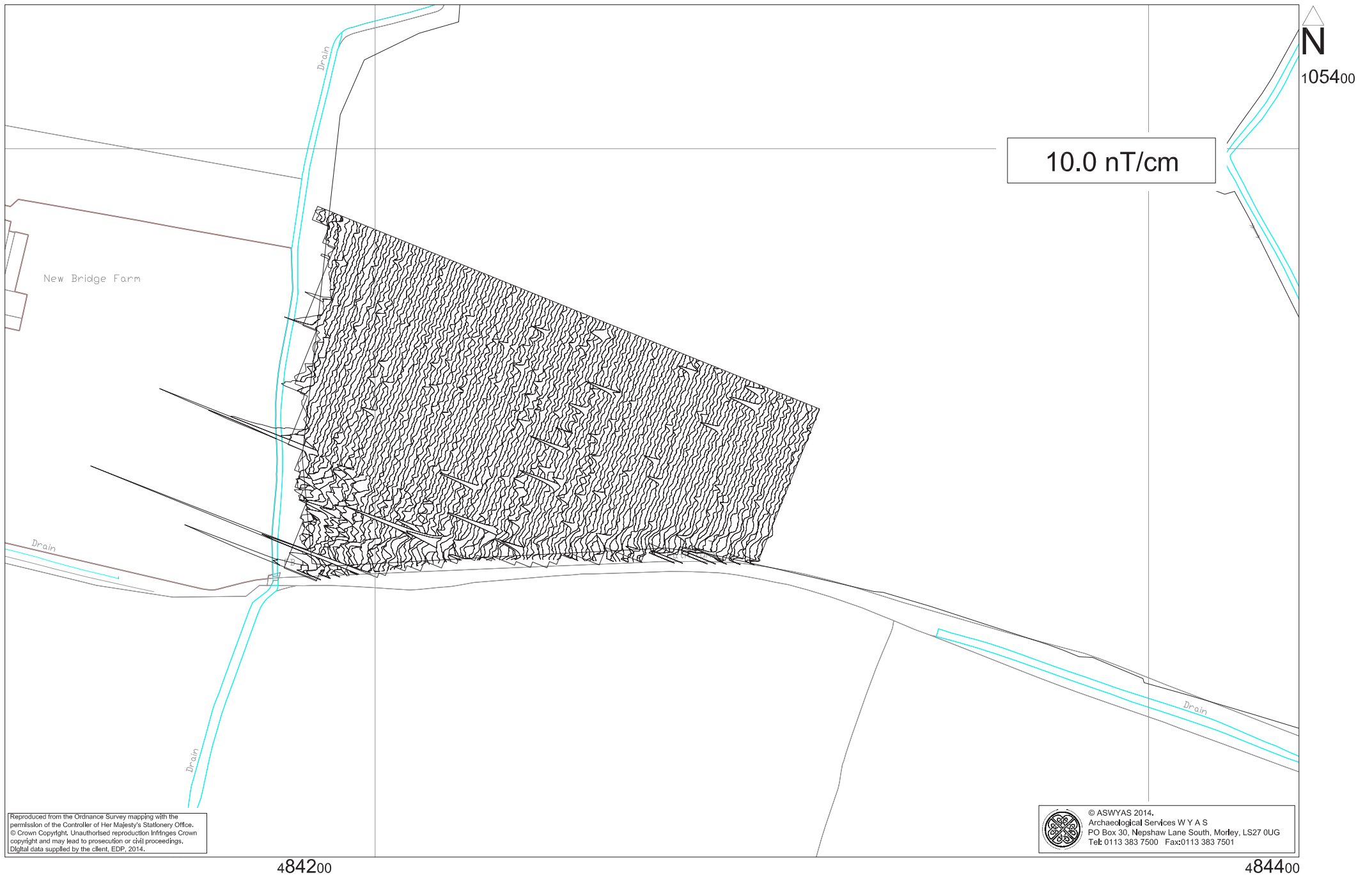
Fig. 6. XY trace plot of minimally processed magnetometer data - Bartington hand carry system (1:1250 @ A4)
