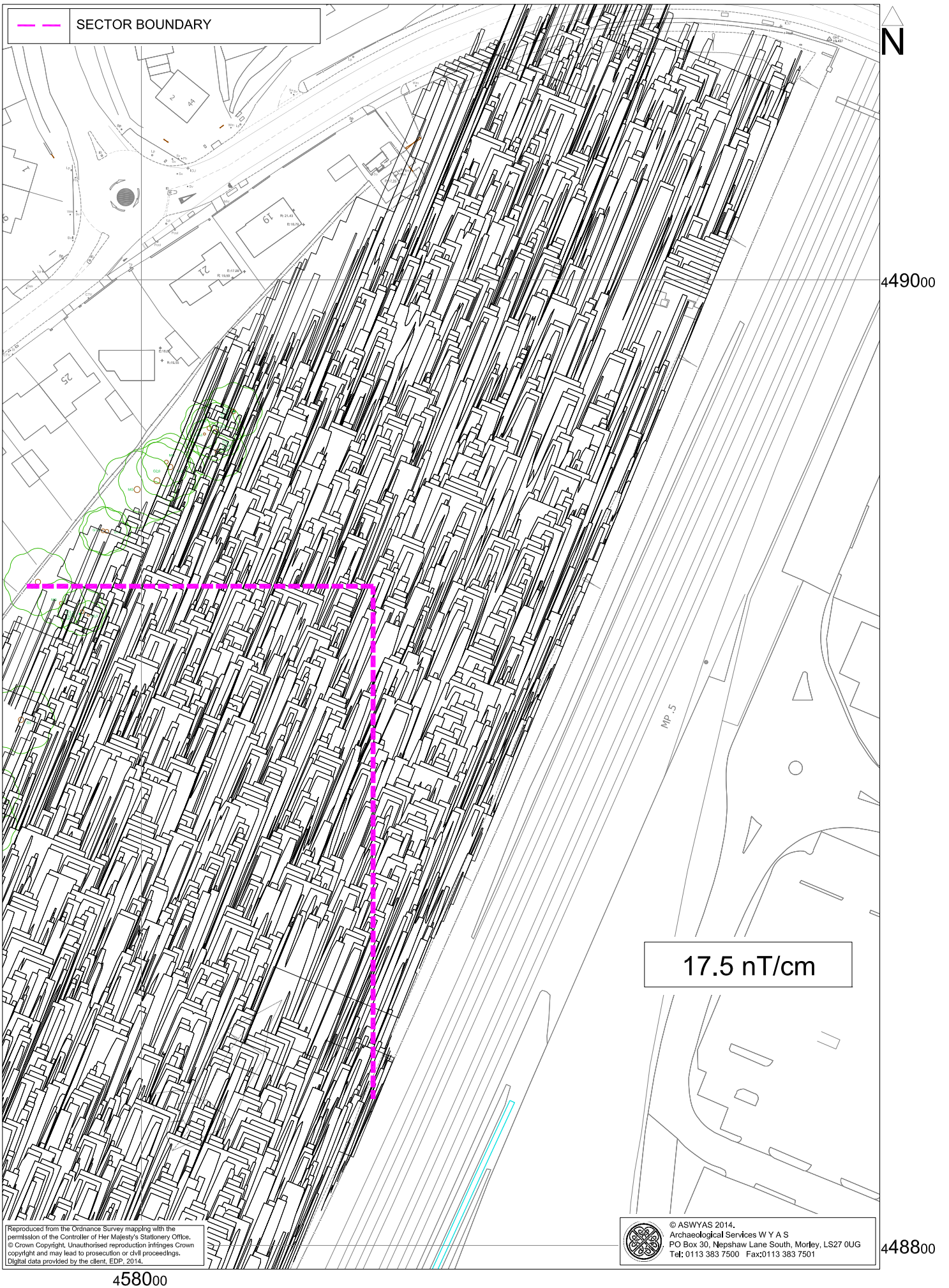
Fig. 49. XY trace plot of minimally processed magnetometer data; Sector 15 (1:1000 @ A4)
