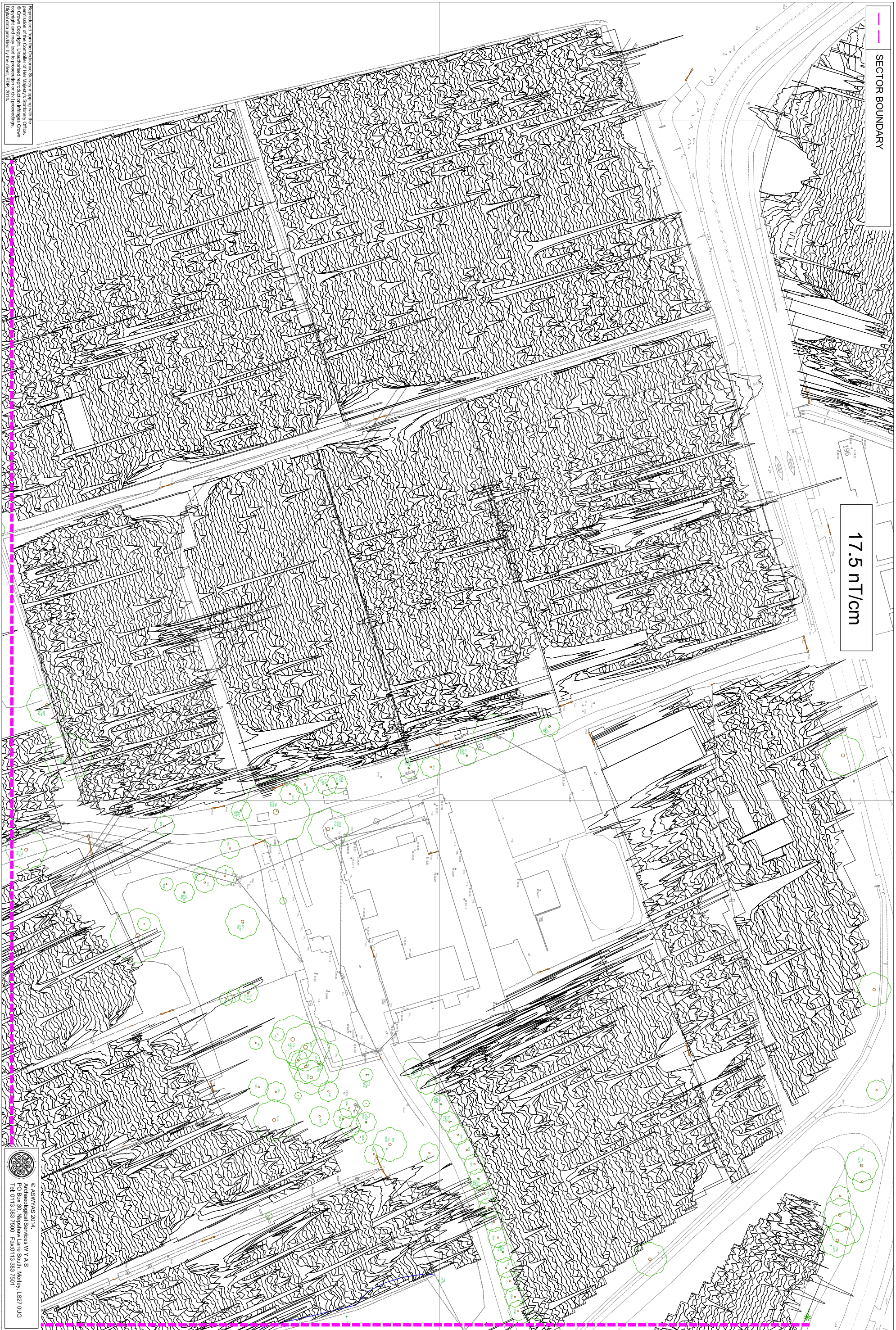
Fig. 13. XY trace plot of minimally processed magnetometer data; Sector 3 (1:1000 @ A3)
