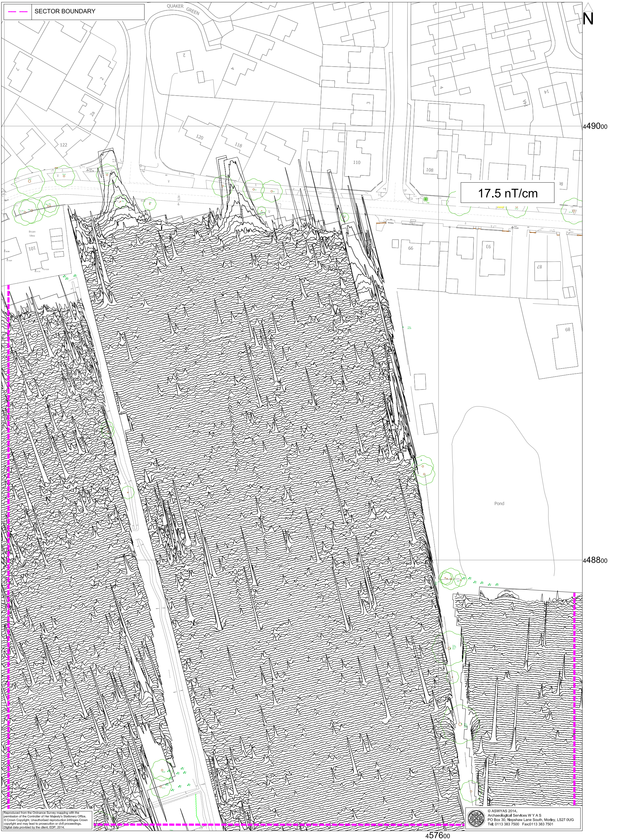
Fig. 37. XY trace plot of minimally processed magnetometer data; Sector 11 (1:1000 @ A3)
