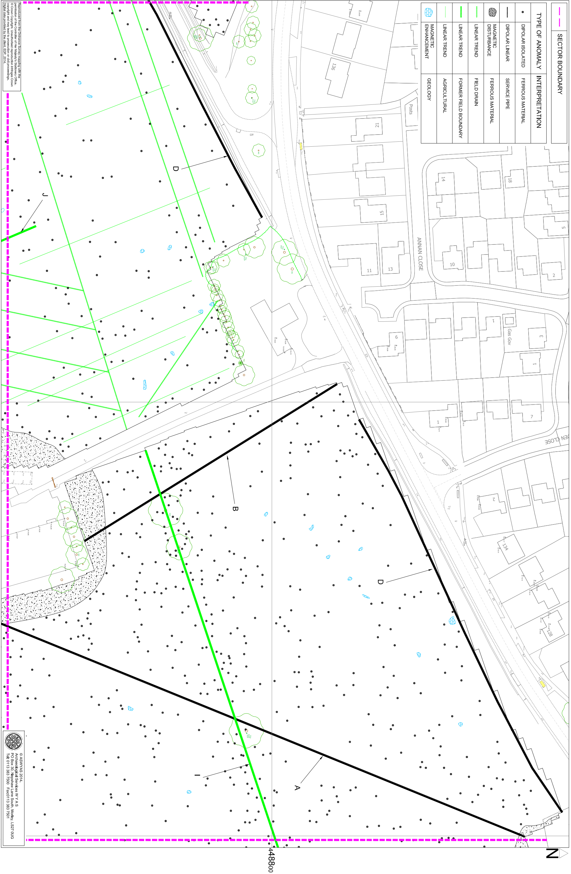
Fig. 29. Interpretation of magnetometer data; Sector 8 (1:1000 @ A3)
