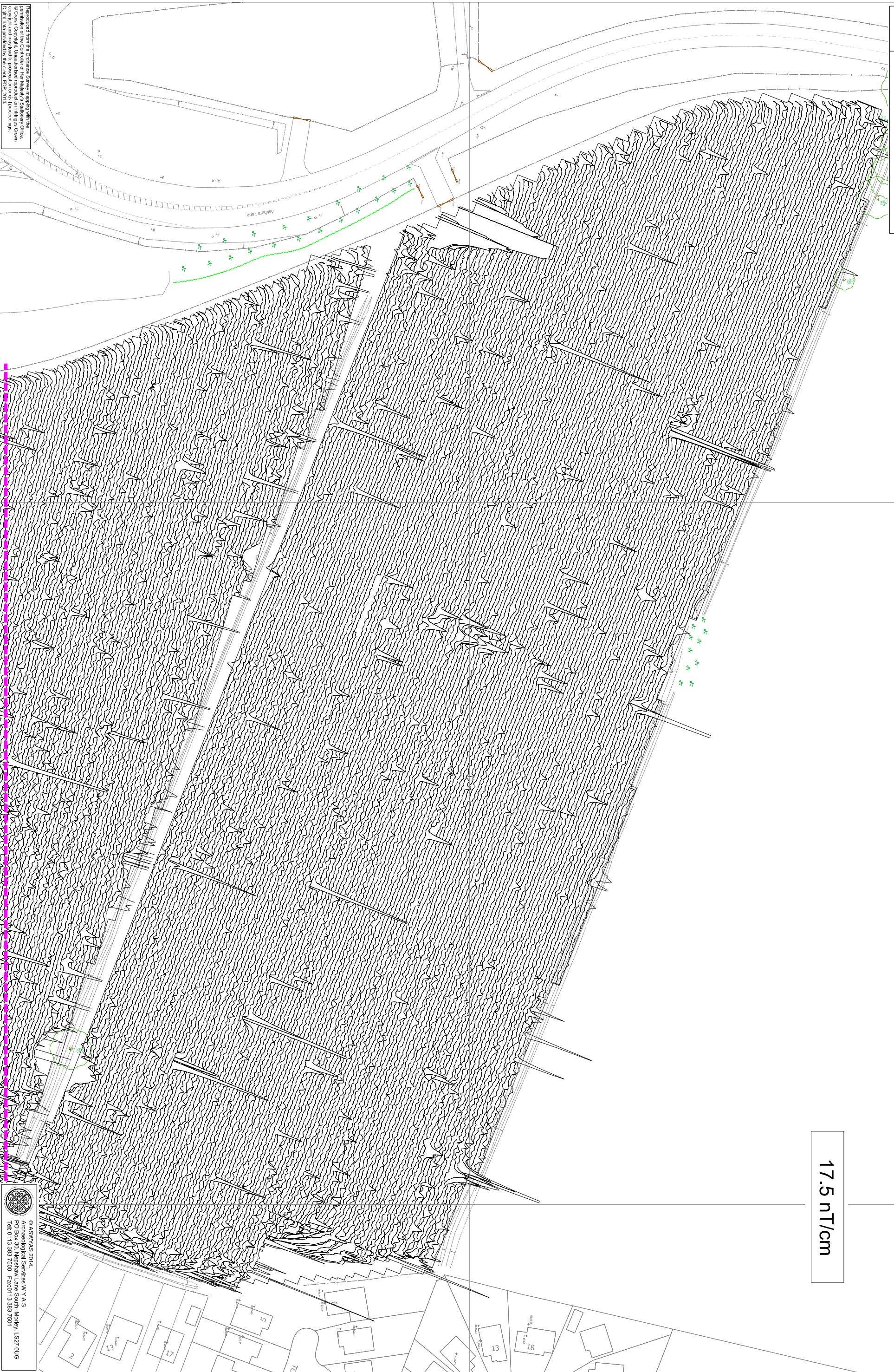
Fig. 7. XY trace plot of minimally processed magnetometer data; Sector 1 (1:1000 @ A3)
