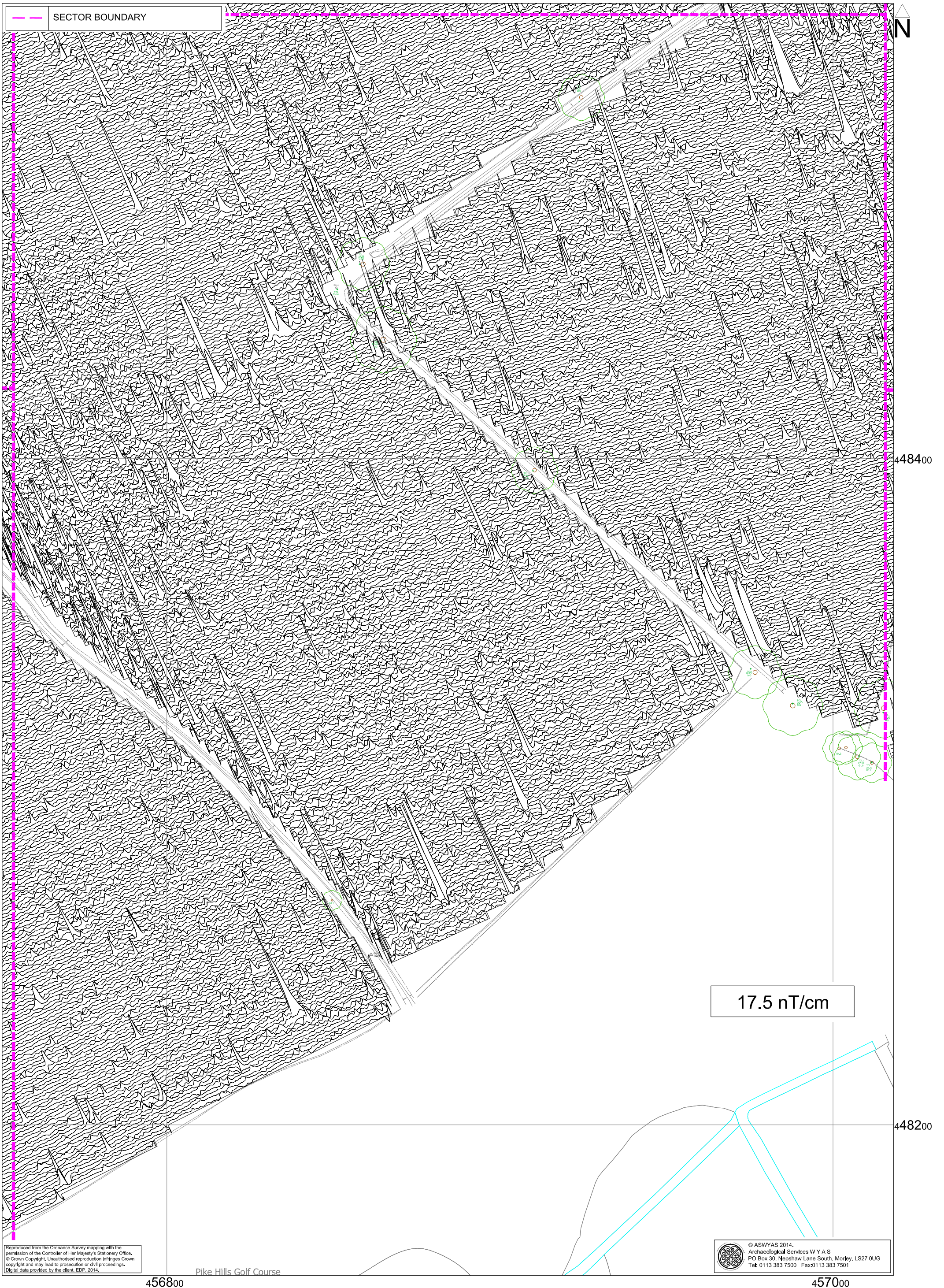
Fig. 40. XY trace plot of minimally processed magnetometer data; Sector 12 (1:1000 @ A3)
