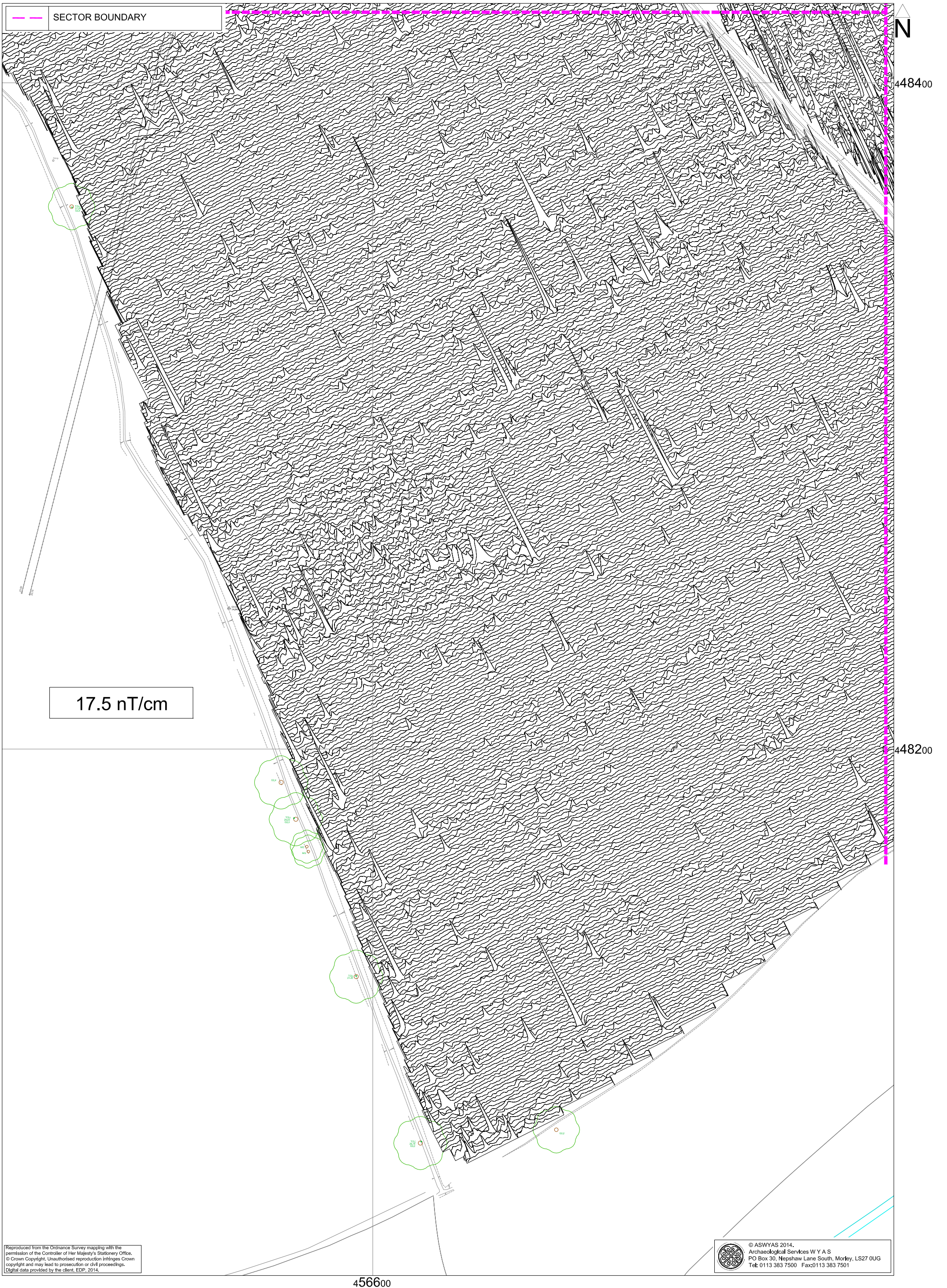
Fig. 19. XY trace plot of minimally processed magnetometer data; Sector 5 (1:1000 @ A3)
