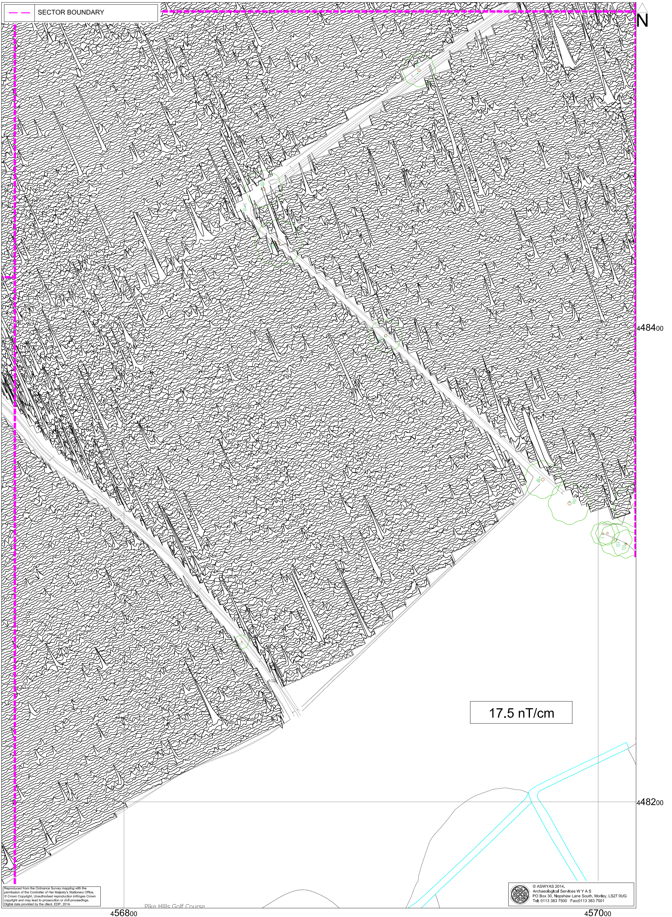
Fig. 25. XY trace plot of minimally processed magnetometer data; Sector 7 (1:1000 @ A3)
