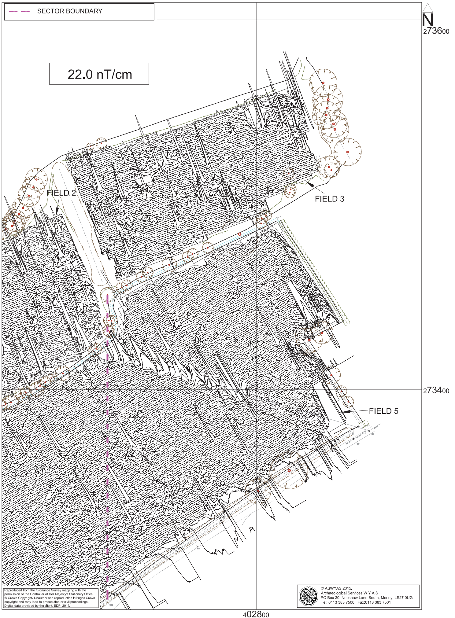
Fig. 8. XY trace plot of minimally processed magnetometer data; Sector 2 (1:1250 @ A4)
