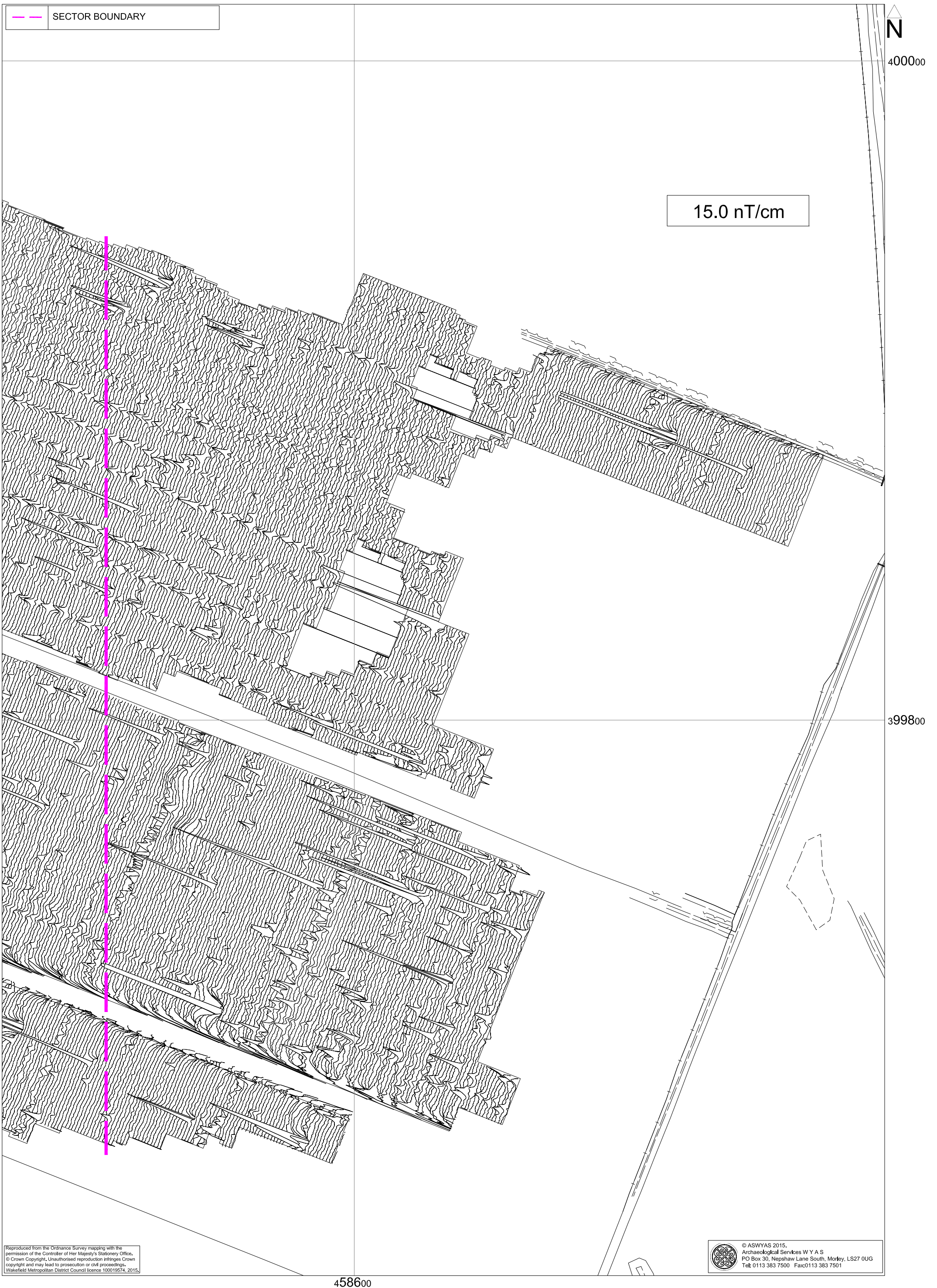
Fig. 11. XY trace plot of minimally processed magnetometer data; Area A, Sector 3 (1:1000 @ A3)
