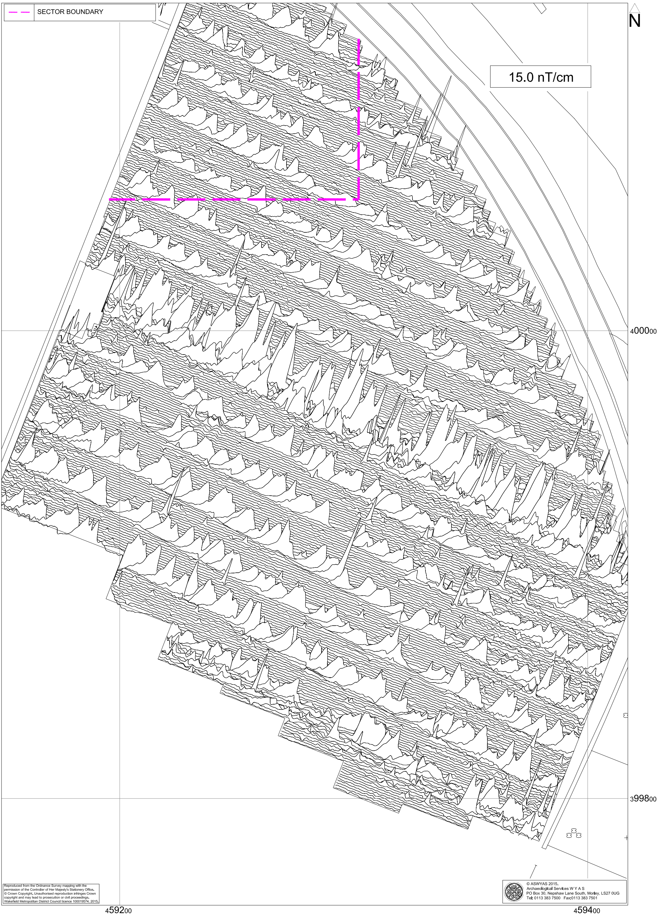
Fig. 17. XY trace plot of minimally processed magnetometer data; Area C (1:1000 @ A3)
