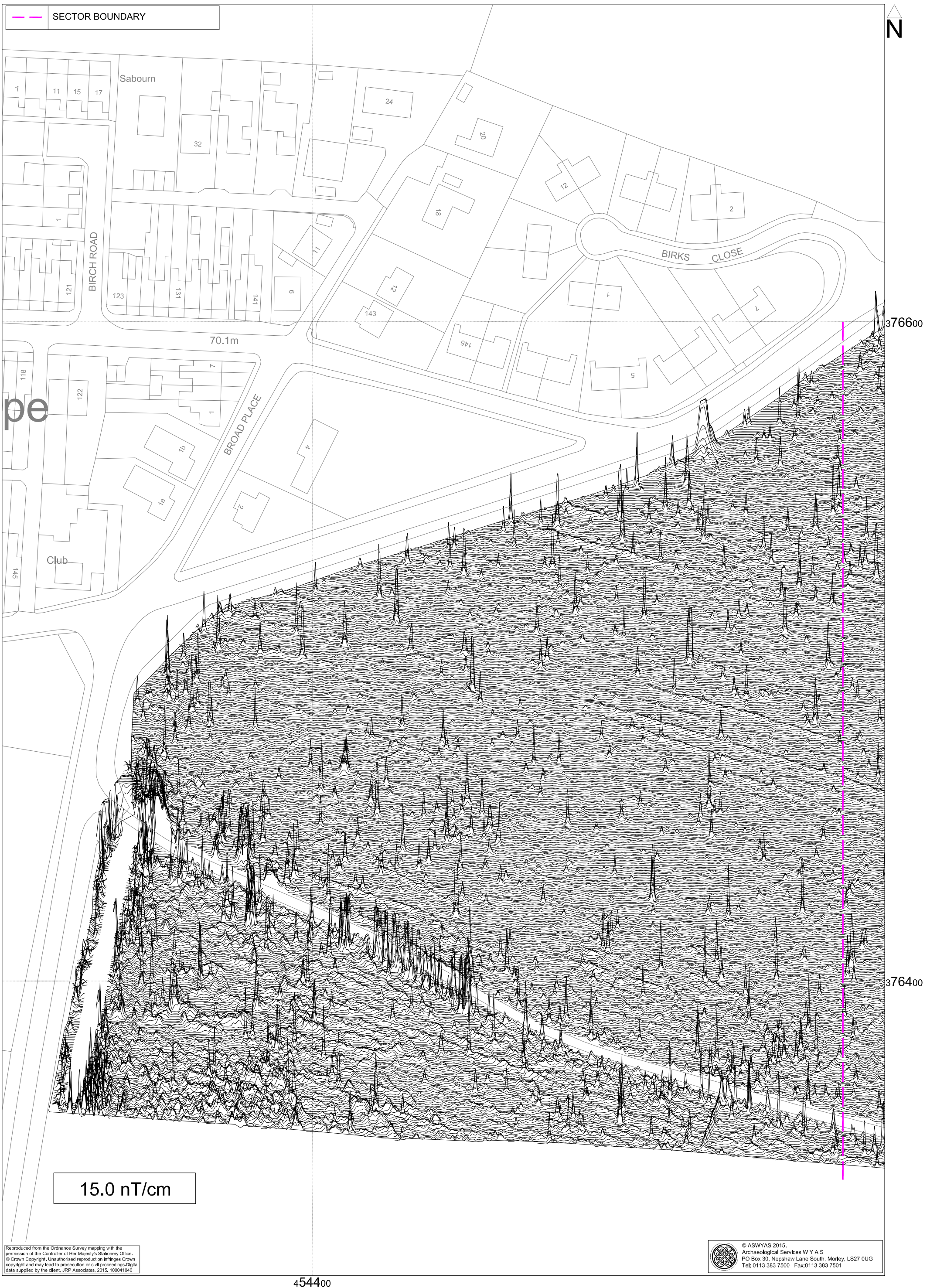
Fig. 6. XY trace plot of minimally processed magnetometer data; Sector 1 (1:1000 @ A3)
