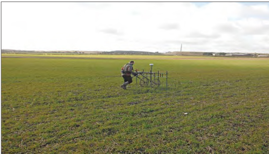
Plate 3. The Sensys Magneto MXPDA five sensor cart-based magnetometer system
