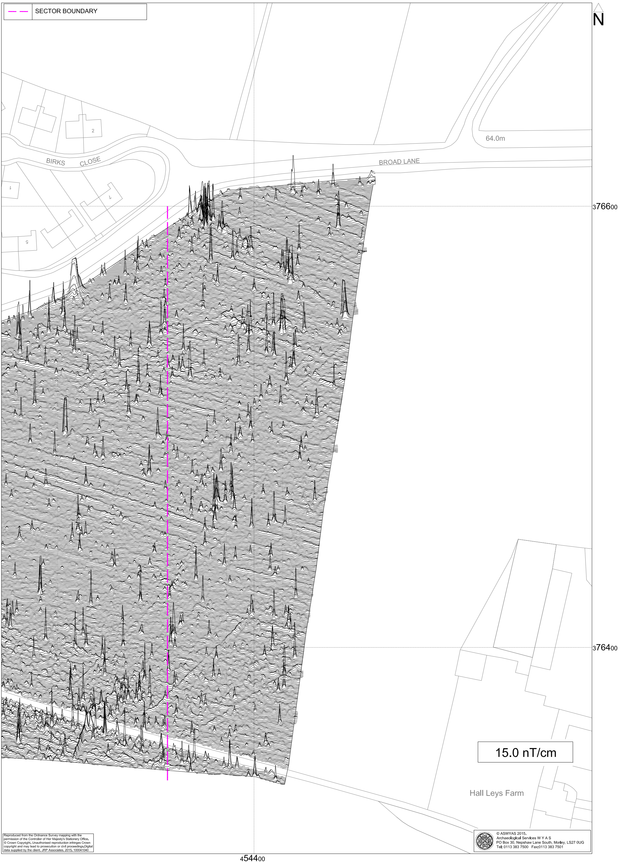
Fig. 9. XY trace plot of minimally processed magnetometer data; Sector 2 (1:1000 @ A3)
