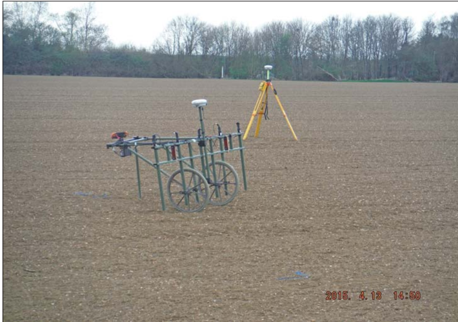
Plate 1. The Sensys Magneto MXPDA five sensor cart-based magnetometer system
