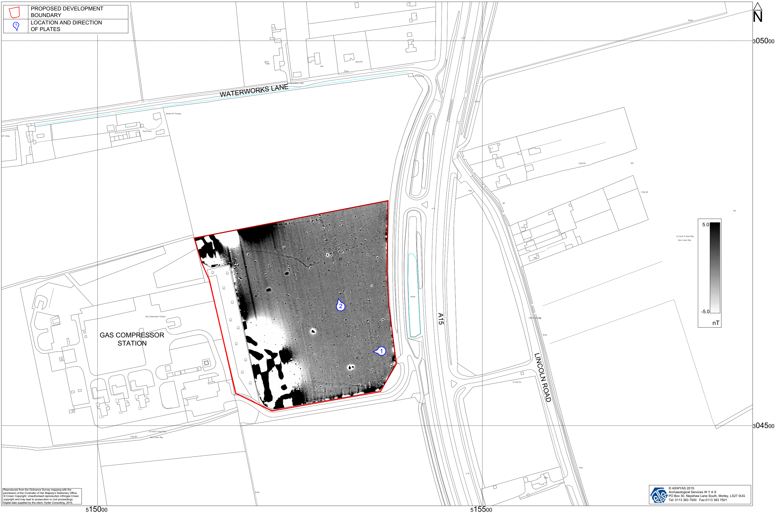
Fig. 2. Survey location showing greyscale magnetometer data (1:2500 @ A3)
