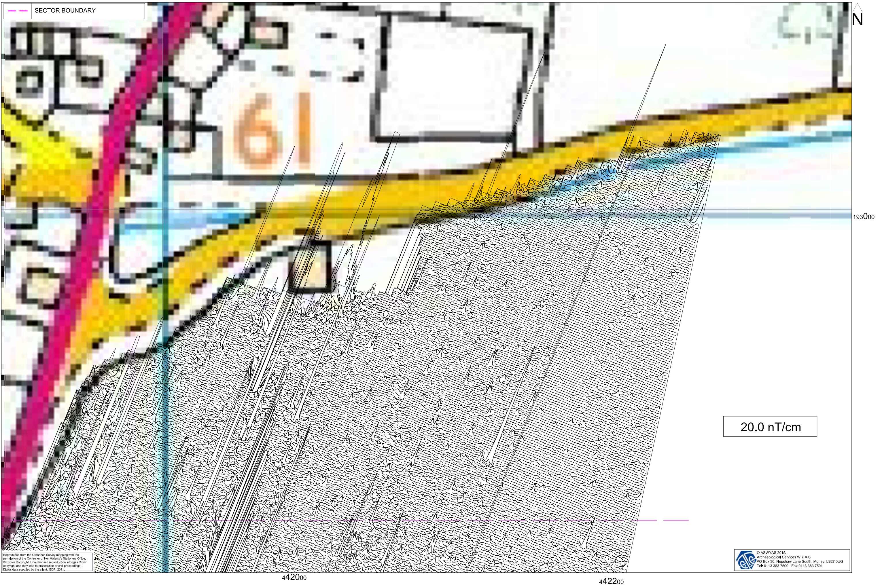
Fig. 5. XY trace plot of minimally processed magnetometer data; Sector 1 (1:1000 @ A3)
