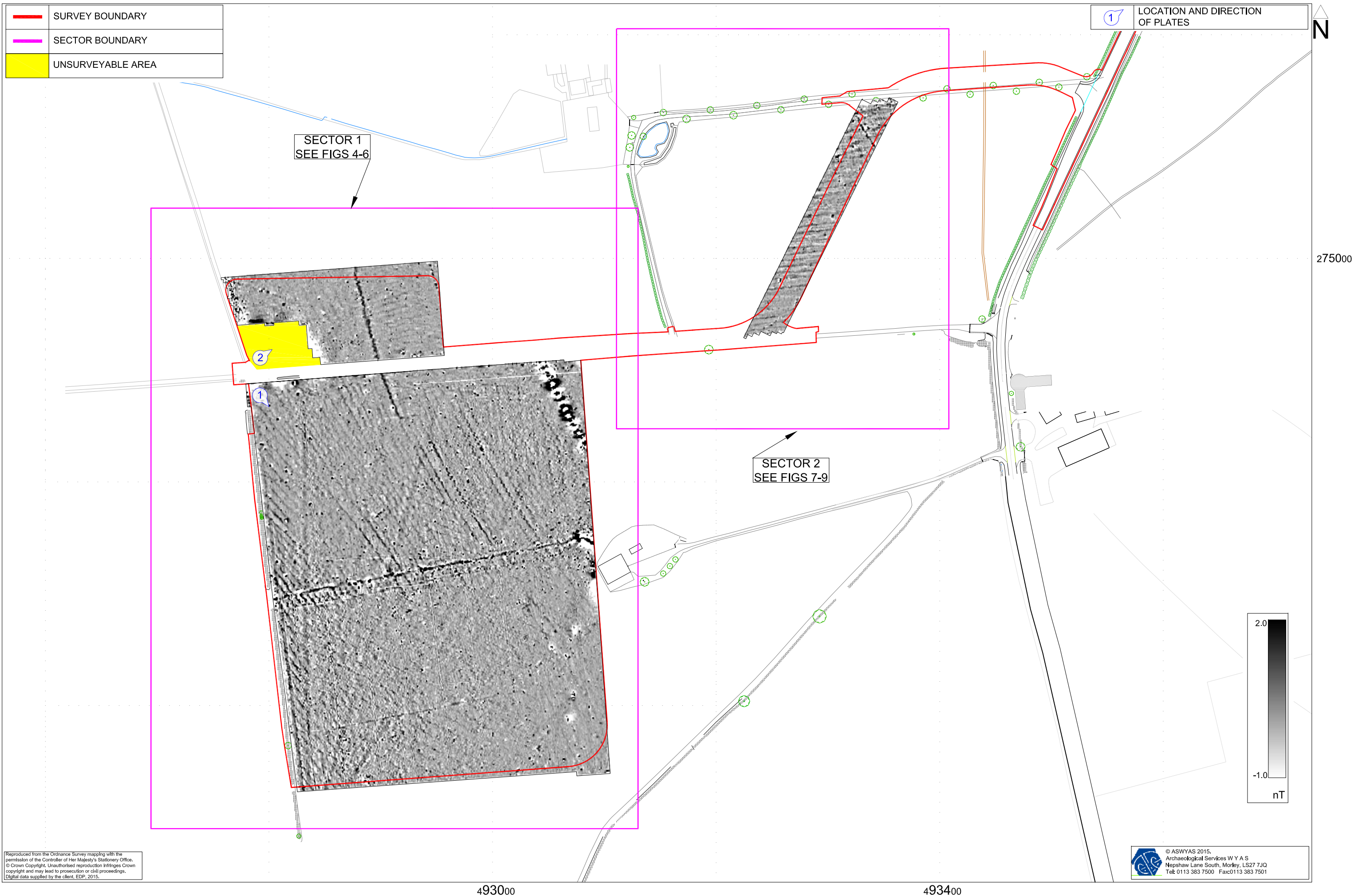
Fig. 2. Survey location showing greyscale magnetometer data (1:3000 @ A3)
