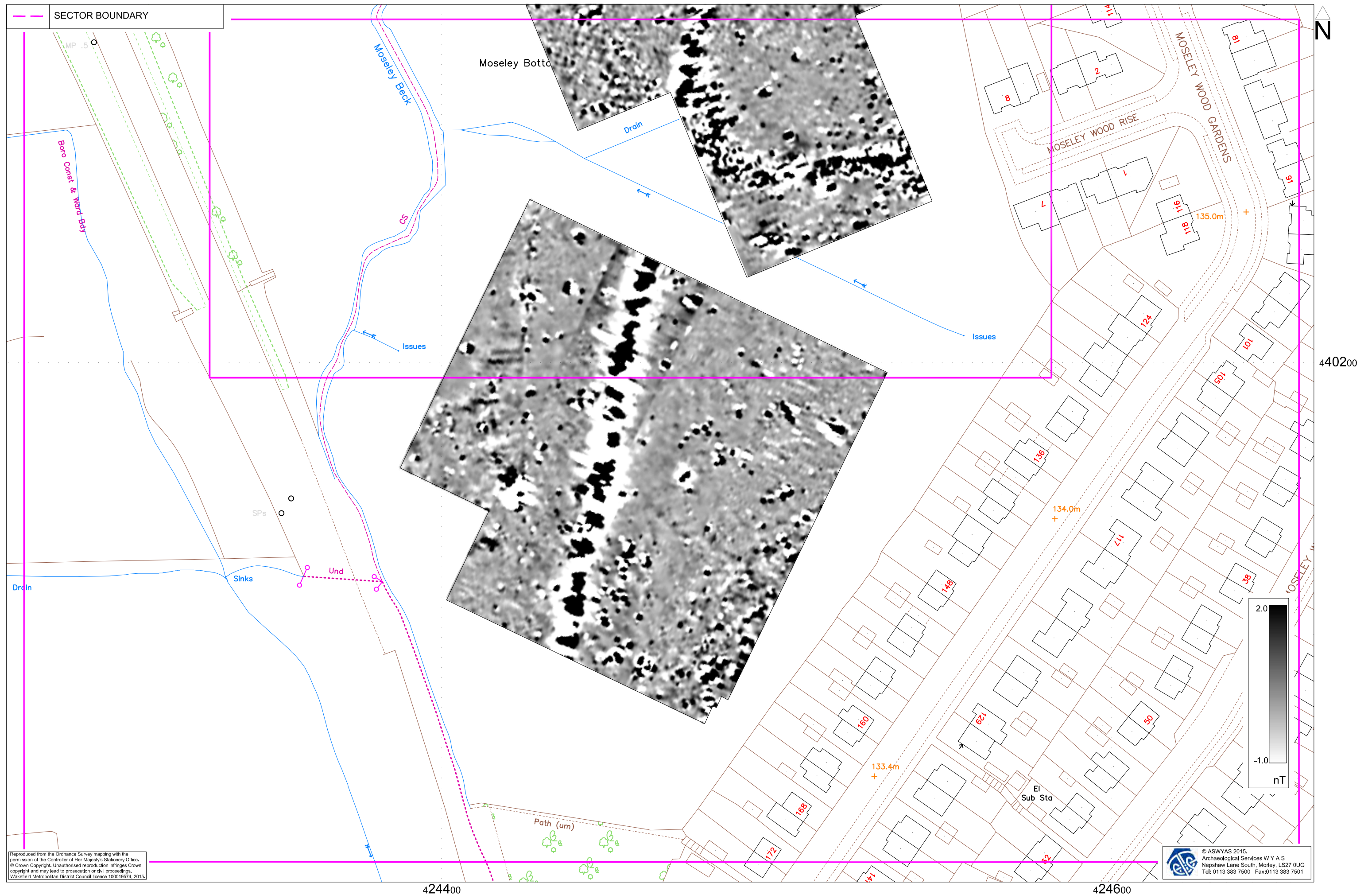
Fig. 4. Processed greyscale magnetometer data; Sector 1 (1:1000 @ A3)
