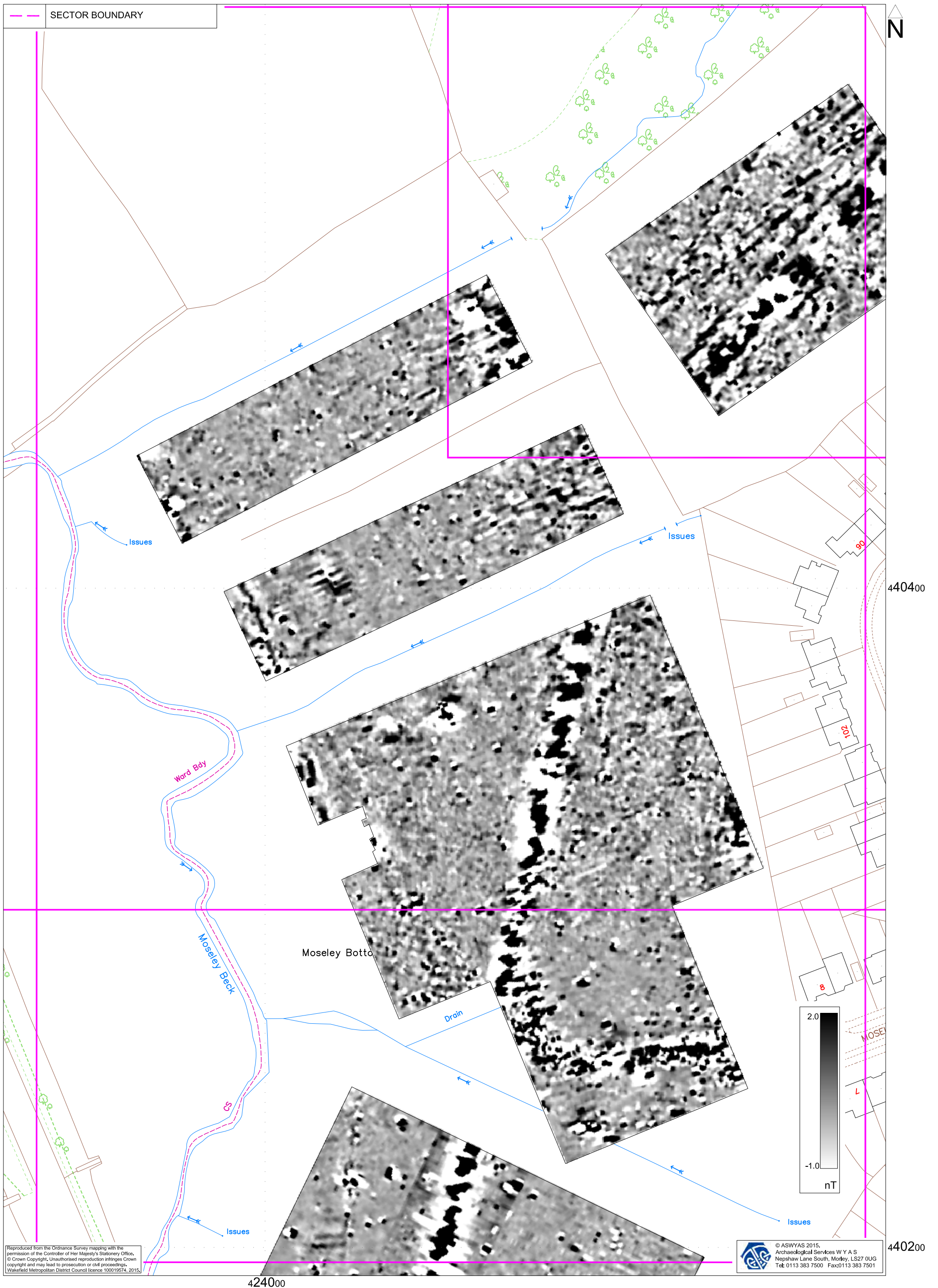
Fig. 7. Processed greyscale magnetometer data; Sector 2 (1:1000 @ A3)
