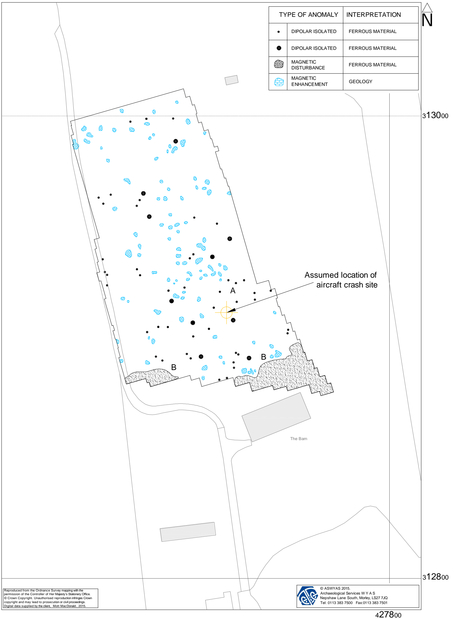
Fig. 5. Interpretation of processed greyscale magnetometer data (1:1000 @ A1)
