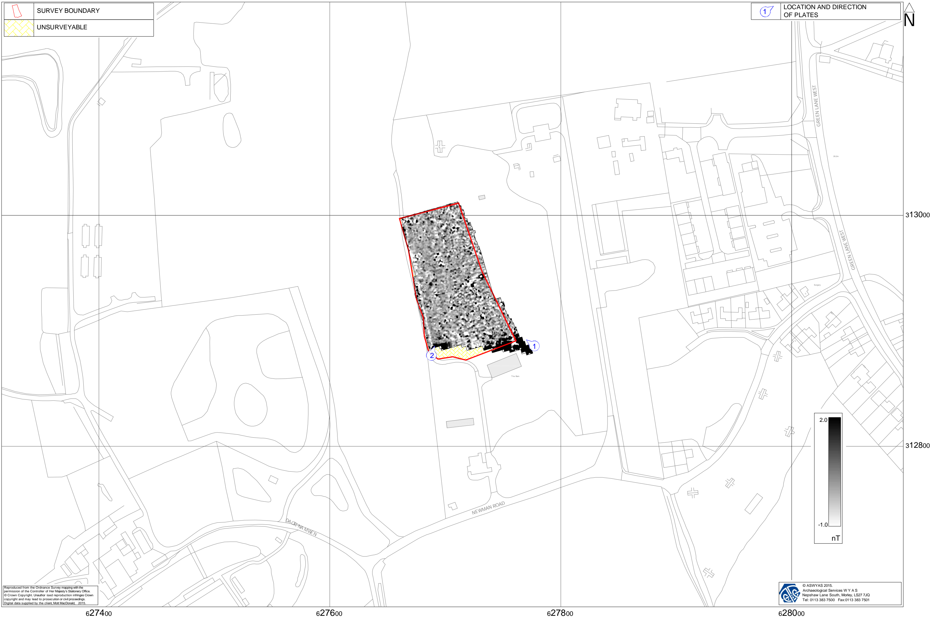
Fig. 2. Survey location showing greyscale magnetometer data (1:2000 @ A3)
