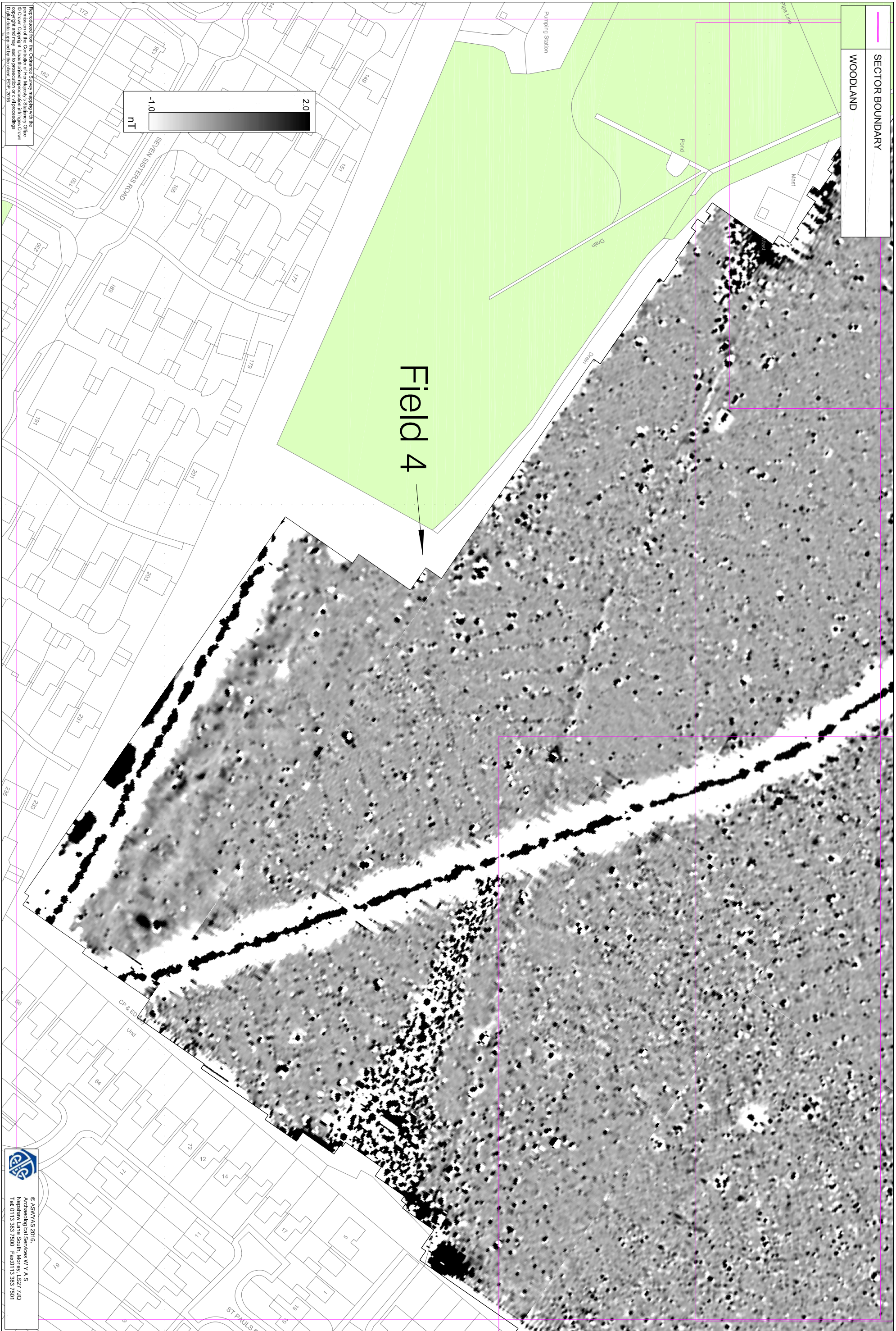
Fig. 13. Processed greyscale plot of magnetometer data; Sector 4 (1:1250 @ A3)
