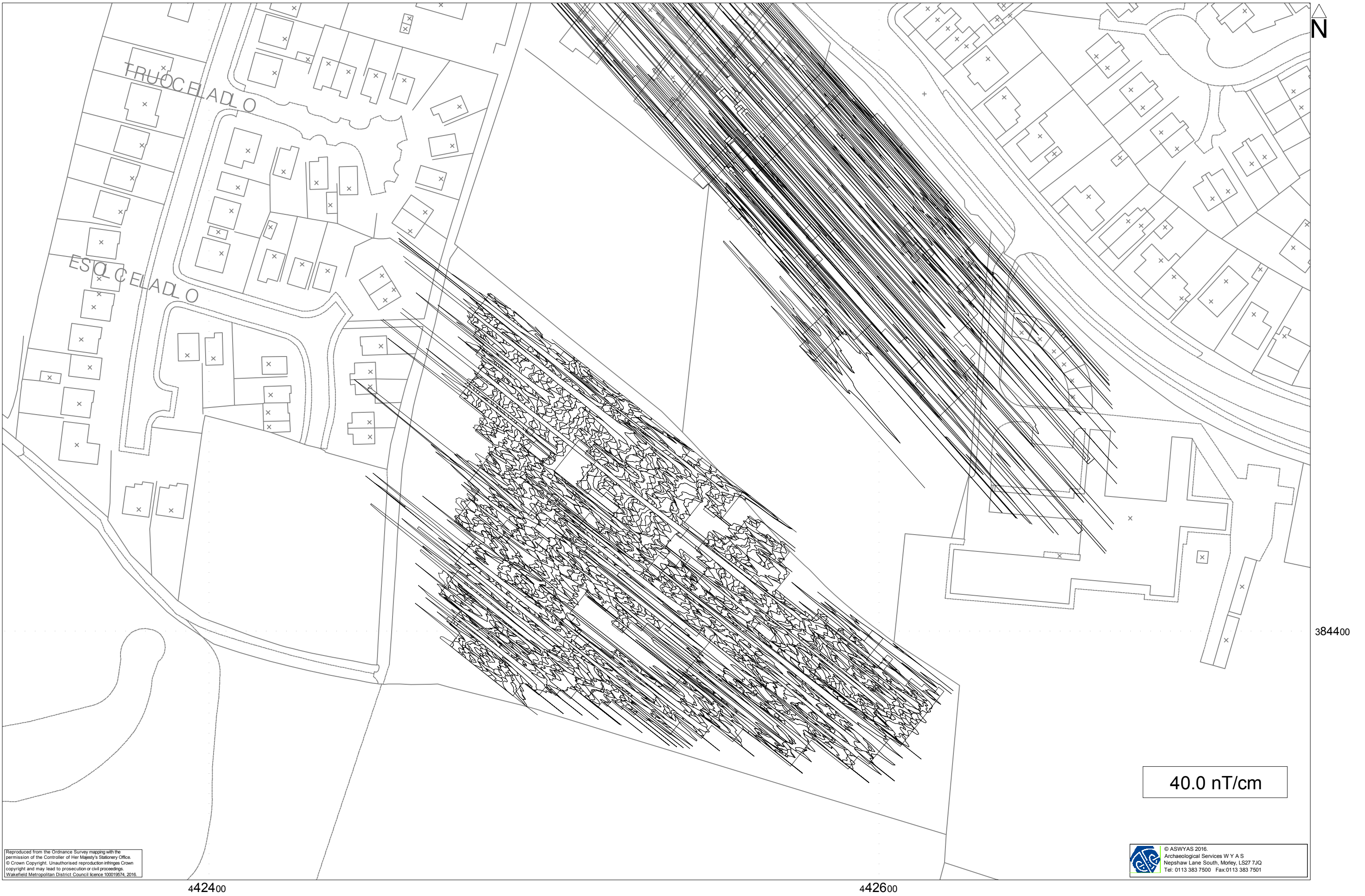
Fig. 4. XY trace plot of magnetometer data (1:1000 @ A3)
