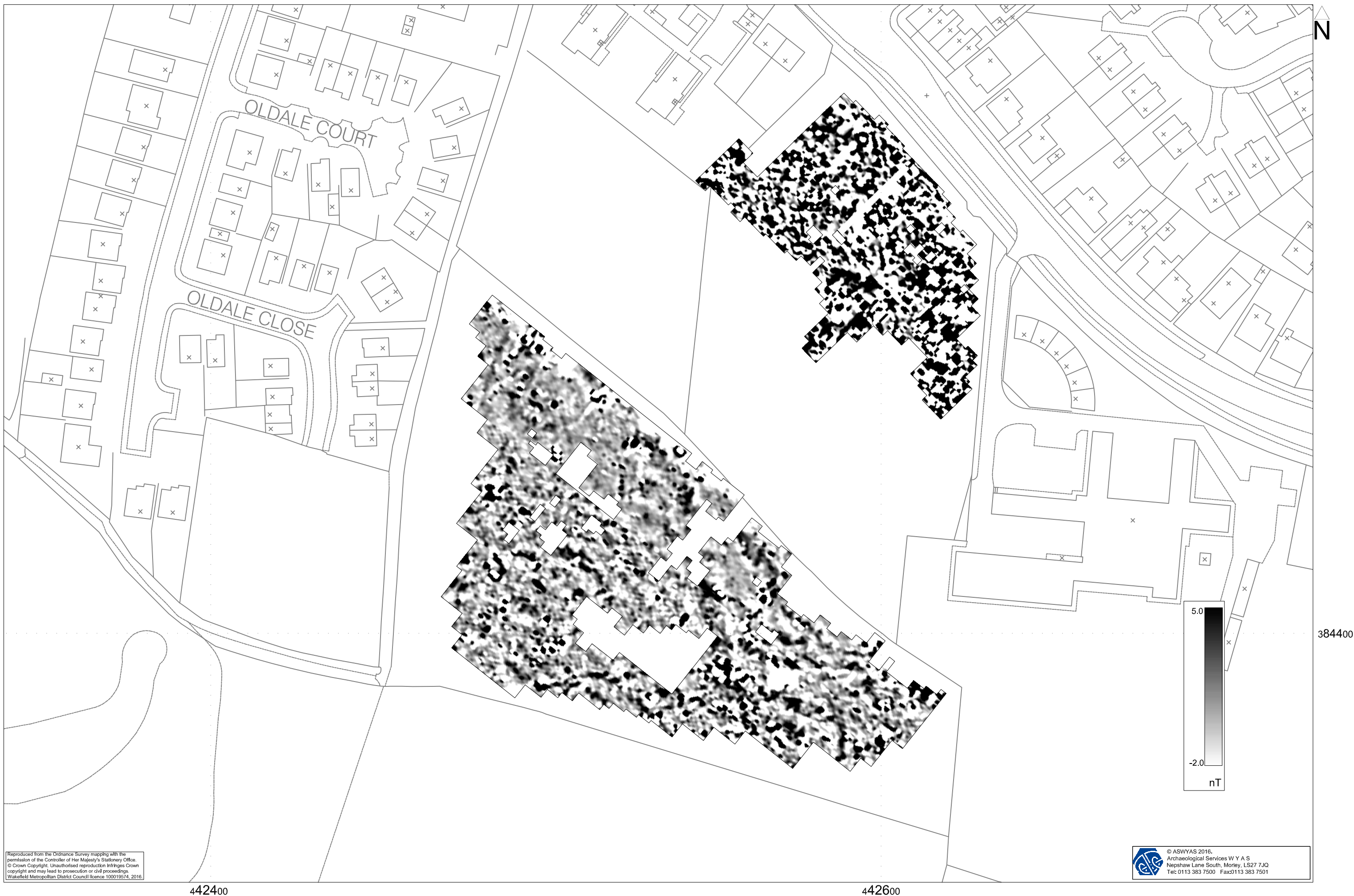
Fig. 3. Greyscale plot of magnetometer data (1:1000 @ A3)
