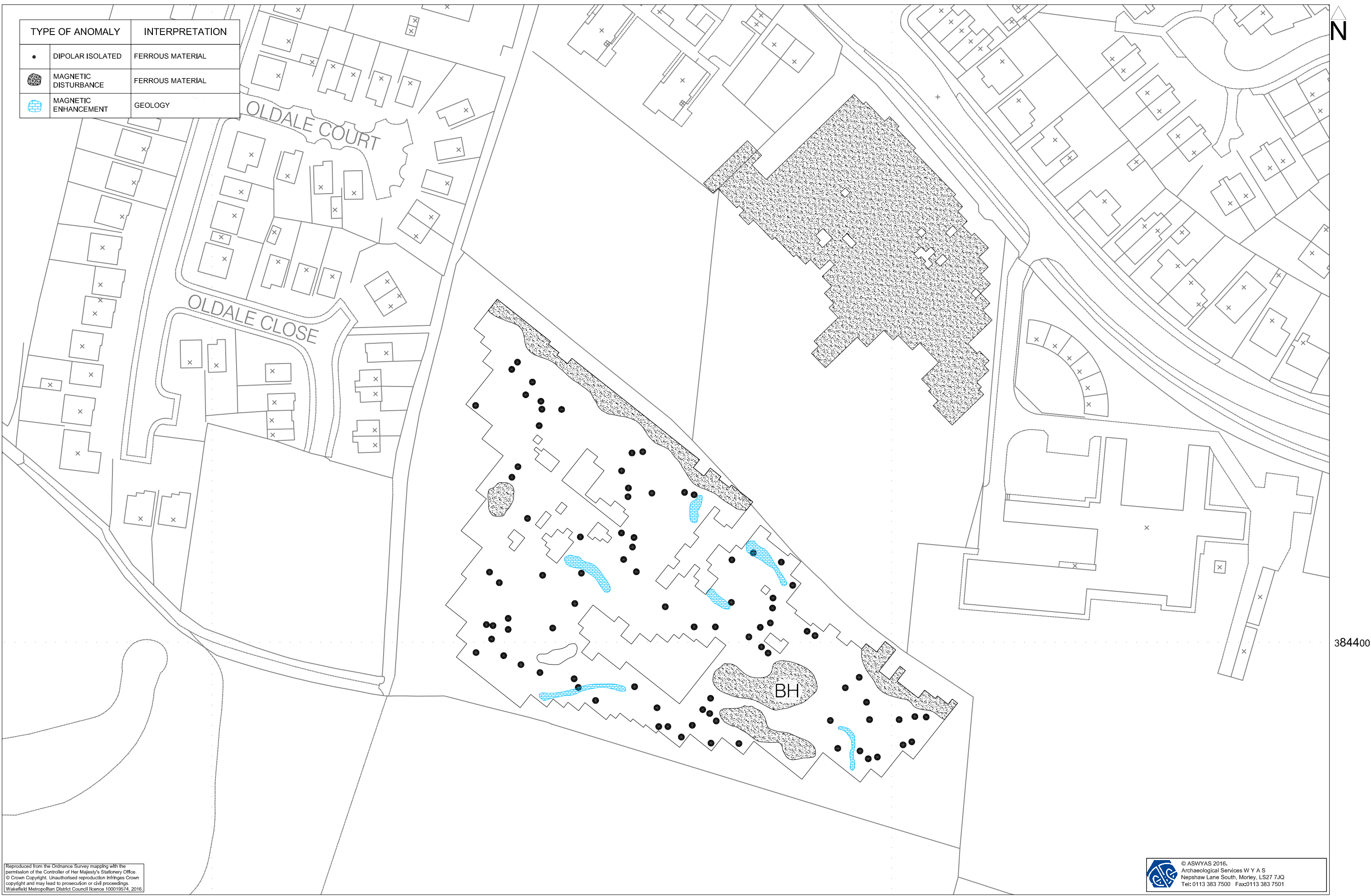
Fig. 5. Interpretation of magnetometer data (1:1000 @ A3)
