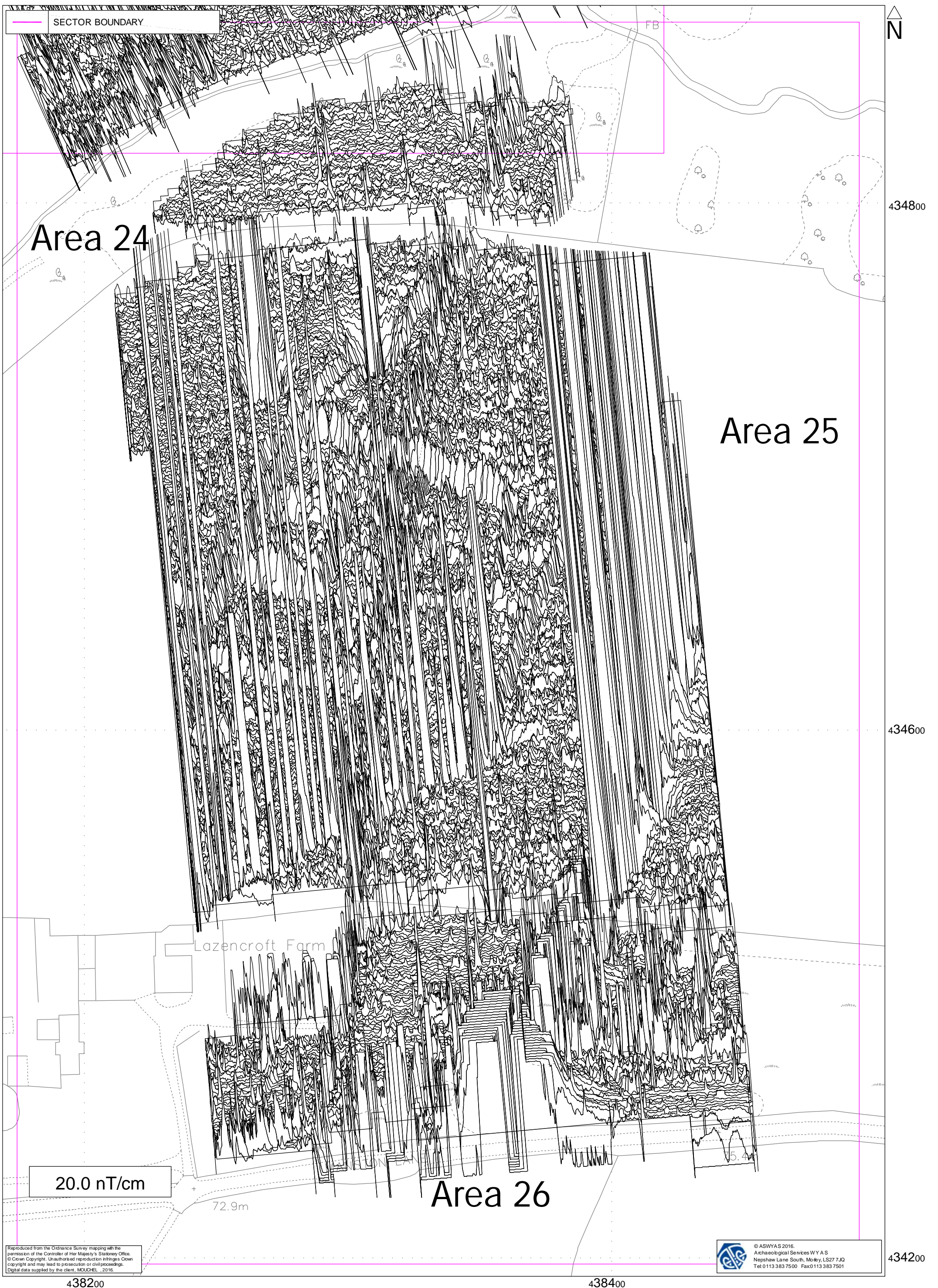
Fig. 47. XY trace plot of minimally processed greyscale magnetometer data; Sector 14 (1:1250 @ A3)
