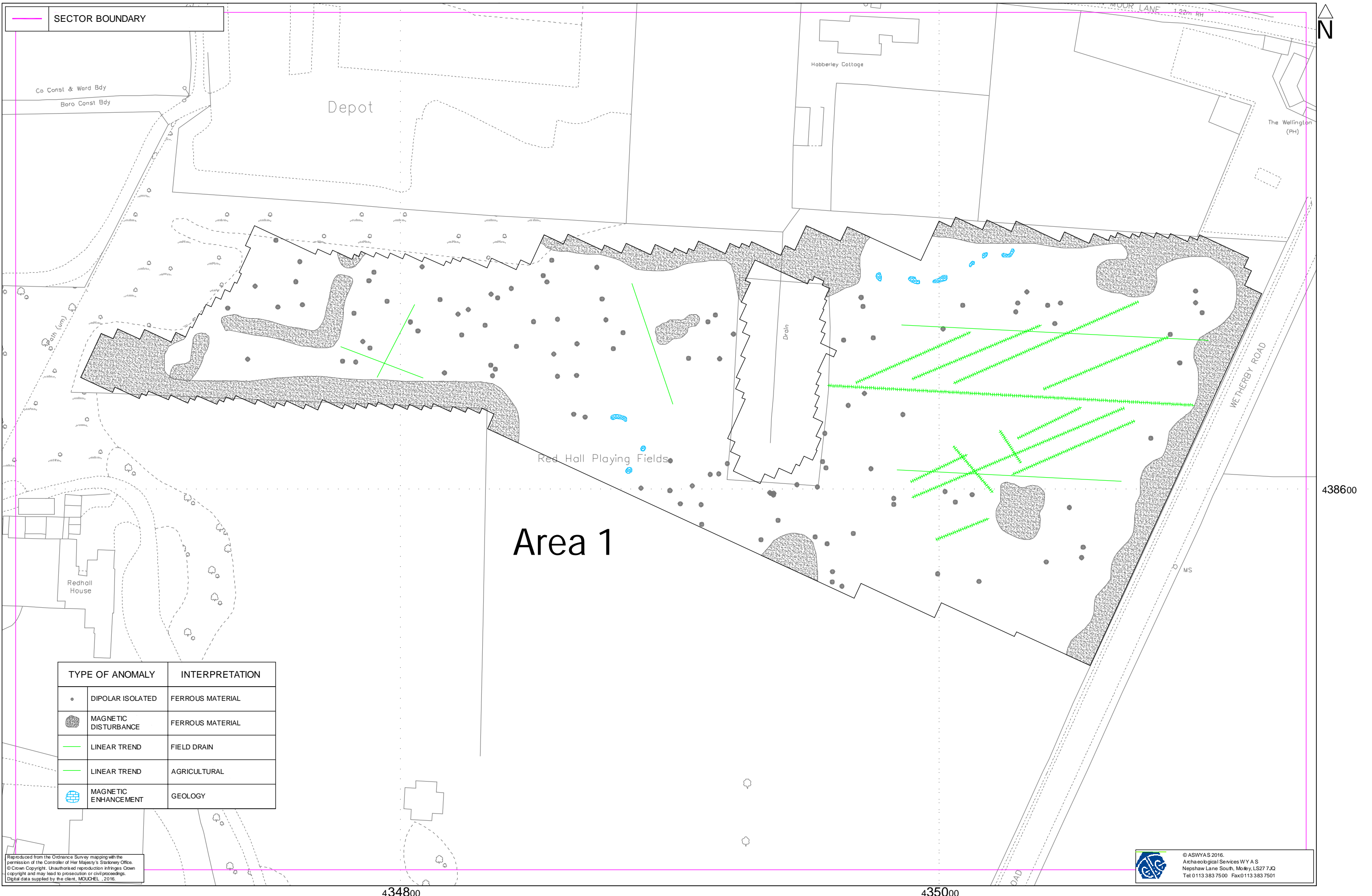
Fig. 9. Interpretation of magnetometer data; Sector 1 (1:1250 @ A3)
