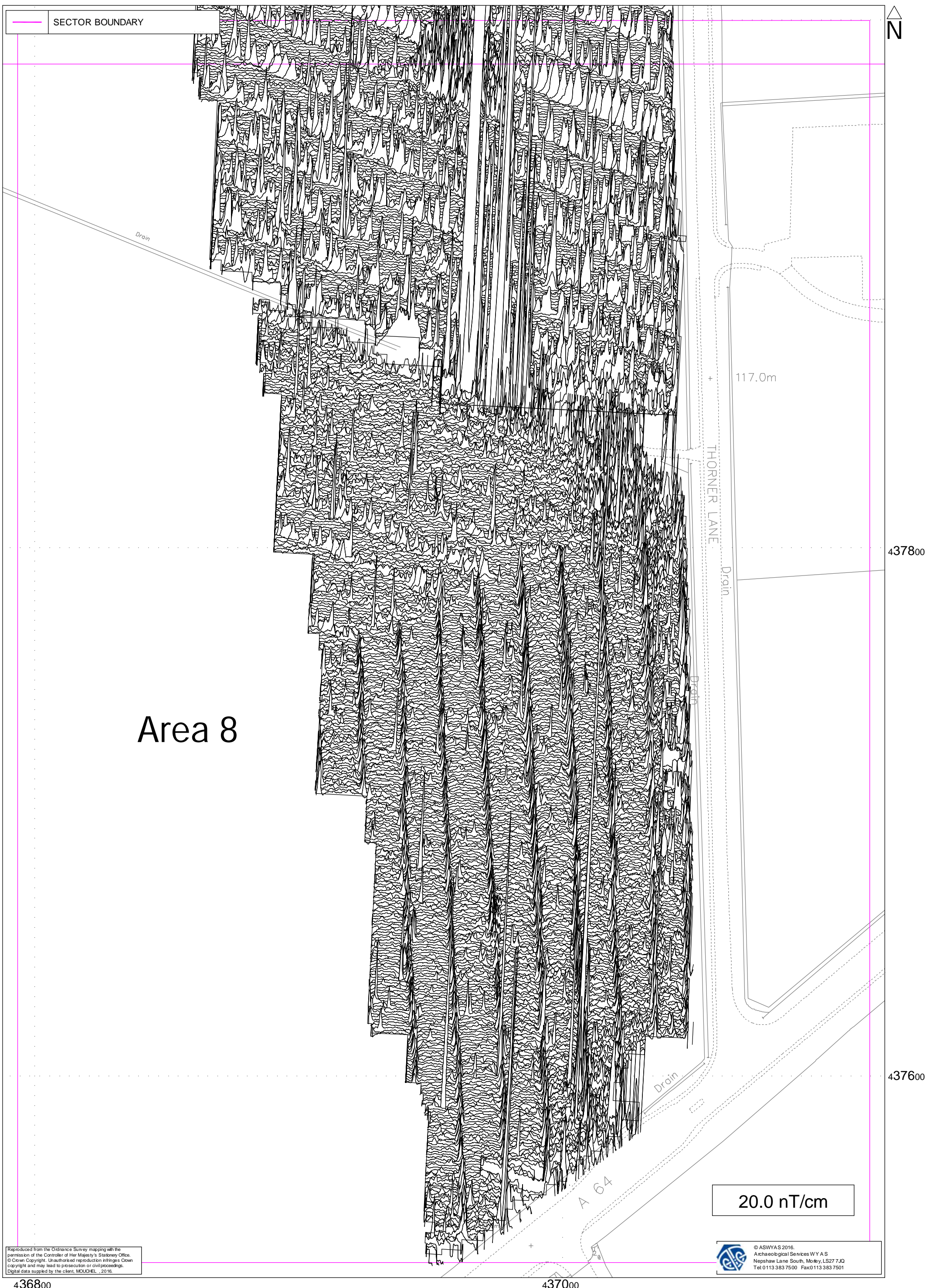
Fig. 17. XY trace plot of minimally processed greyscale magnetometer data; Sector 4 (1:1250 @ A3)
