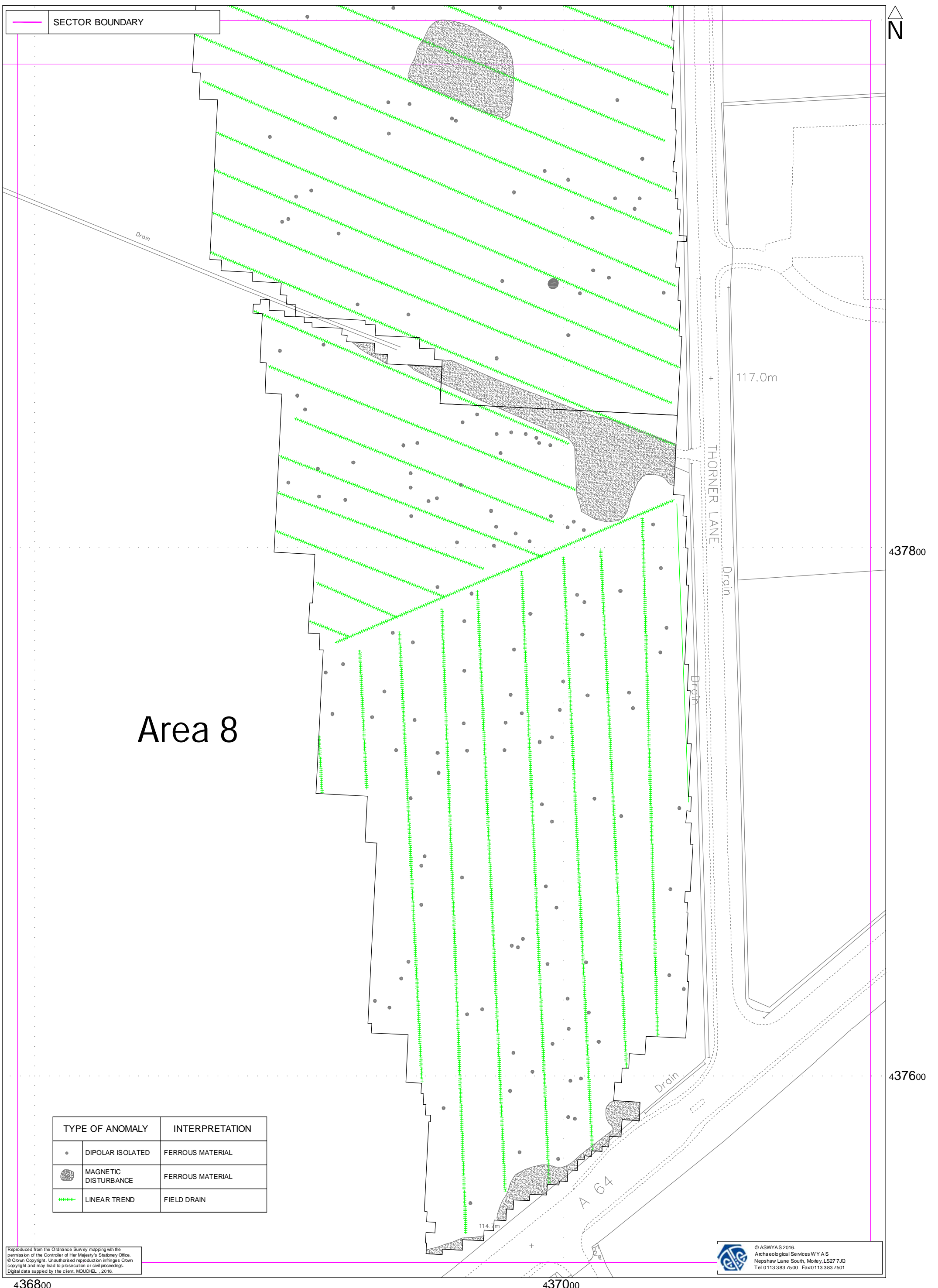
Fig. 18. Interpretation of greyscale magnetometer data; Sector 4 (1:1250 @ A3)
