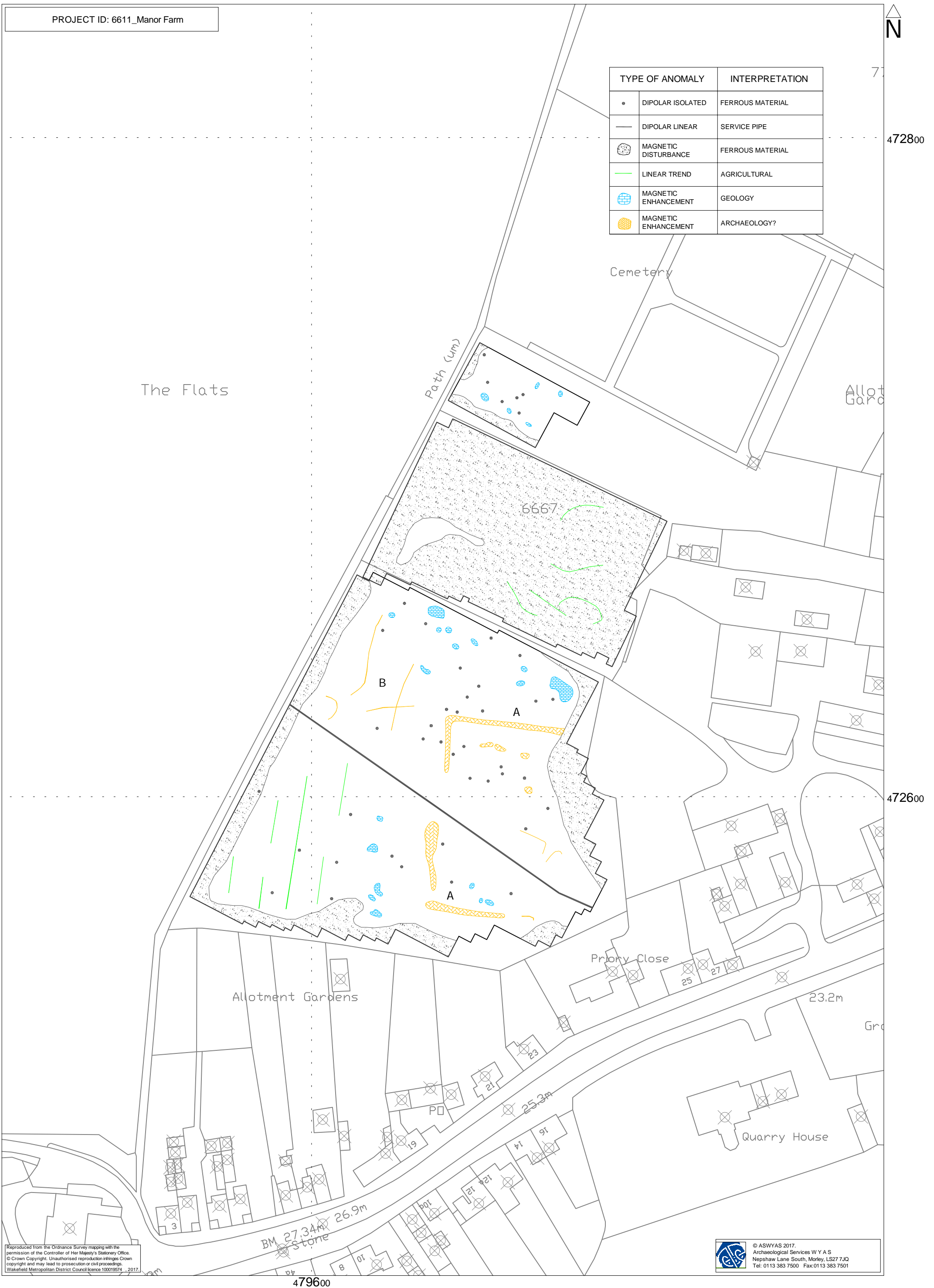
Fig. 5. Interpretation of magnetometer data (1:1000 @ A3)
