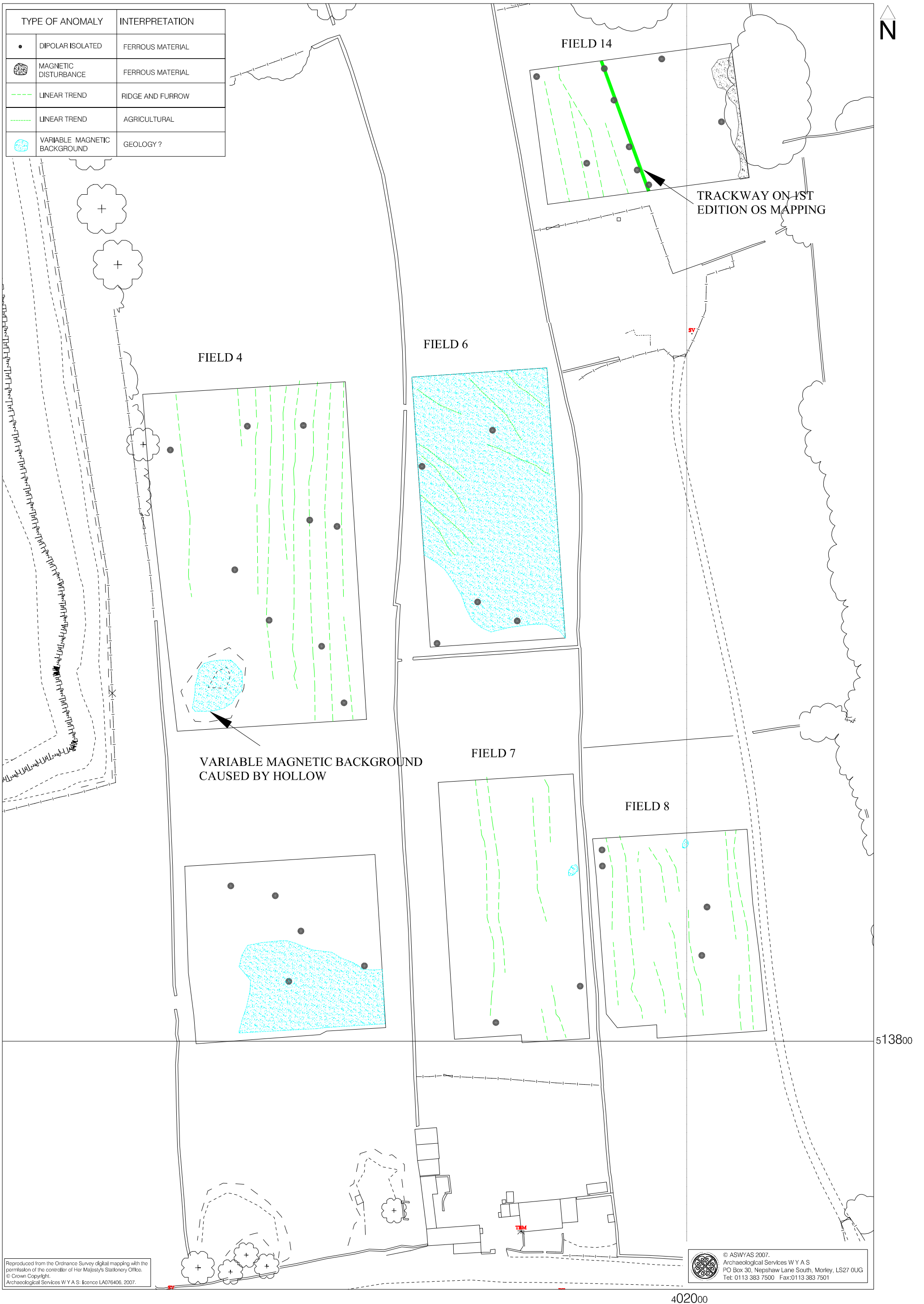
Fig. 5. Interpretation of magnetometer data: Fields 4, 6, 7, 8 and 14 (1:1000 @ A3)
