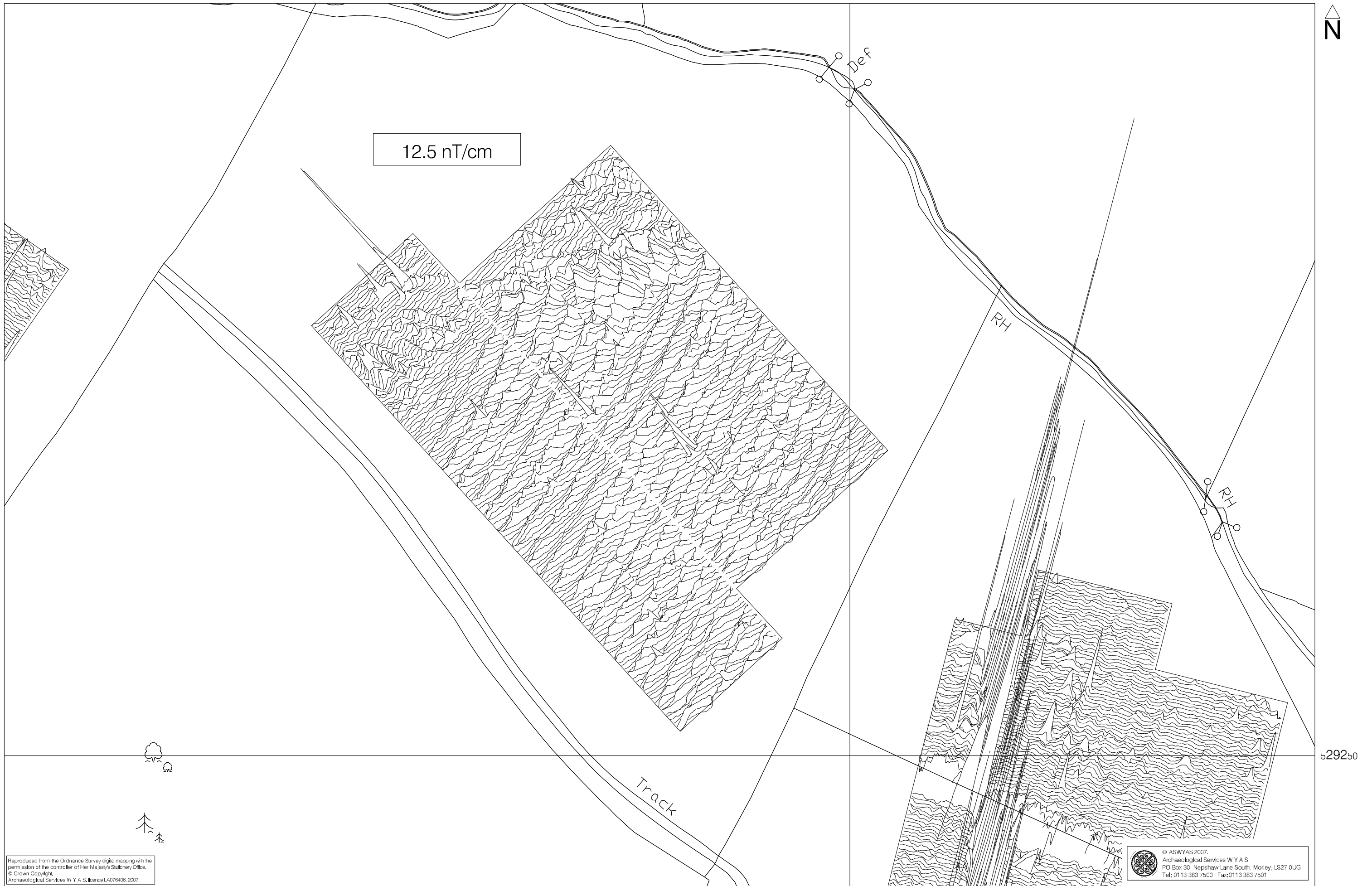
Fig. 7. XY trace plot of unprocessed magnetometer data; Area B (1:1000 @ A3)
