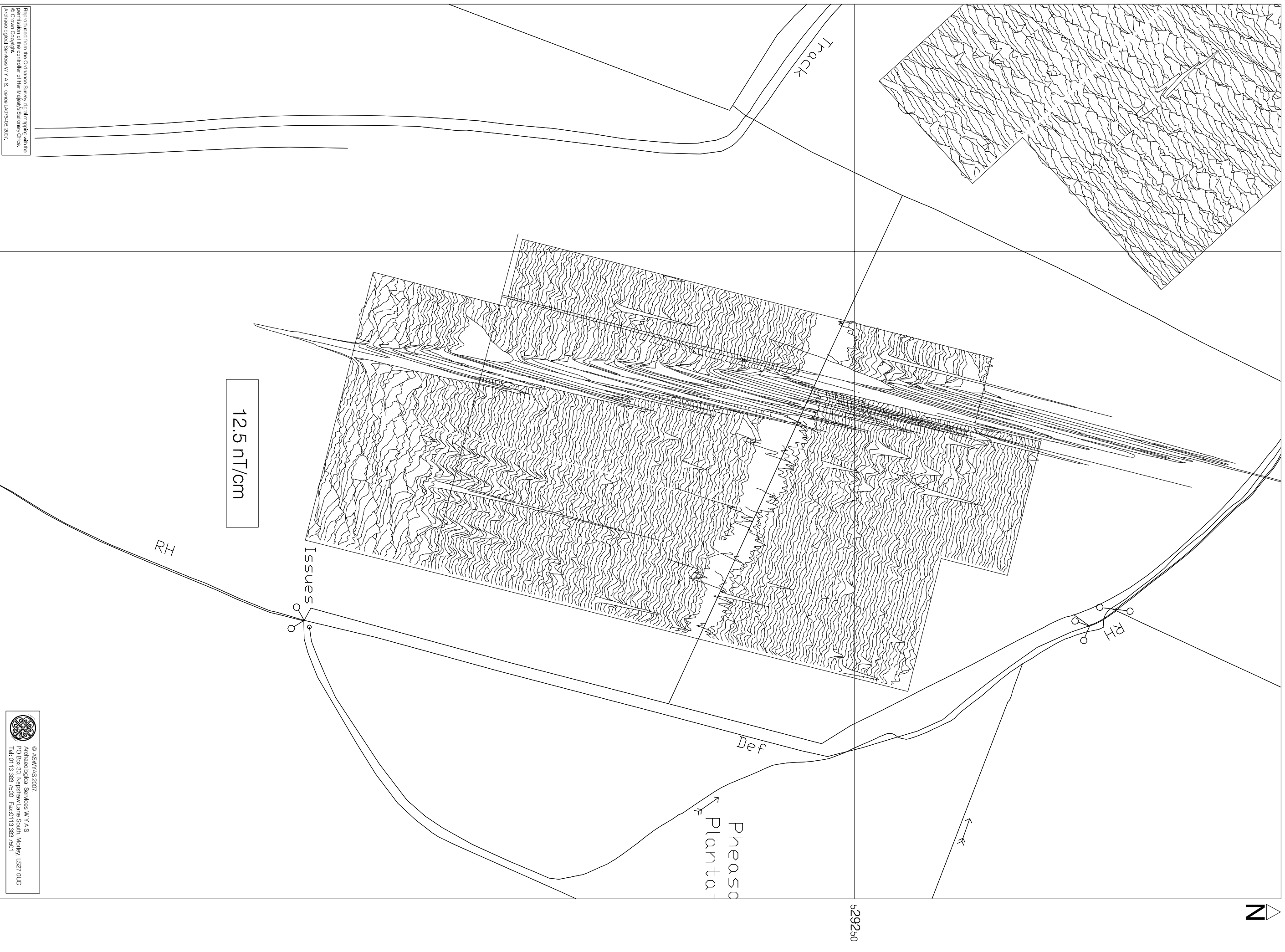
Fig. 10. XY trace plot of unprocessed magnetometer data. Area C (1:1000 @ A3)
