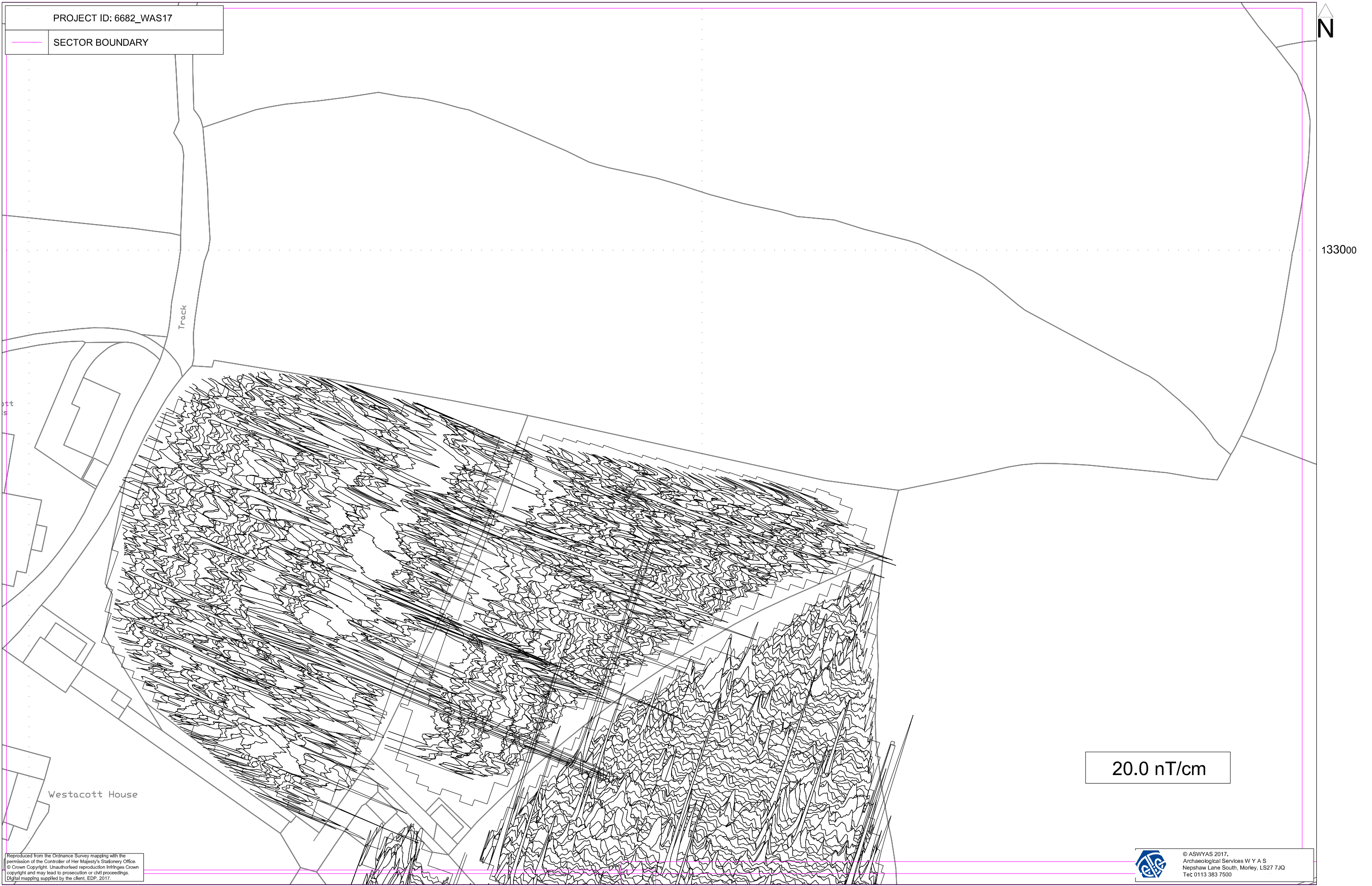
Fig. 5. XY trace plot of minimally processed magnetometer data; Sector 1 (1:1000 @ A3)
