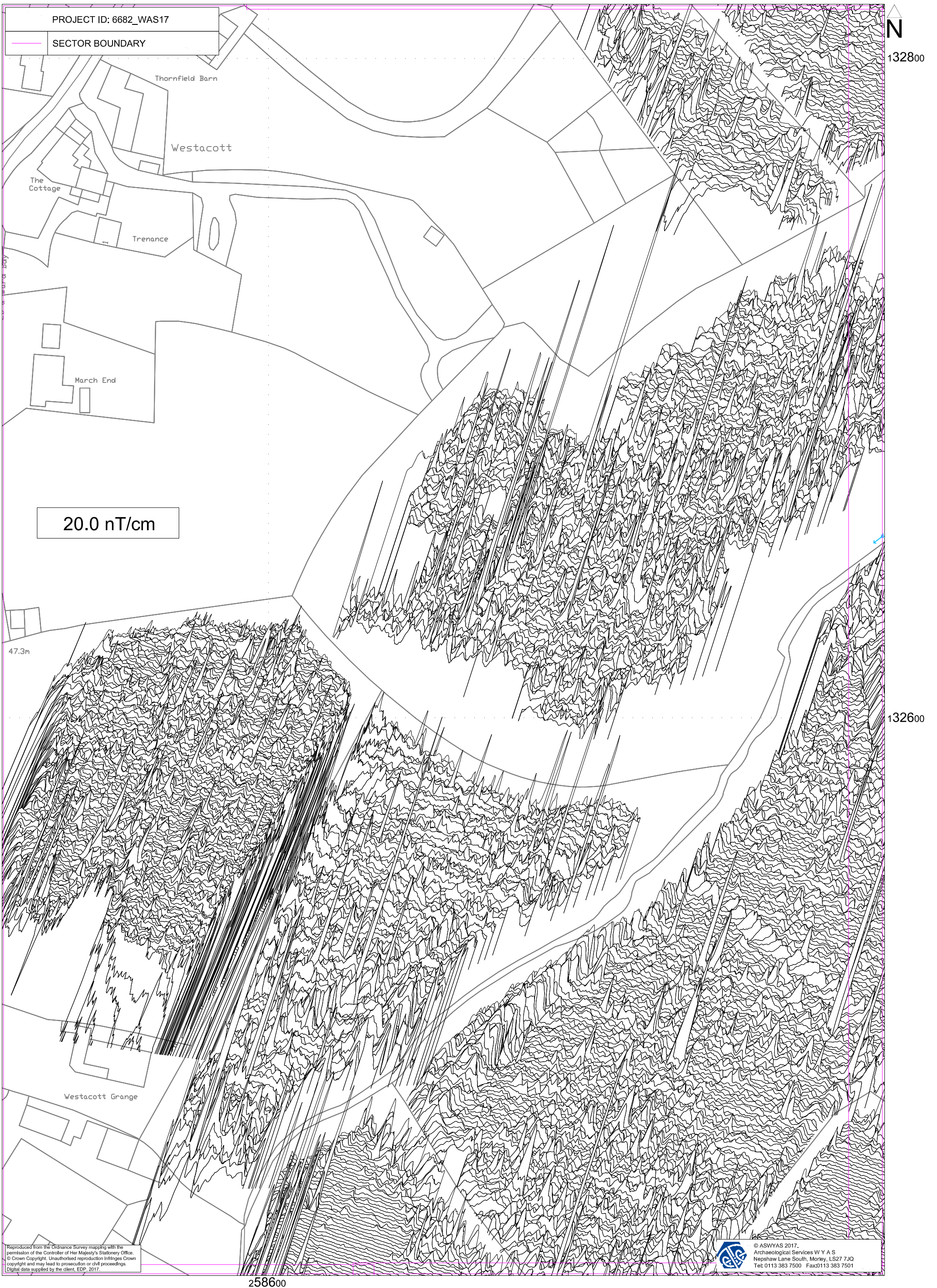
Fig. 8. XY trace plot of minimally processed magnetometer data; Sector 2 (1:1000 @ A3)
