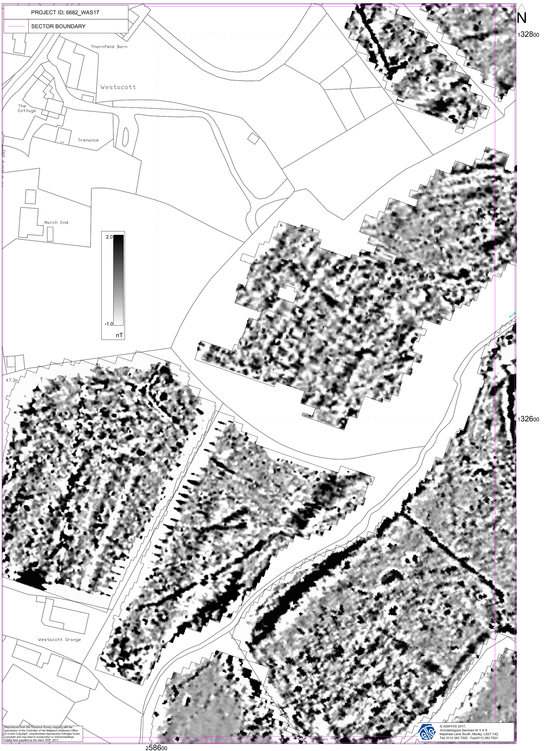
Fig. 7. Processed greyscale magnetometer data; Sector 2 (1:1000 @ A3)
