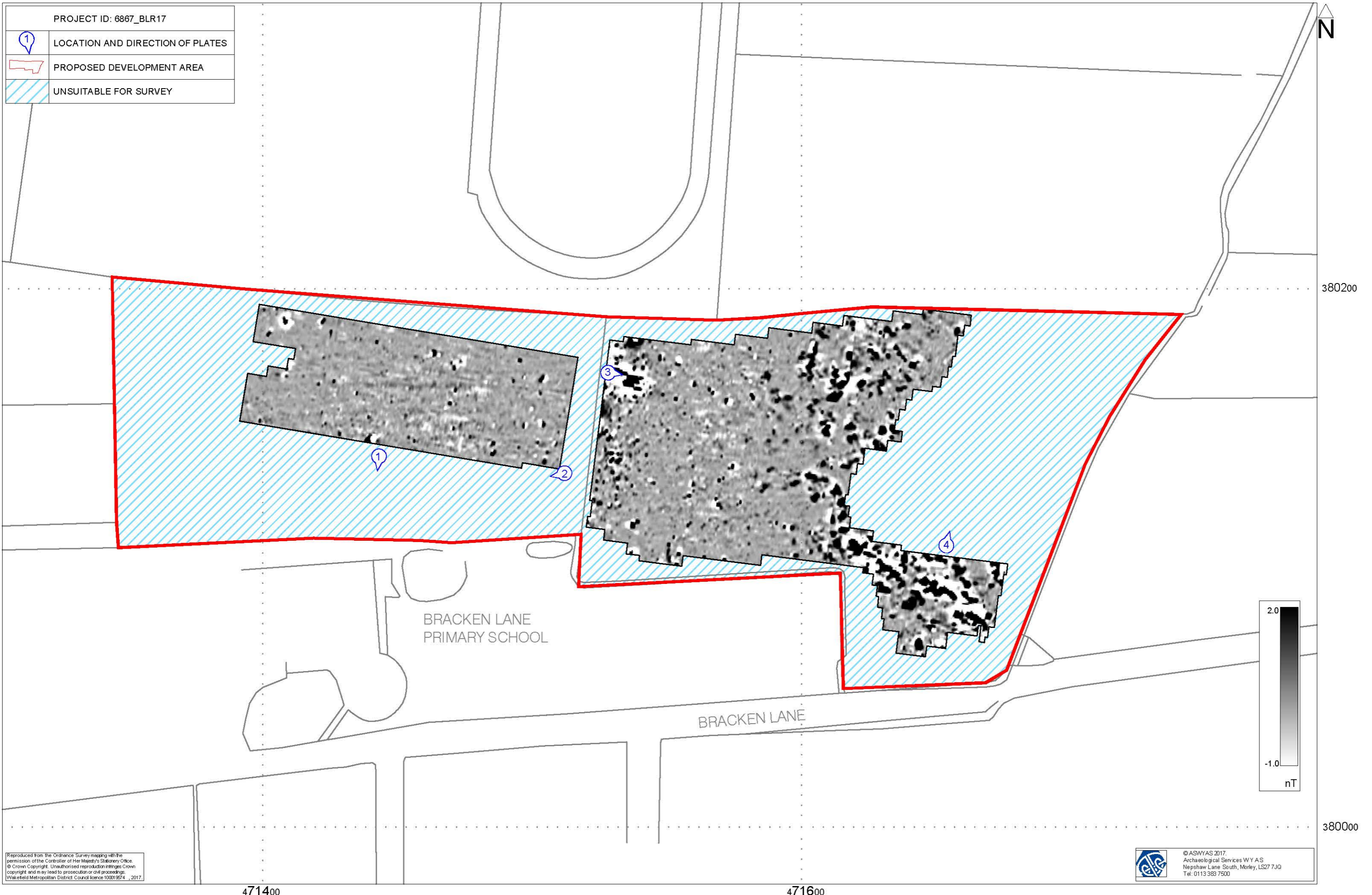
Fig. 2. Survey location showing processed magnetometer data (1:1250 @ A3)
