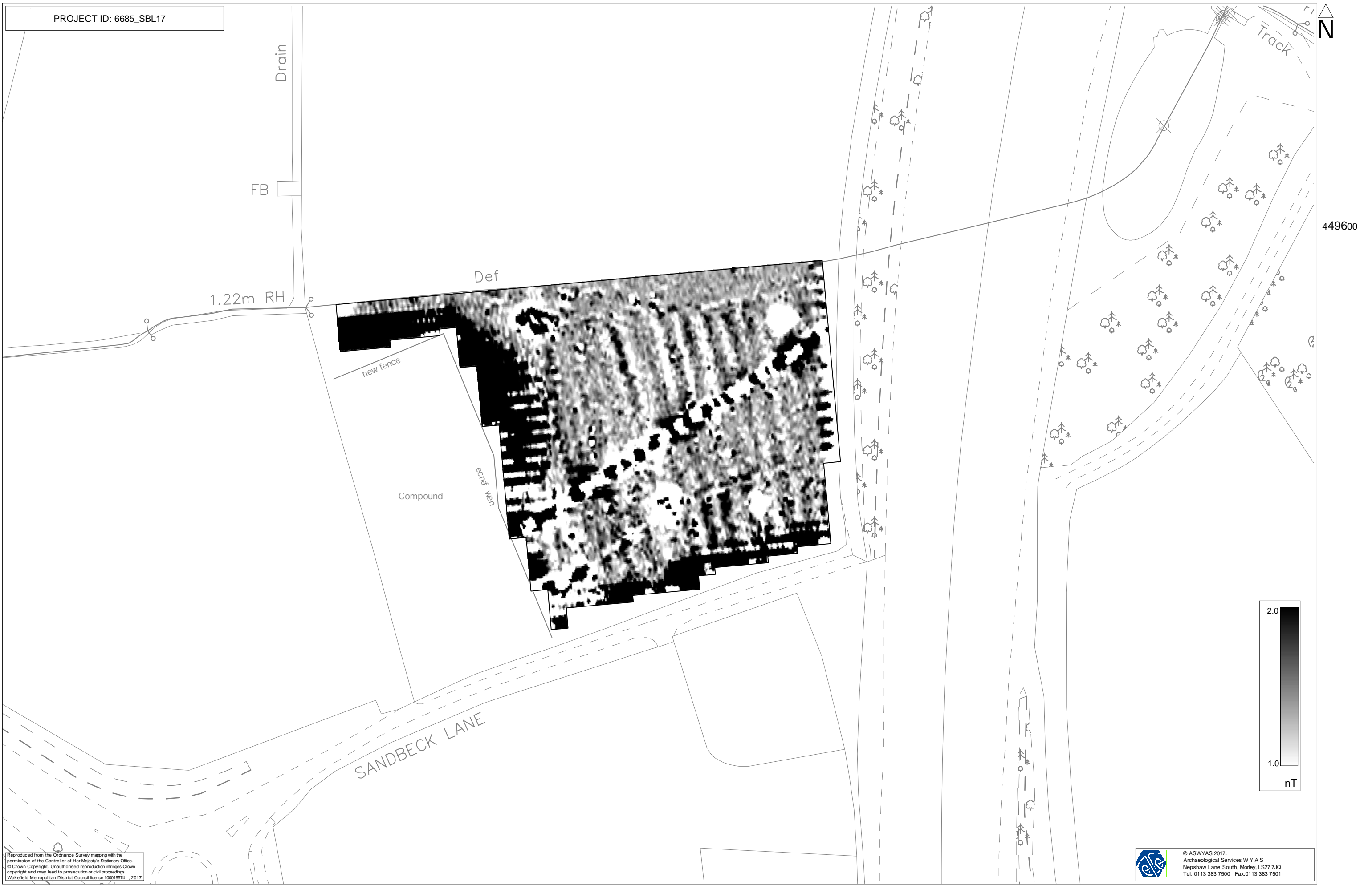
Fig. 3. Processed greyscale magnetometer data (1:1000 @ A3)
