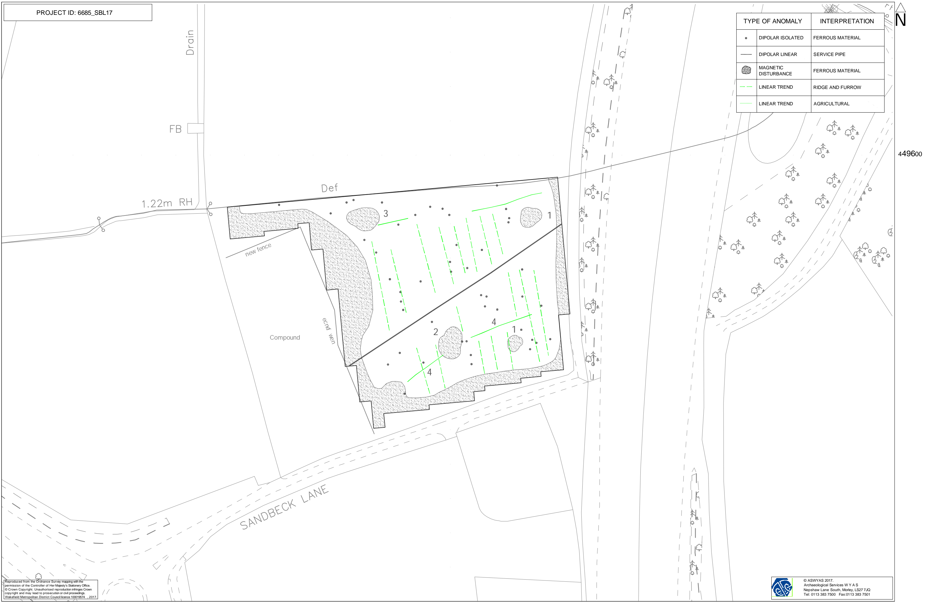
Fig. 5. Interpretation of magnetometer data (1:1000 @ A3)
