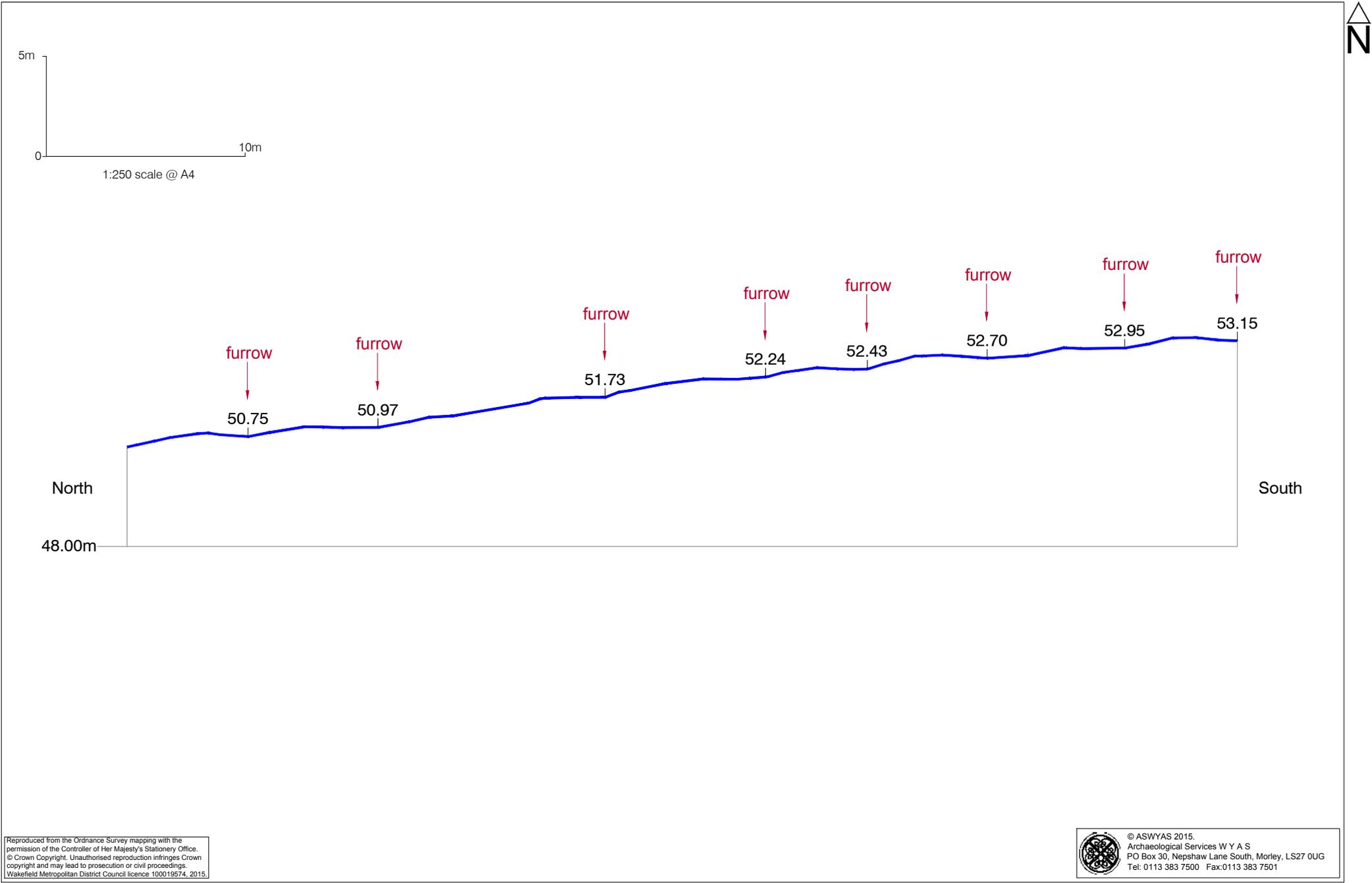
Fig. 10. Profile over ridge and furrow earthworks (1:250 @ A4)
