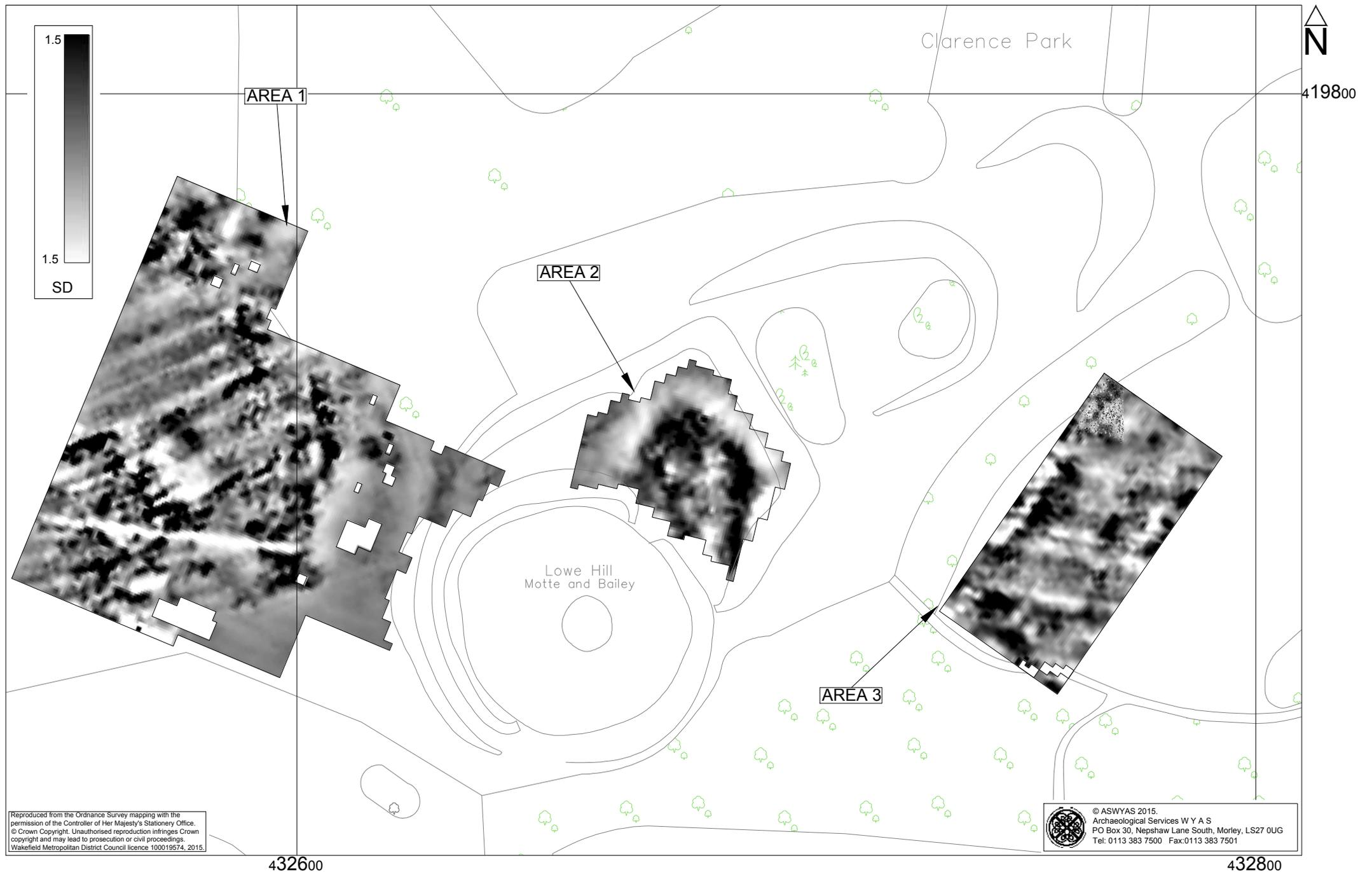
Fig. 6. Processed greyscale earth resistance data (1:1000 @ A4)
