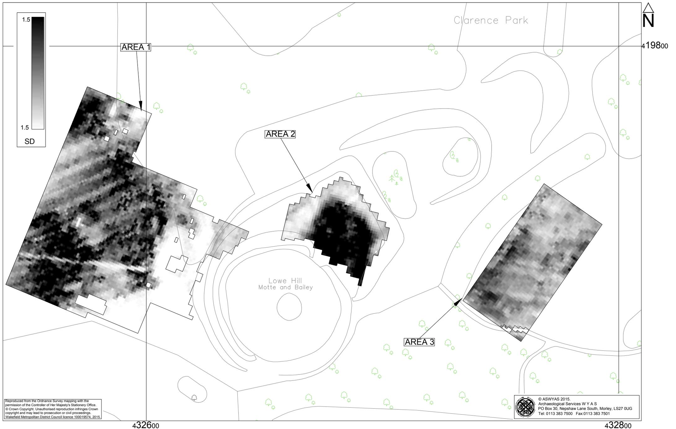
Fig. 7. Unprocessed greyscale earth resistance data (1:1000 @ A4)
