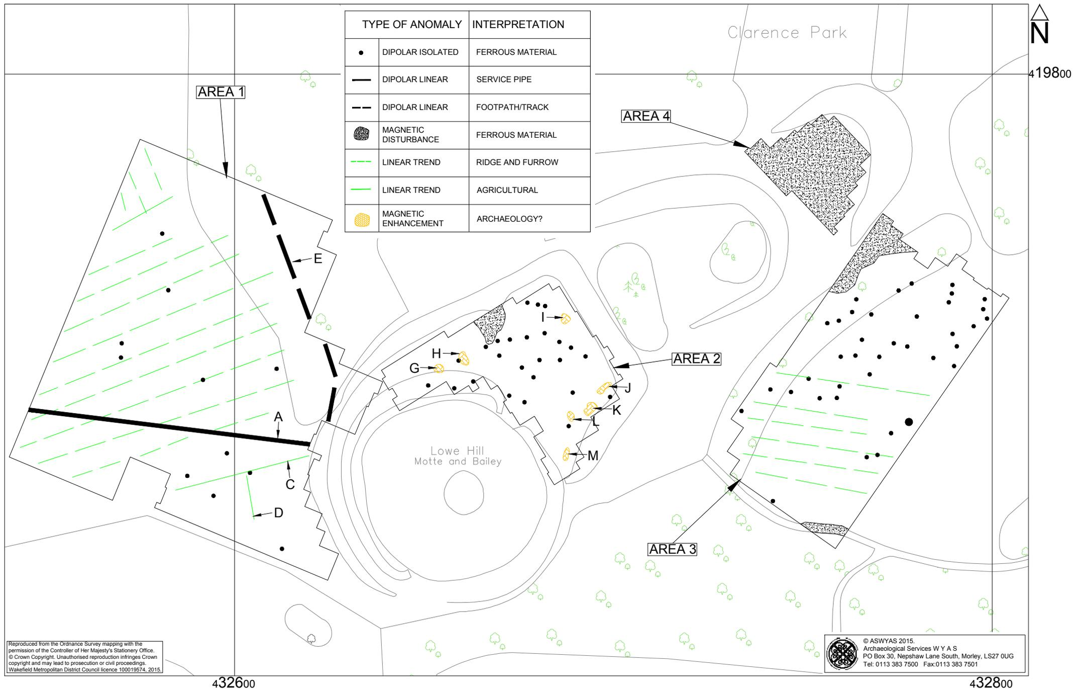
Fig. 5. Interpretation of magnetometer data (1:1000 @ A4)
