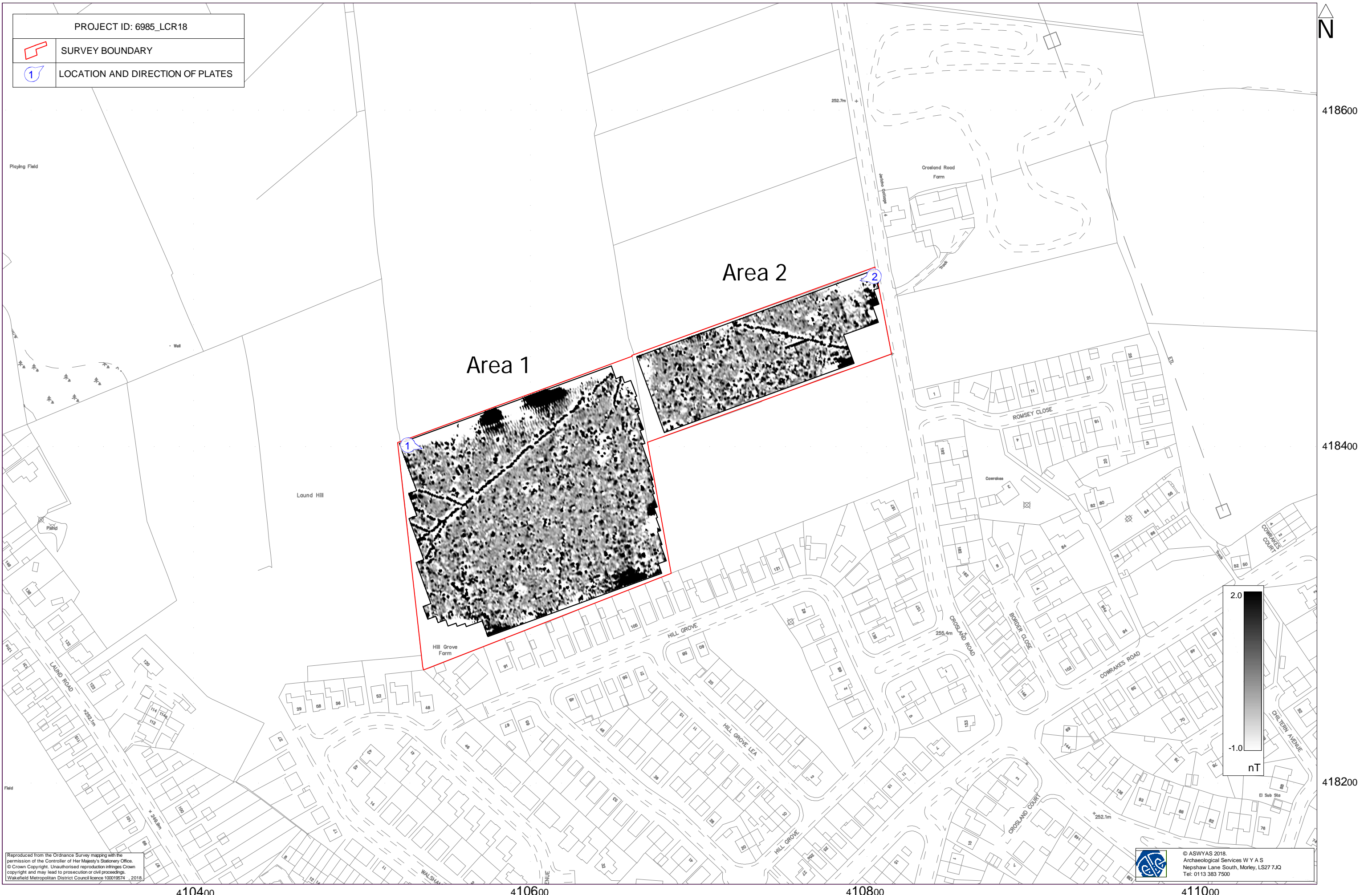
Fig. 2. Survey location showing greyscale gradiometer data (1:2000 @ A3)
