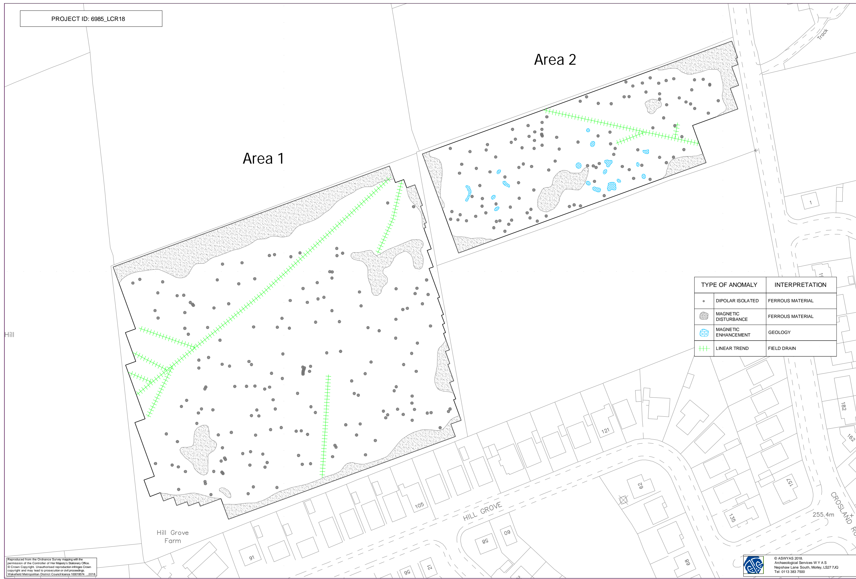
Fig. 5. Interpretation of gradiometer data (1:1000 @ A3)
