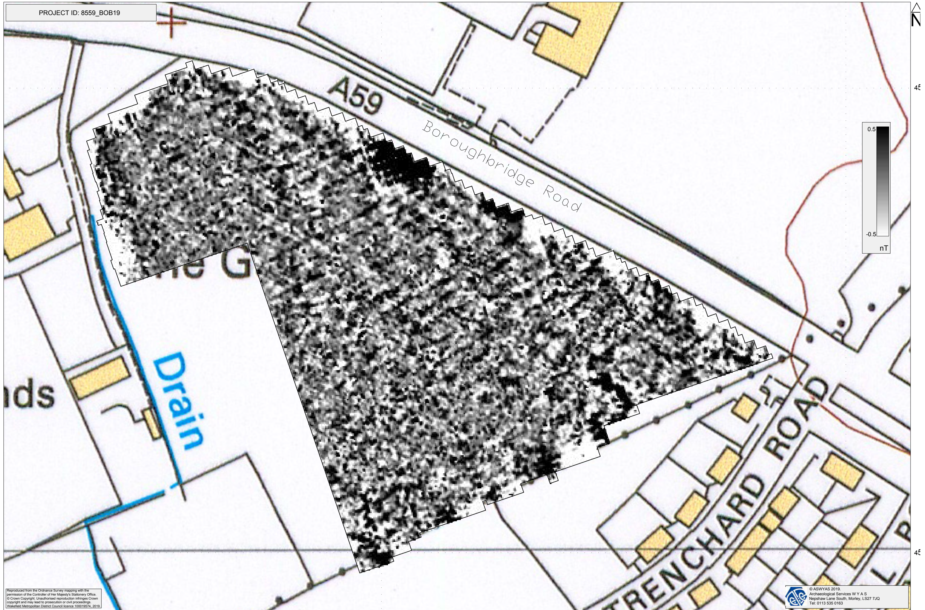
Fig. 6. Processed greyscale of magnetometer data, displayed at a narrow nano-tesla range (1:1000 @ A3)
