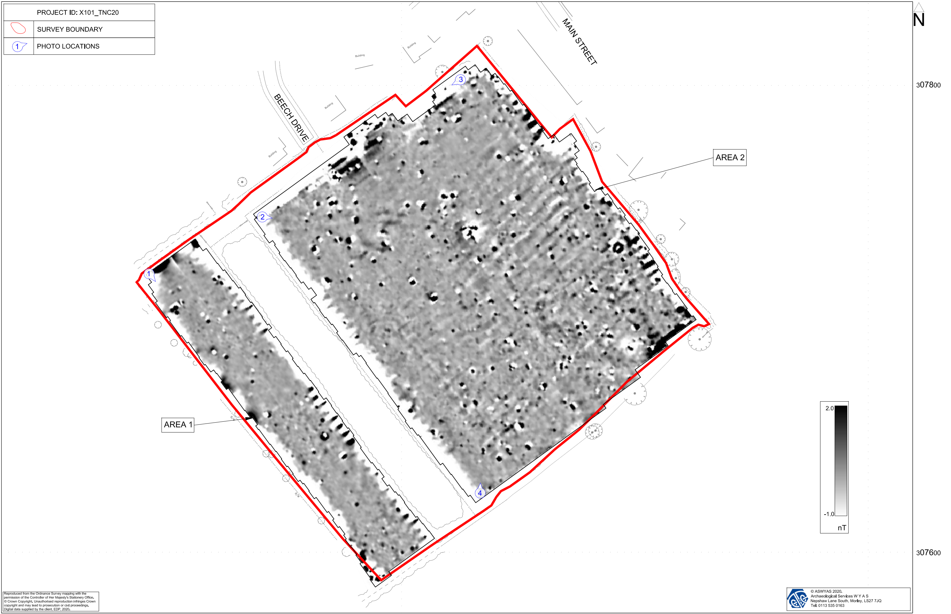
Fig. 2. Survey location showing processed greyscale of magnetometer data and plate locations (1:1000 @ A3)
