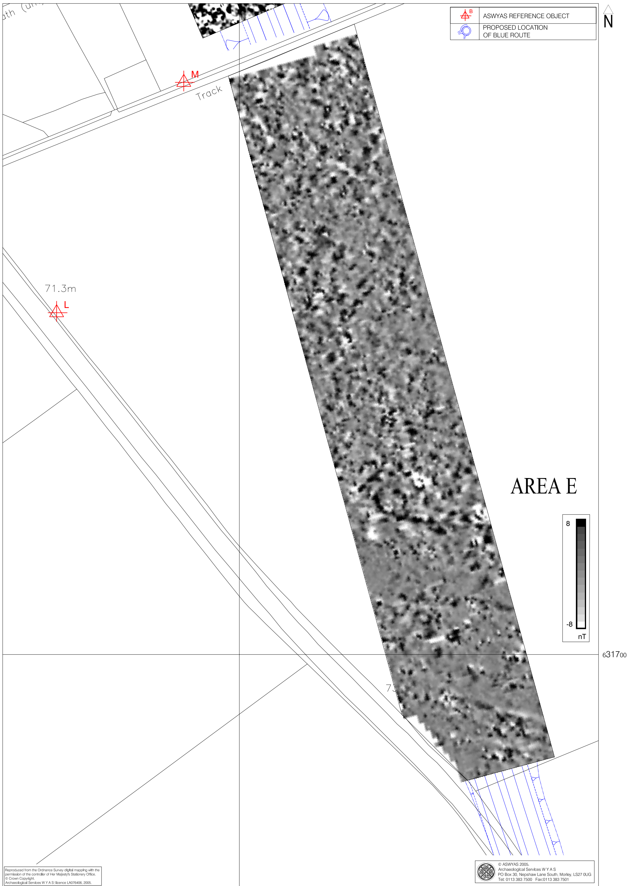
Fig. 12. Plot of greyscale magnetometer data; Area E
