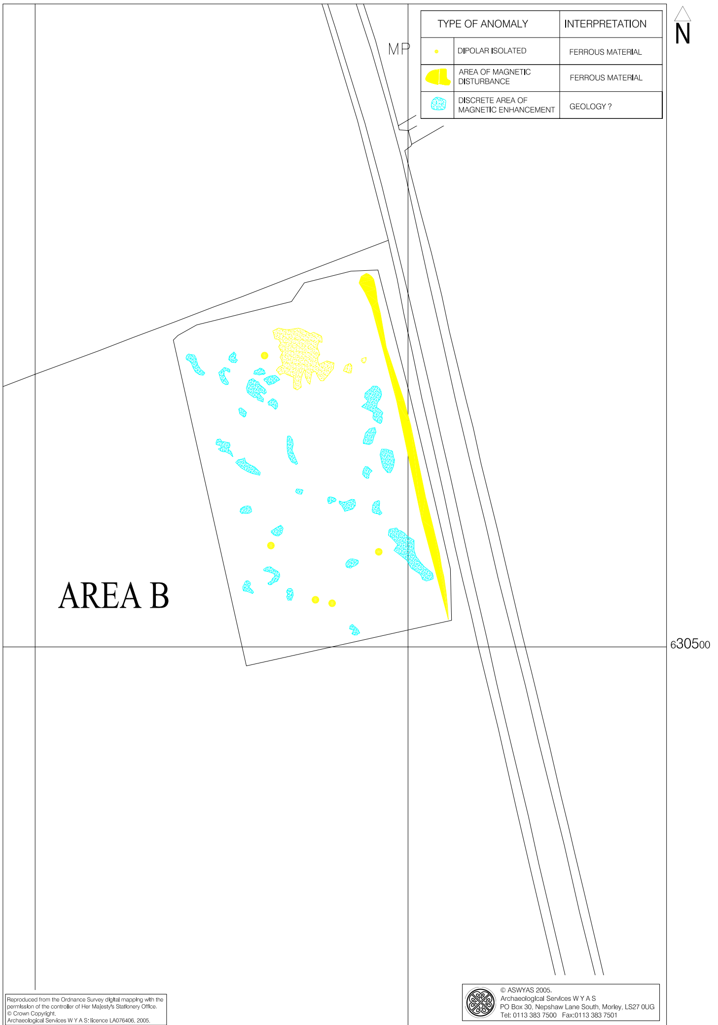
Fig. 7. Interpretation plot of magnetometer data; Area B
