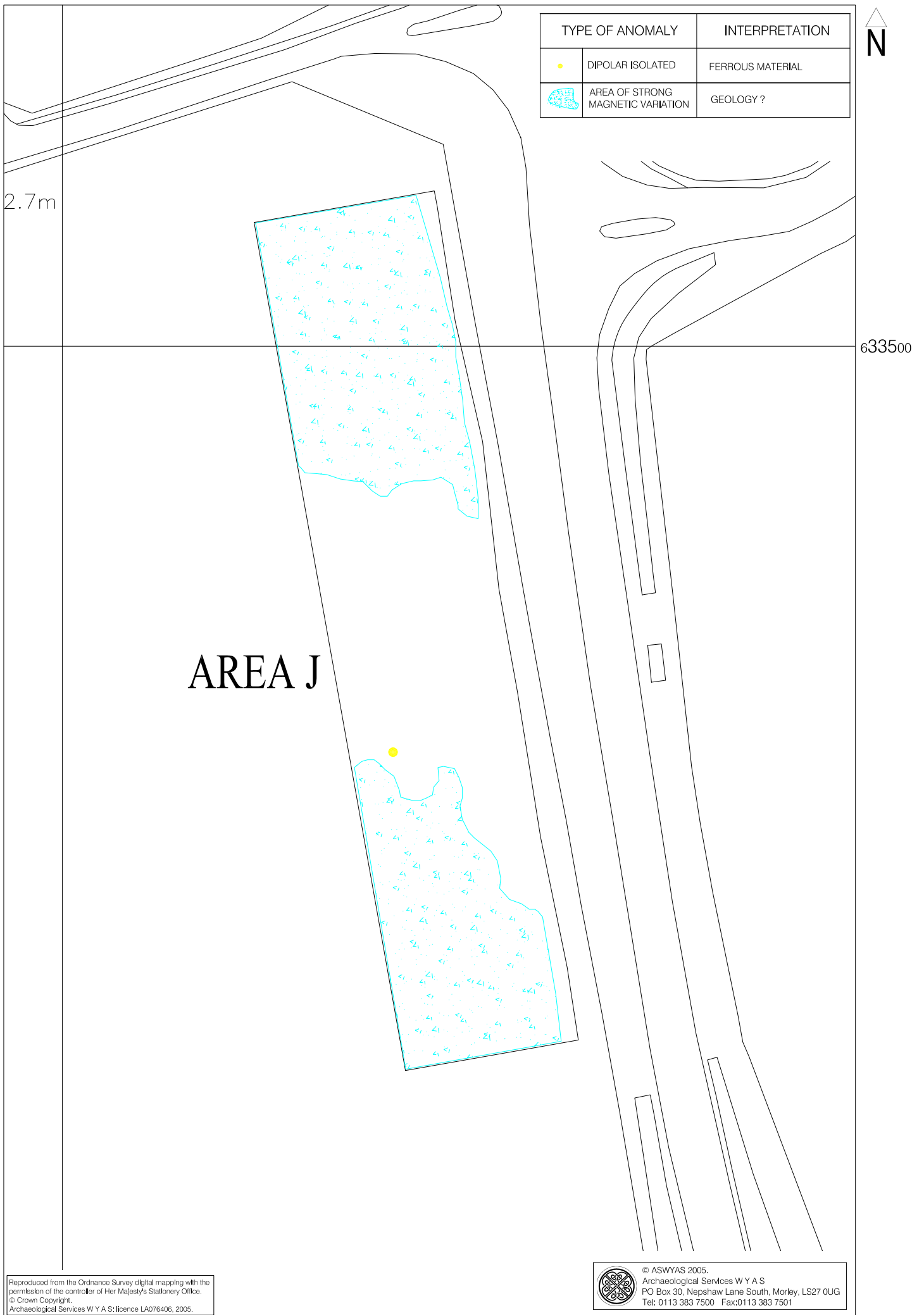
Fig. 28 Interpretation plot of magnetometer data; Area J
