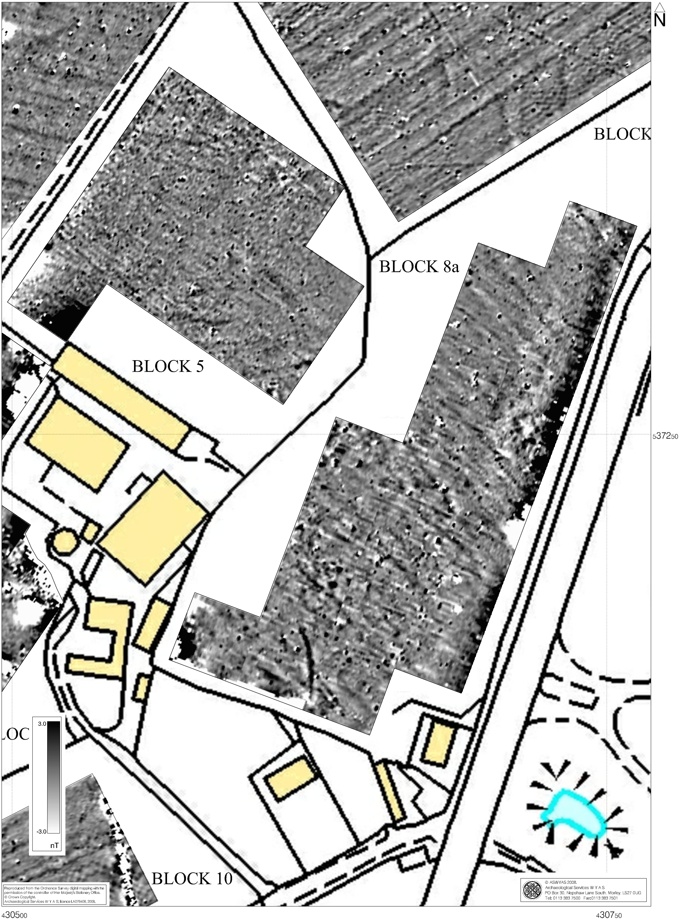
Fig. 16. Processed greyscale magnetometer data; Block 5 and 8a (1:1000 @ A3)
