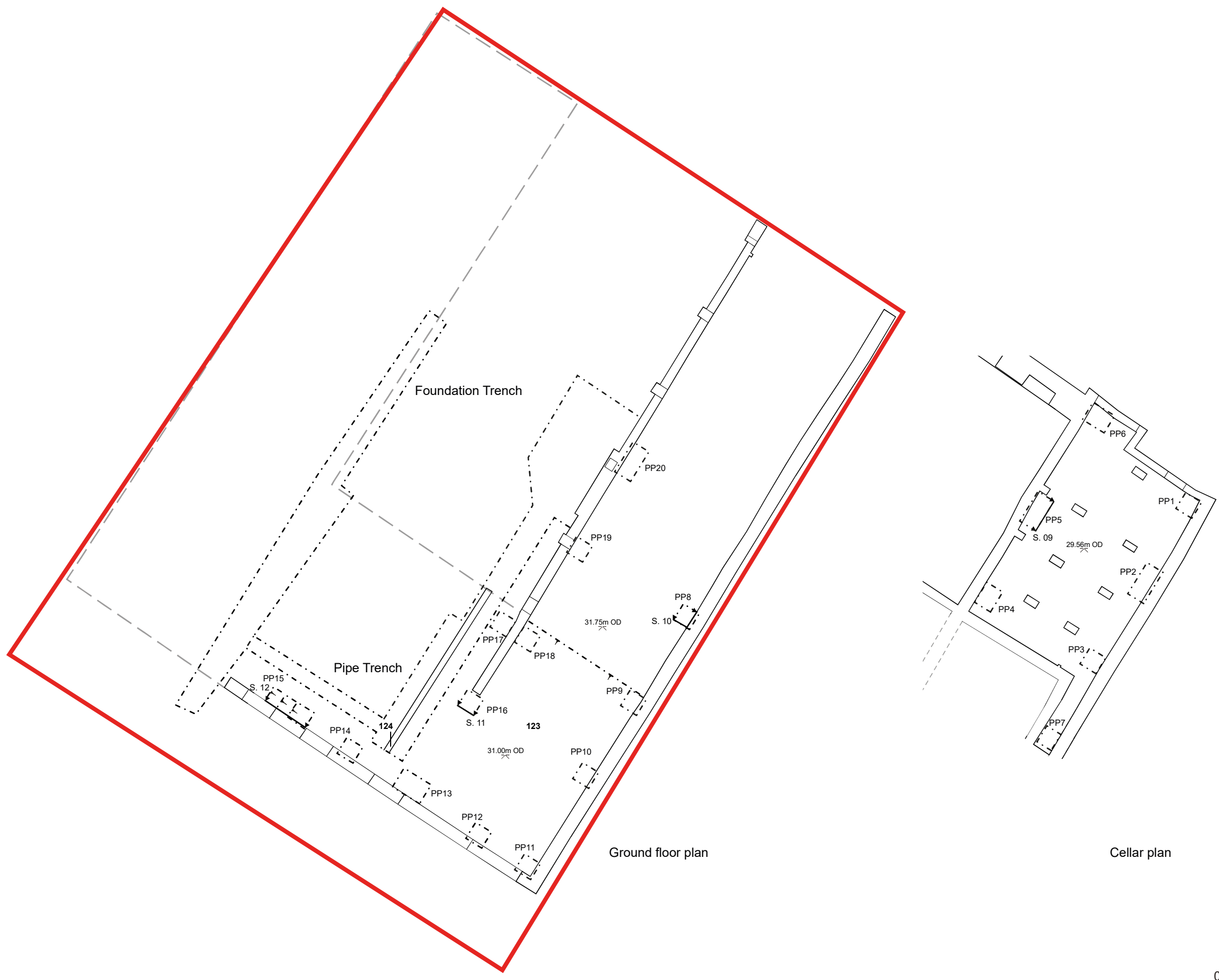
Fig. 7. Plan showing the location of the Pile Pad pits, Foundation Trench and Pipe Trench (scale 1:150 @ A3)
