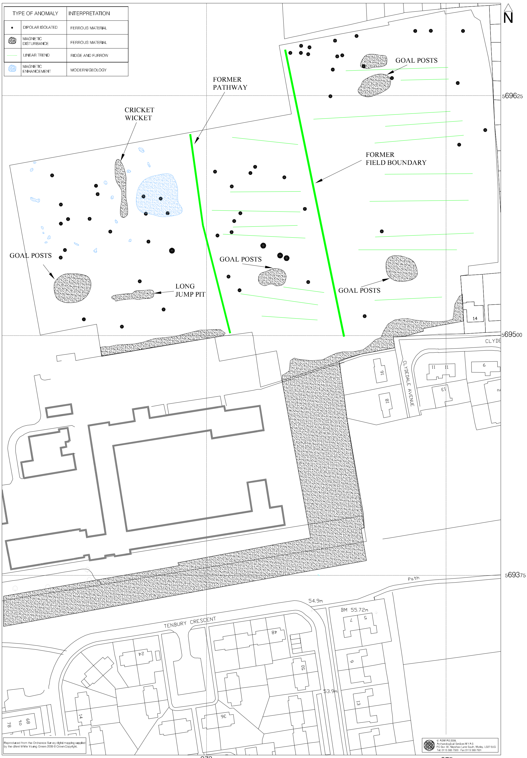
Fig. 5. Interpretation of magnetometer data (1:1000 @ A3)
