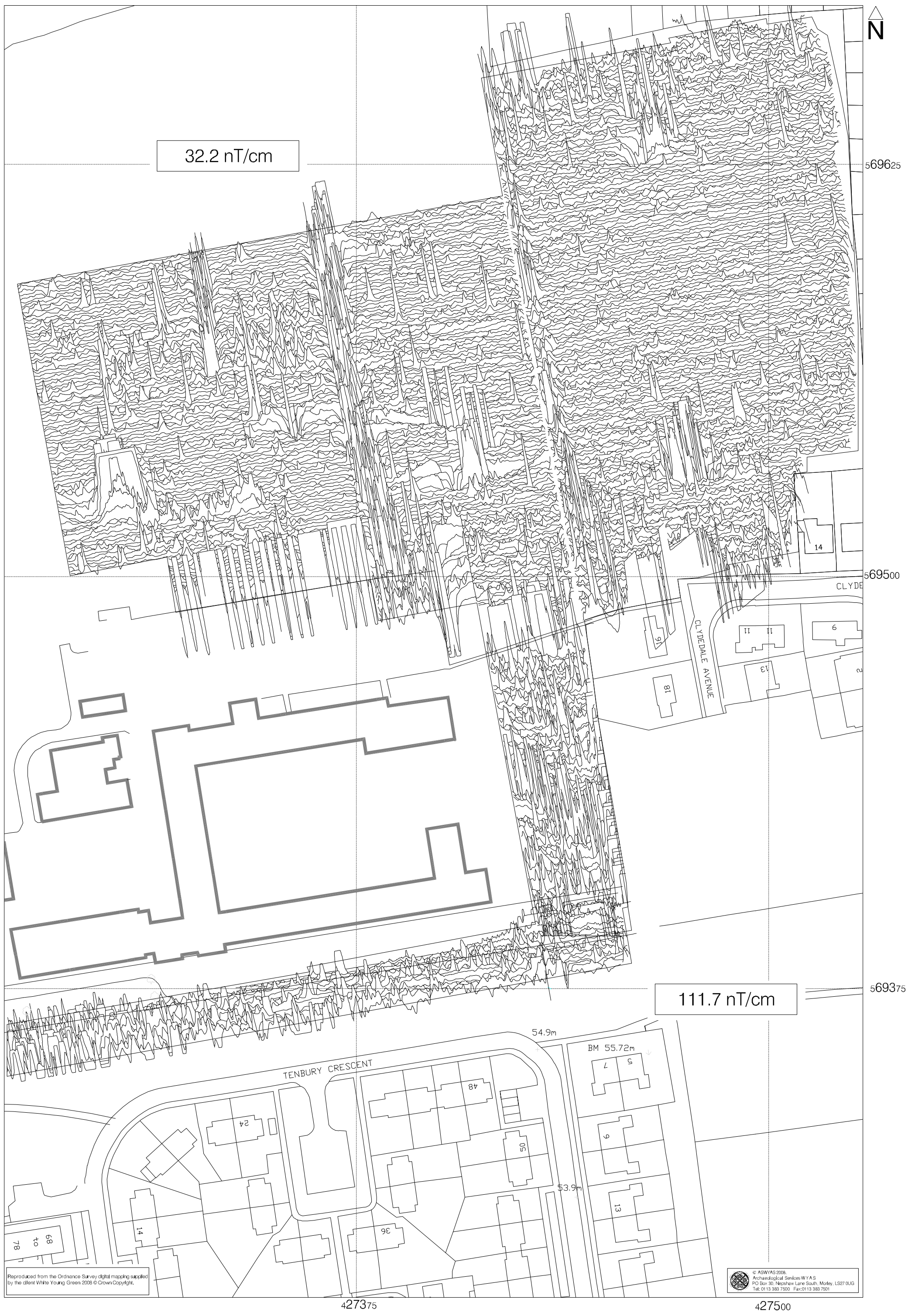
Fig. 4. XY trace plot of unprocessed magnetometer data (1:1000 @ A3)
